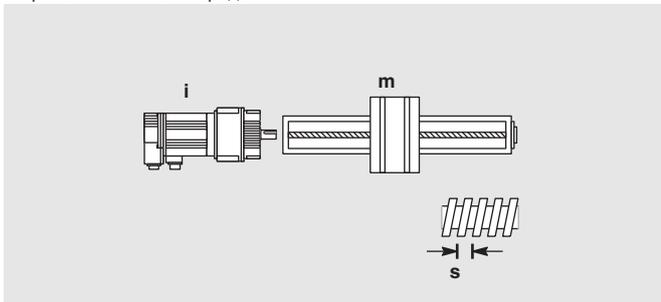
$$J_{total} = J_{motor} + \frac{\left(\frac{s}{2\pi}\right)^2 \cdot m + \frac{1}{2} \cdot m_{screw} \cdot r_{screw}^2}{i^2}$$
