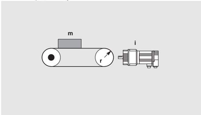
$$J_{total} = J_{motor} + \frac{2 \cdot J_{pulley} + J_{load}}{i^2}$$
