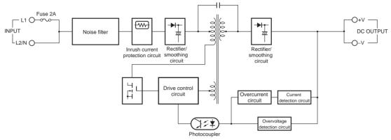
Note: The Power Supply is provided with reinforced insulation between the input and output terminals.
