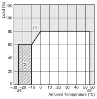
**Note: 1.** The maximum ambient temperature for parallel operation is 45°C.
