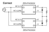
Note: When the load is an operational amplifier or other device allowing series operation, a startup failure may occur when the Power Supply is turned ON and internal circuits may be damaged. Connect a diode as shown in the figure to prevent this.
