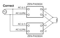
**Note: 1.** For parallel operation, a maximum of two Power Supplies of the same model can be connected.
