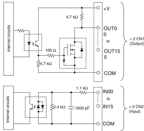
Terminal Connections: CS1W-MD561 TTL 32-point Input/32-point Output Unit
