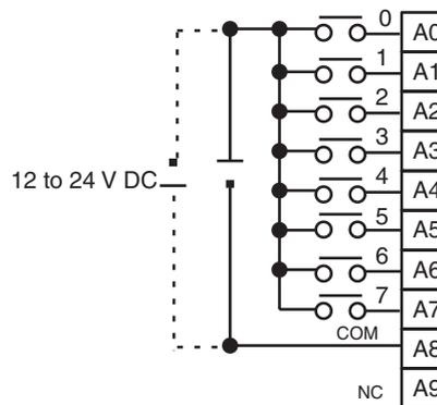
**Note** Terminal numbers A0 to A9 and B0 to B9 are used in this manual, but they are not printed on the Unit.
