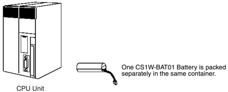
**Note** The Battery Set is required to backup the user program in the RAM memory, the contents of the PLC Setup, the I/O memory holding areas, etc., when the power supply is turned OFF.
