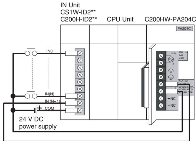
Connect the negative terminal of the 24-V DC power supply to the Input Unit common (COM) terminal.
