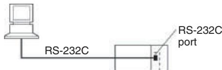
**Note** The maximum cable length for an RS-232C connection is 15 m. RS-232C communications specifications, however, do not cover transmissions at 19.2 Kbps. Refer to documentation of the device being connected when using this baud rate.
