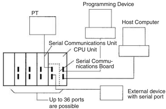
**Standard Serial Communications with External Devices**
