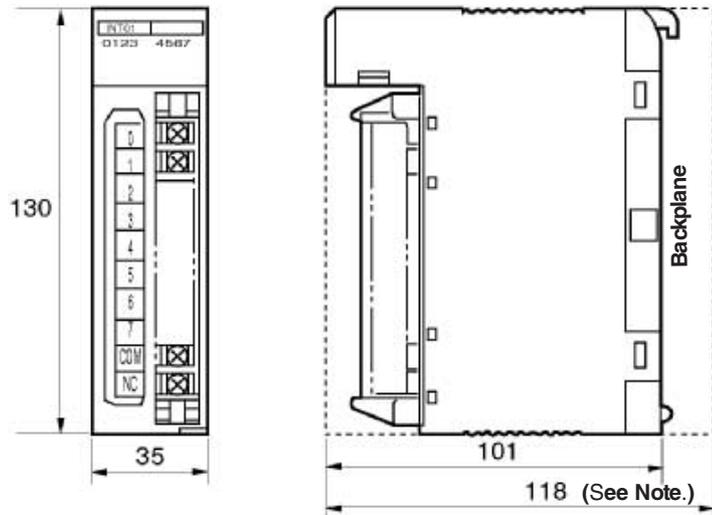
**Note** The height of the Unit including the Backplane is 5 mm greater on the CPU Backplane and CS-series Expansion Backplane (123 mm).
