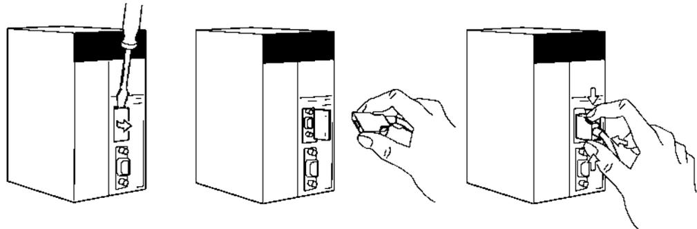
Insert a small flat-blade screwdriver into the opening at the top of the port cover and pull open.
