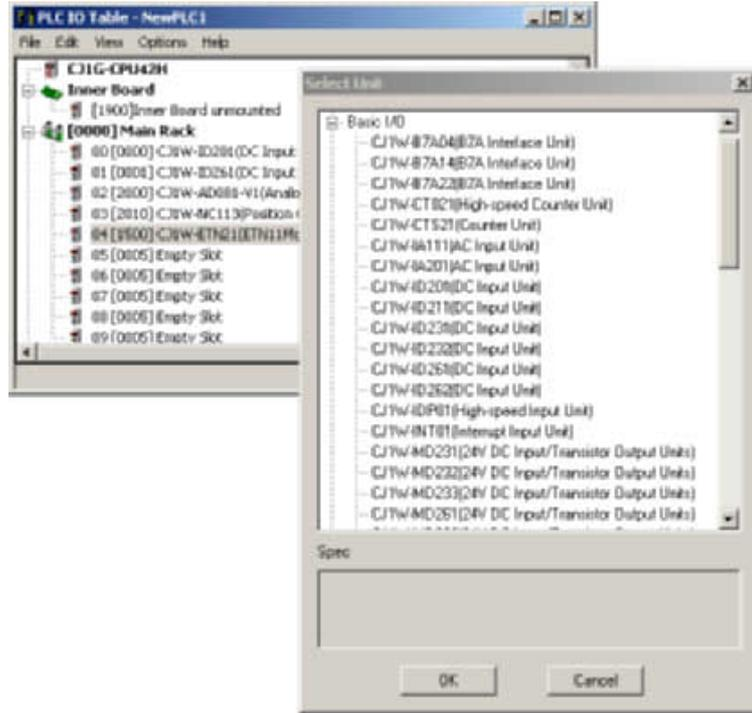
**Note** The first word allocated to each Rack can be set by selecting **Rack/Slot Start Addresses** from the Option Menu of the PLC IO Table Window of the CX-Programmer.
