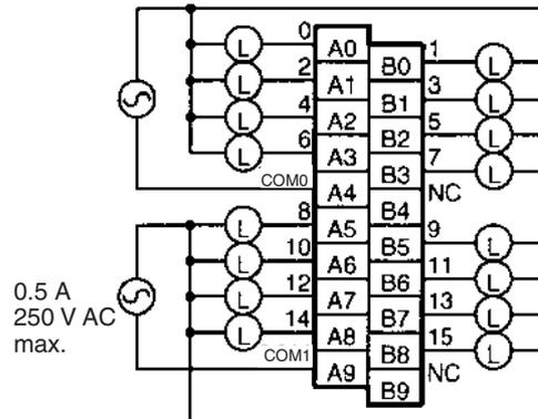
**Note** Terminal numbers A0 to A9 and B0 to B9 are used in this manual, but they are not printed on the Unit.
