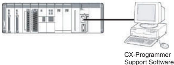
2. When connecting to the RS-232C port, pin 5 of the CPU Unit's DIP switch must be ON. After checking the power supply wiring and voltage, turn ON the power and verify the Power Supply Unit's POWER Indicator is lit.
