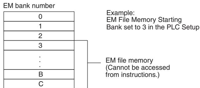
**Note** When designating addresses in programming or allocations inside C200H Special I/O Units, “EM 0000” to “EM 6143” will actually specify E0\_00000 to E0\_06143 in the CPU Unit. Other addresses in this area cannot be specified.
