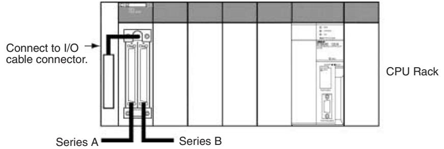
**Note** Connect a Terminator (CV500-TER01) to the unused connector when connecting only series A or series B.
