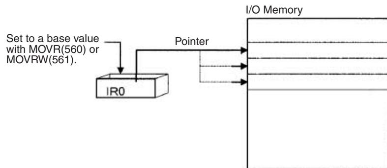
**Note** It is possible to specify regions outside of I/O memory and generate an Illegal Access Error when indirectly addressing memory with Index Registers. Refer to *Appendix C Memory Map* for details on the limits of PLC memory addresses.
