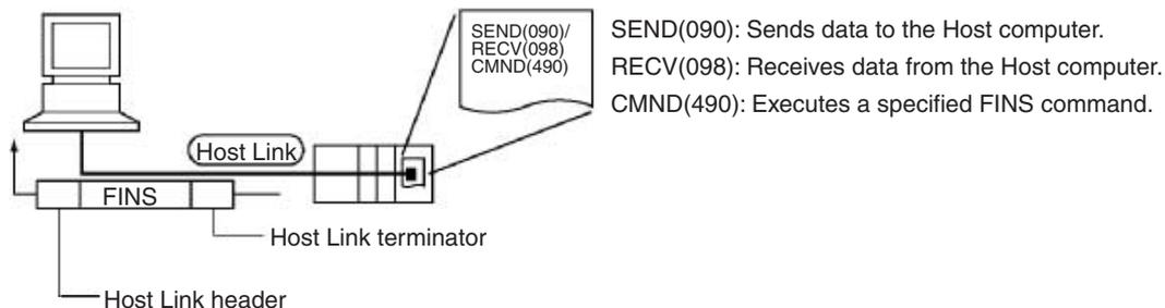
In Host Link mode, FINS commands contained between a header and terminator can be sent from the host computer to any PLC on the Network. Communications are possible with PLCs on the same or different types of interconnected Networks up to two levels away (three levels including the local level but not including the Host Link connection).
