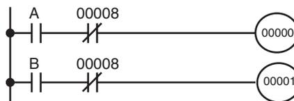
Since alarm output bit 08 covers both output bits 00 and 01, both these outputs are forced OFF as soon as output bit 08 turns ON (bits A and B can be any other bits required in the program).
