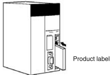
3. Push the Memory Card securely into the compartment. If the Memory Card is inserted correctly, the Memory Card eject button will be pushed out.
