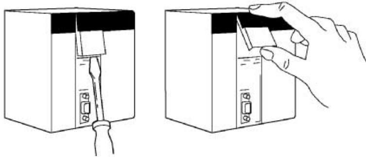
Insert a small flat-blade screwdriver into the opening at the bottom of the battery compartment cover and lift open the cover.
