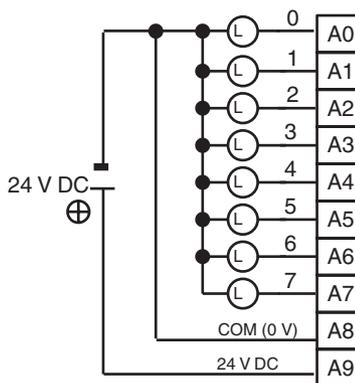
**Note** Be sure to supply power to A9; otherwise current will leak through the load while the output is OFF.
