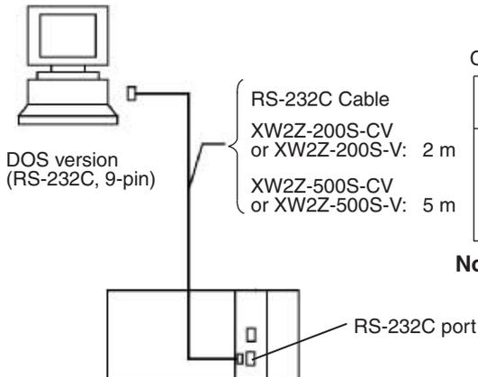
Connecting Cables for RS-232C Port
