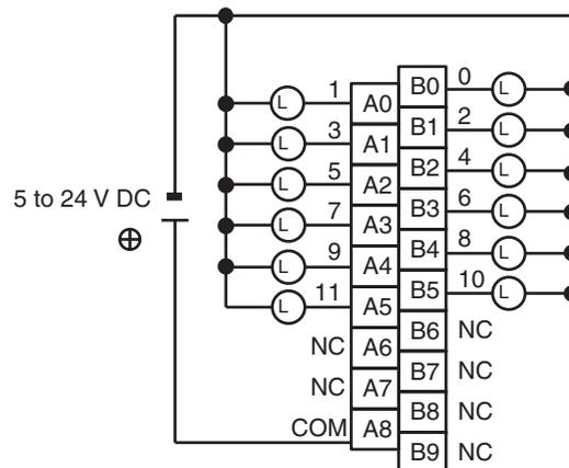
**CS1W-OD212 Transistor Output Unit (16 Points, Sourcing)**
