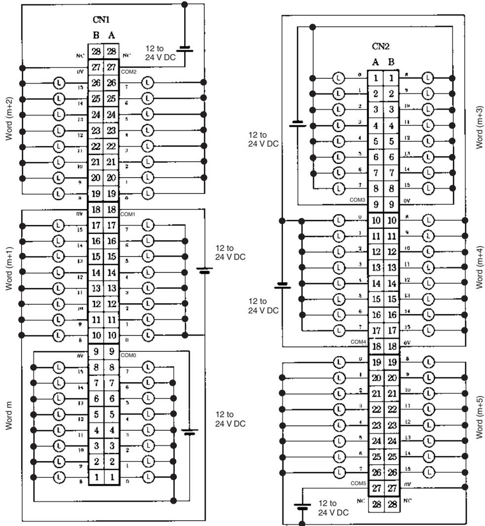
**CS1W-MD261 DC Input/Transistor Output Unit (32/32 Points, Sinking)**
