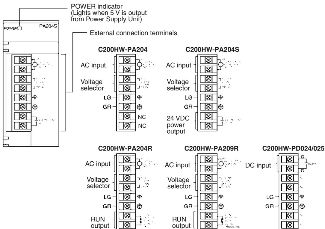
**Note** 100 to 120 V AC: Closed circuit, 200 to 240 V AC: Open circuit
