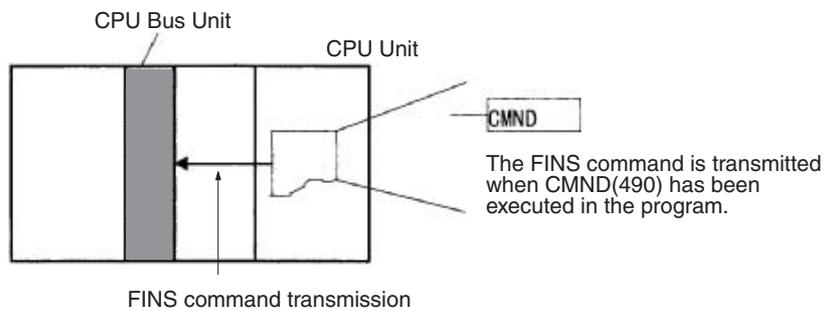
FINS commands can be transmitted to CPU Bus Units in other PLCs in the network, not just the local PLC.
