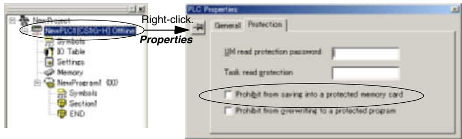
2. Either select **PLC - Transfer - To PLC** to transfer the program or select **PLC - Protection - Set Password** and click the **OK** button.
