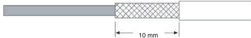
4. Use wire strippers to remove the insulation from the end of each wire.
