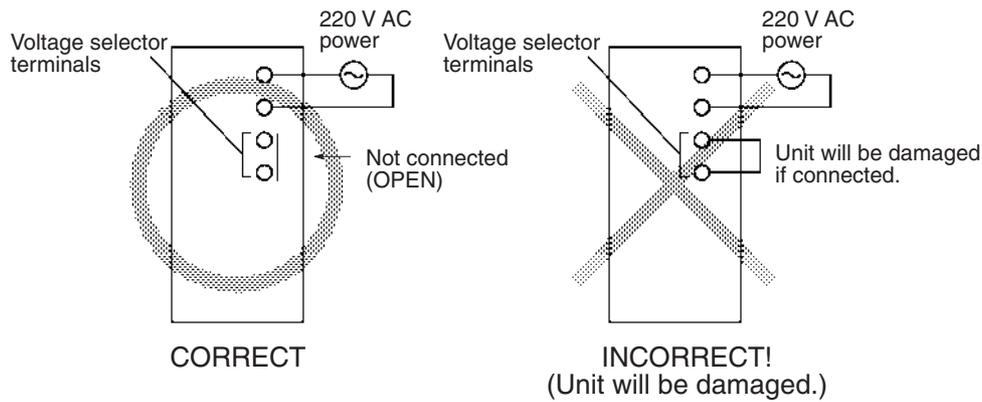
**Note** If 110 V AC power is supplied but the jumper bar has been removed to select 220 V AC, the Unit will not operate because the power supply voltage will be below the 85% minimum level.
