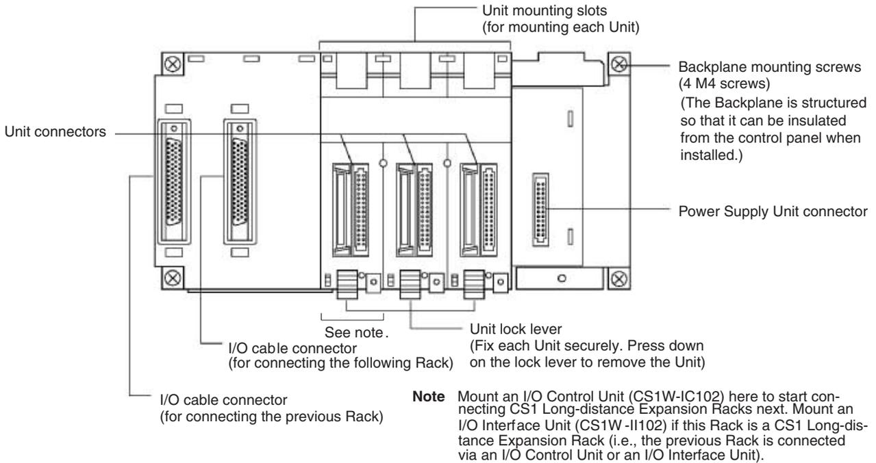
**Note** Always cover the connectors that are not being used with Connector Covers (sold separately) as a measure against dust.
