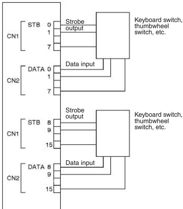
Using strobe signals STB 0 to 7 as outputs, data signals DATA 0 to 7 as inputs, strobe signals STB 8 to 15 as outputs, and data signals DATA 8 to 15 as inputs, 128 bits (8 words) can be input from strobe input keyboard switches or thumbwheel switches as shown in the following diagram.
