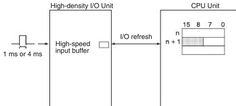
The High-density I/O Unit data in the high-speed input buffer can also be refreshed during program execution by executing the IORF(097) instruction for the desired Special I/O Unit.
