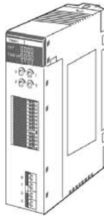
The Analog Timer Unit is classified as a Basic I/O Unit and is allocated one word in the I/O Area. The word (16 bits) allocated to the Unit is used for the 4 timers' start input, pause input, time-up output, and data transfer with the CPU Unit.
