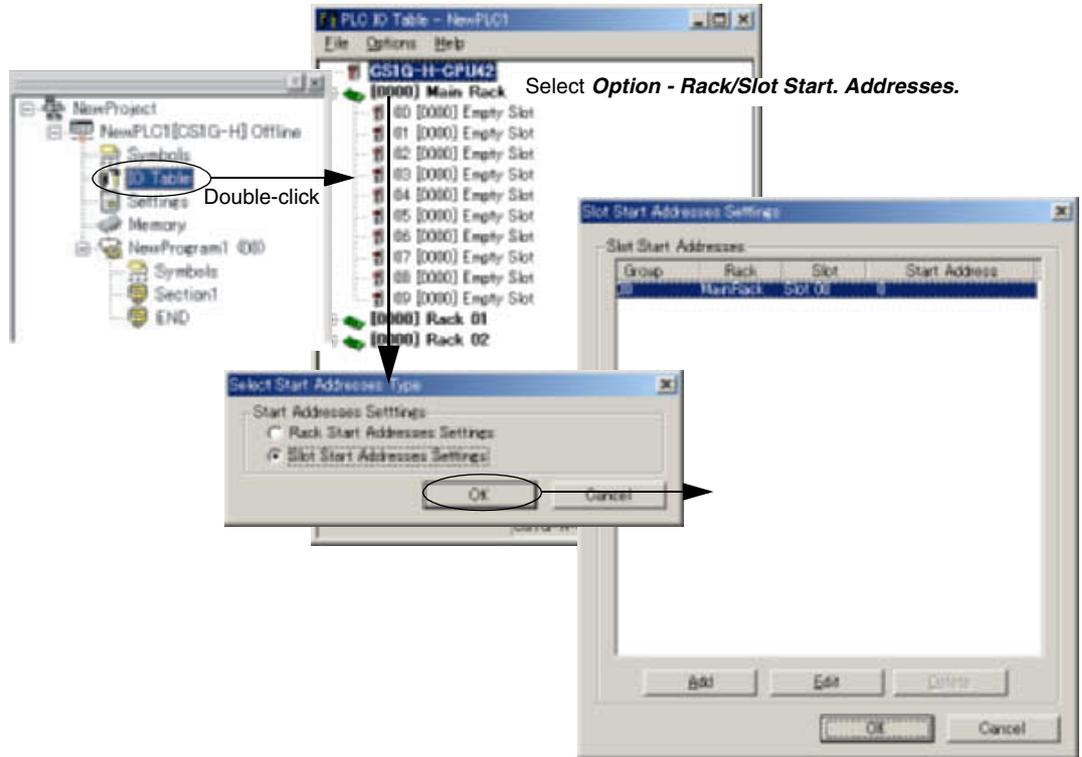
This function can be used, for example to allocate fixed addresses to Input Units and Output Units. (With CQM1H PLCs, input bits are from IR 000 to IR 115 and output bits are from IR 100 to IR 115. First slot addresses can be set when replacing CQM1H PLCs with CS/CJ-series PLCs to reduce conversion work.)
