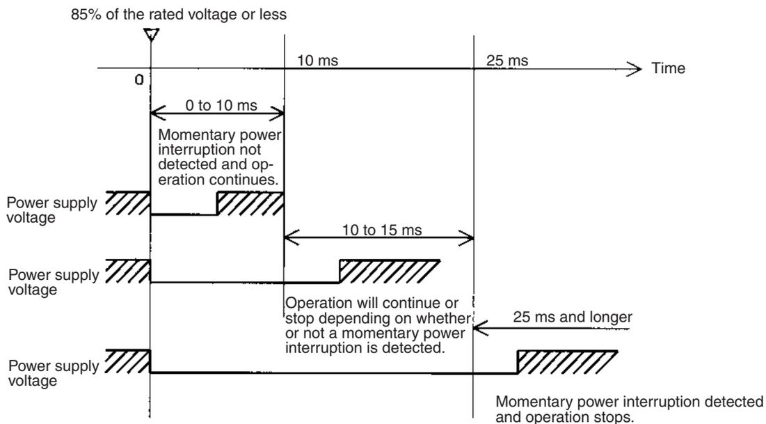
**Note** The above timing chart shows an example when the power OFF detection time is set to 0 ms (the default value).
