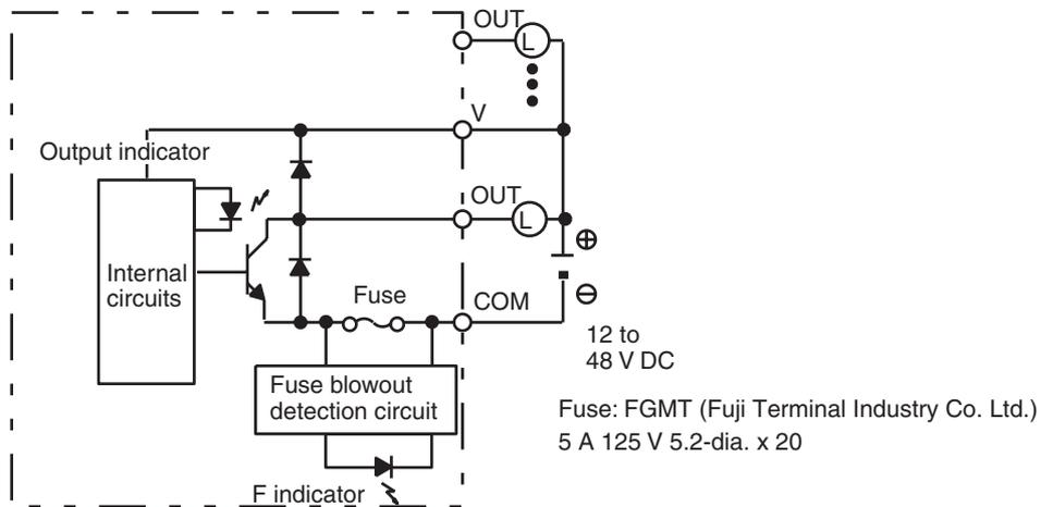
**Note** When the fuse blows, the F indicator lights and bit 08 turns ON. Bits 08 through 15 cannot be used as work bits.
