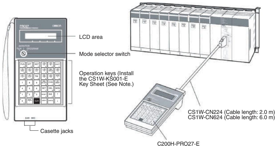
Connect the CPU Unit to the Programming Console with the following cables.
