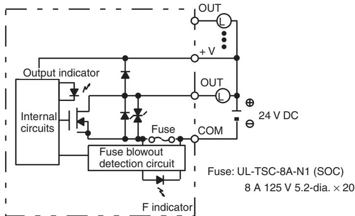
**Note** When the fuse blows, the F indicator lights and bit 08 turns ON. Bits 08 through 15 cannot be used as work bits.
