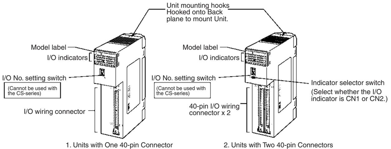
**Note** The I/O number setting switch on the front panel of C200H Group-2 High-density I/O Units is not used for the CS Series, i.e., the I/O number setting will not affect allocations. Words are allocated to the Units according to their position on the Rack in the same way as for Basic I/O Units.
