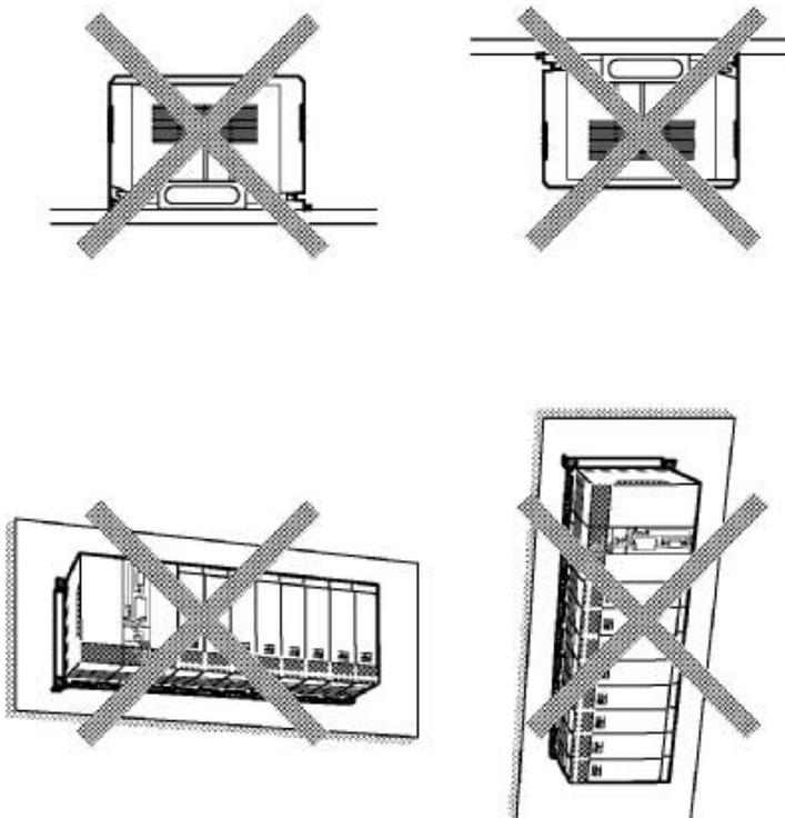
**Note** Always use the standard installation method. A nonstandard installation will decrease heat dissipation, and may delay the replacement notification signal (in particular for C200H-PA204C Power Supply Units with Replacement Notification), or degrade or damage the internal elements.
