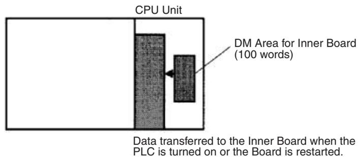
Data transferred to the Inner Board when the PLC is turned on or the Board is restarted.
