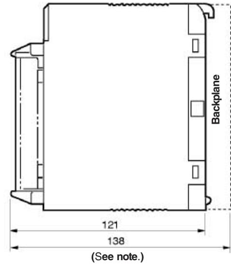
**Note** The heights of the Units including the Backplane are 5 mm greater on the CPU Backplane and CS-series Expansion Backplane (123 and 143 mm).
