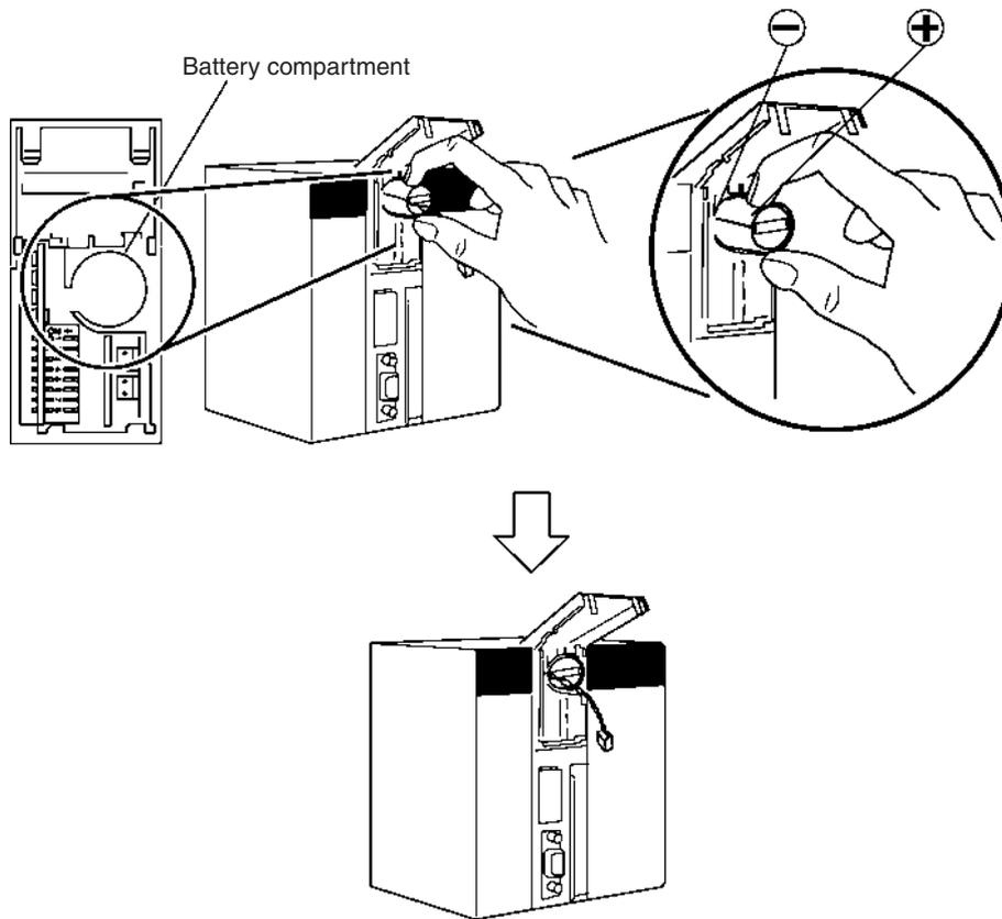
3. Connect the battery connector to the battery connector terminals. Connect the red wire to the top and the black wire to the bottom terminal. There are two sets of battery connector terminals; connect the battery to either one. It does not matter whether the top terminals or bottom terminals are used.
