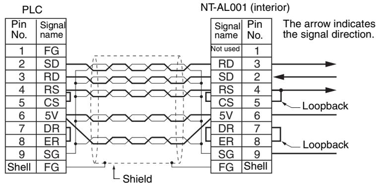
2. When the NT-AL001-E Link Adapter is connected to the RS-232C port on the CPU Unit, 5 V is supplied from pin 6, eliminating the need for a 5-V power supply.
