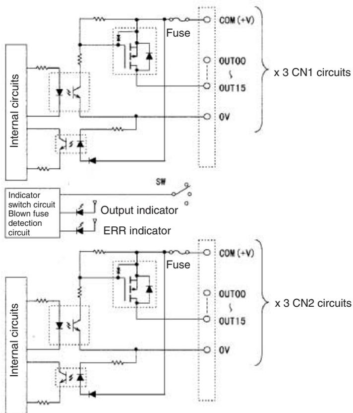
**Note** The ERR indicator will light if a fuse blows or if the external power supply is turned OFF, and the corresponding Flag in the Basic I/O Unit Information Area (A050 to A089) will turn ON.
