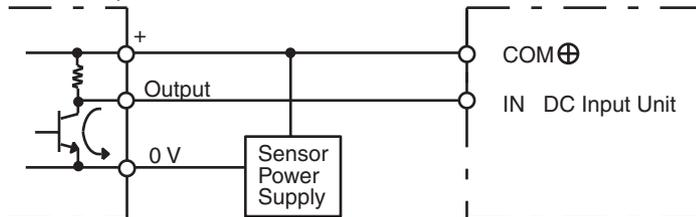
The circuit below should **NOT** be used for I/O devices having a voltage output.
