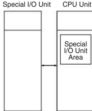
These settings determine whether or not data will be exchanged with the 10 words allocated to each Special I/O Unit in the Special I/O Unit Area during cyclic I/O refreshing.
