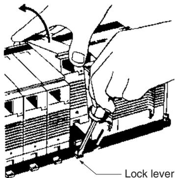
4. Use a Phillips-head screwdriver to remove the screws from the top and bottom of the Unit.
