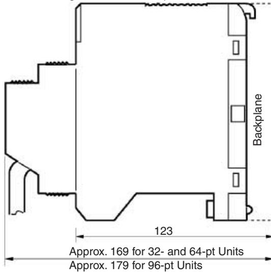
Using Pressure-welded Connector
