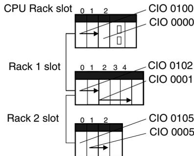
**Note** The first address settings for Racks and slots can be uploaded/downloaded from/to the CPU Unit.
