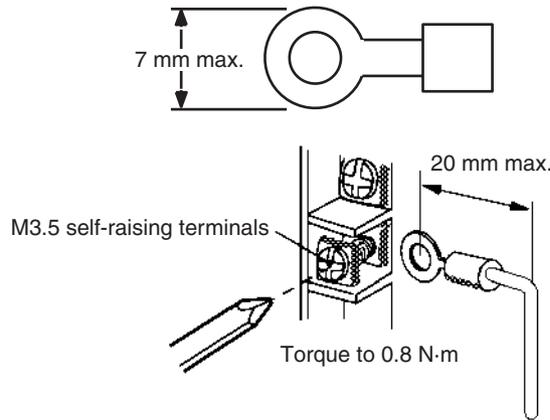
**Caution** ⚠ Tighten the AC power supply terminal block screws to the torque of 0.8 N·m. Loose screws may result in short-circuit, malfunction, or fire.
