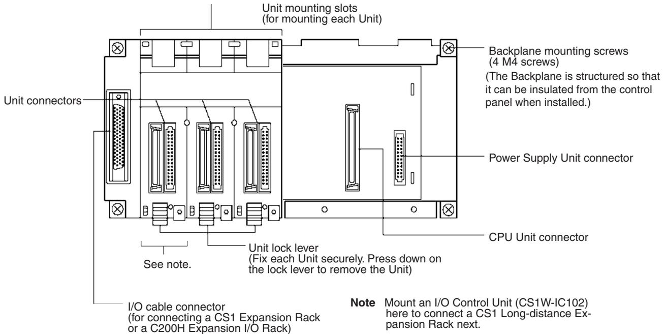
**Note** Always cover the connectors that are not being used with Connector Covers (sold separately) as a measure against dust.
