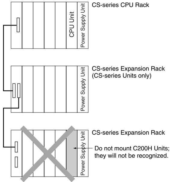
4. When using a CS-series-only CPU Expansion Rack (CS1W-BI□□2) with a CPU Unit with a lot number of 000427 (27 April 2000) or earlier, C200H Units cannot be used on any Expansion Racks past the CS-series-only CPU Expansion Rack. If they are used past the CS-series-only CPU Expansion Rack, the C200H Units will not be recognized by the CPU Unit.
