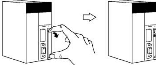
2. Insert the Memory Card with the label facing to the right. (Insert with the Δ on the Memory Card label and the ◁ on the CPU Unit facing each other.)
