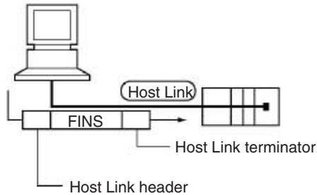
In Host Link mode, FINS commands contained between a header and terminator can be sent from the host computer to any PLC on the Network. Communications are possible with PLCs on the same or different types of interconnected Networks up to two levels away (three levels including the local level but not including the Host Link connection).
