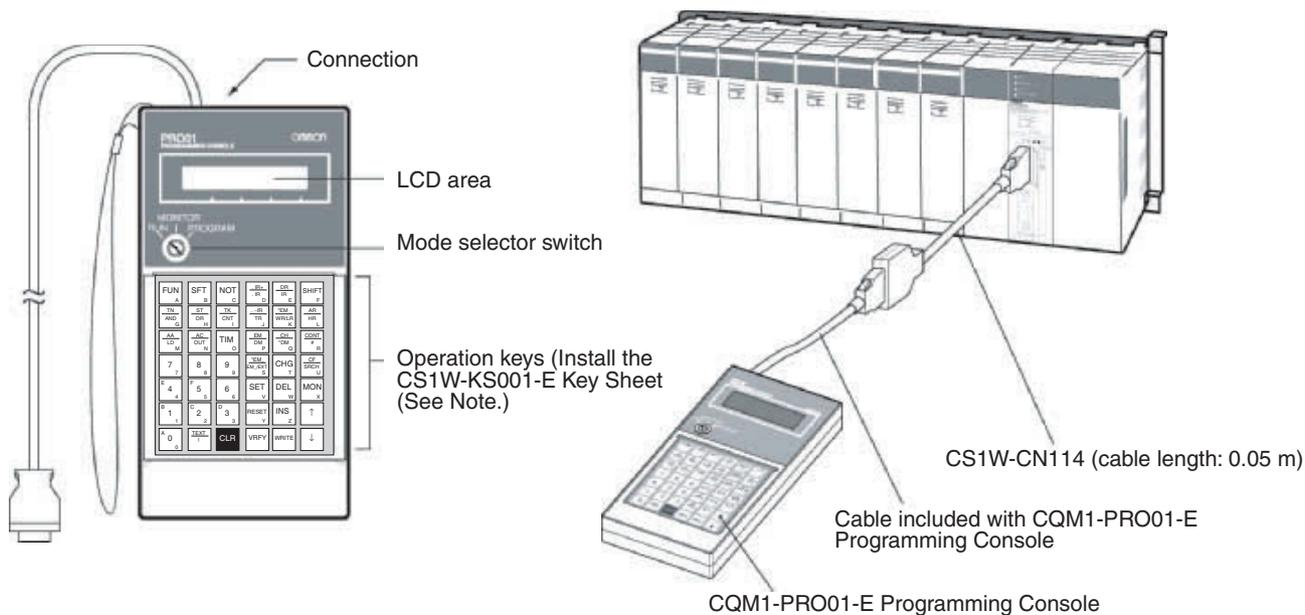
Connect the CPU Unit to the Programming Console with the following cables.
