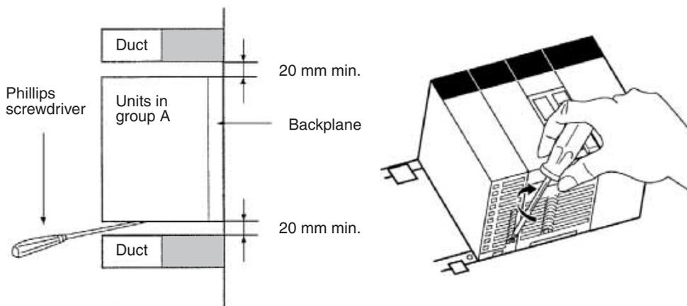
With Group-B Units, the lock lever will snap into place when the Unit is properly inserted. Check that the lock lever is engaged and the Unit is secure.
