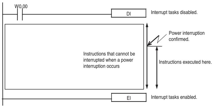
2. Set the Disable Setting for Power OFF Interrupts in A530 to A5A5 hex to enable disabling power interruption processing.
