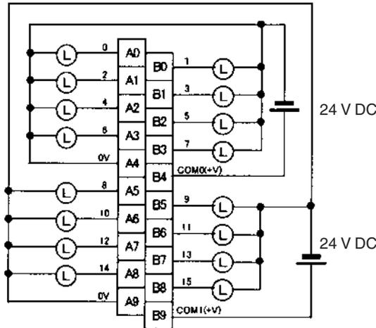
**Note** Terminal numbers A0 to A9 and B0 to B9 are used in this manual, but they are not printed on the Unit.
