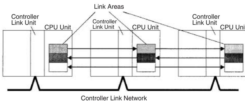
Link Area words are also allocated to PLC Link Systems when a PLC Link is created by connecting PLC Link Units.
