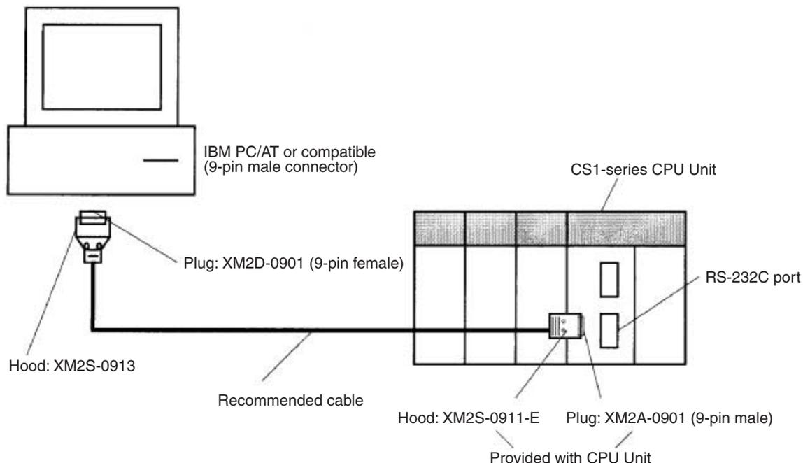
**Note** Use the special cables provided from OMRON for all connections whenever possible. If cables are produced in-house, be sure they are wired correctly. External devices and the CPU Unit may be damaged if general purpose (e.g., computer to modem) cables are used or if wiring is not correct.
