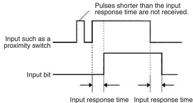
The default setting for the input response time is 8 ms and the setting range is 0 to 32 ms. When the input response time is set to 0 ms, the only delay will be the delays in the Unit's internal elements. For information on the Unit's internal elements, refer to *Appendix A Specifications of Basic I/O Units and High-density I/O Units* and check the input response time for the Unit that you are using.
