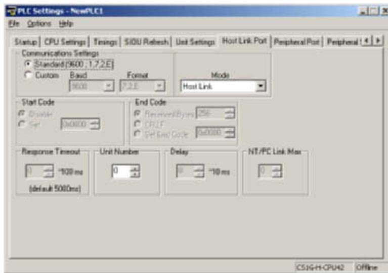
The following settings are valid when pin 4 on the DIP switch on the CPU Unit is ON.
