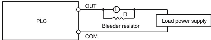
Use the following formula to determine the resistance and rating for the bleeder resistor.
