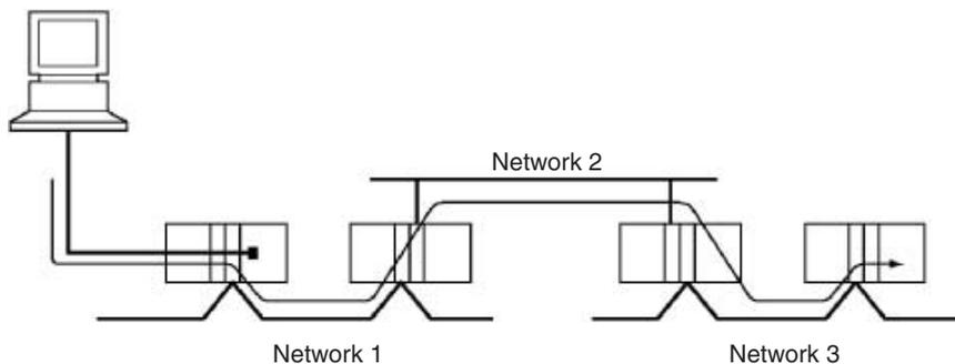
**Note** With CS/CJ-series CPU Units Ver. 2.0 or later, remote programming/monitoring is possible up to 8 levels away. Refer to *1-6-5 Communications through a Maximum of 8 Network Levels* for details.
