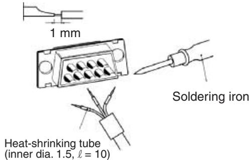
4. Move the heat-shrinking tubes onto the soldered area and shrink them into place.
