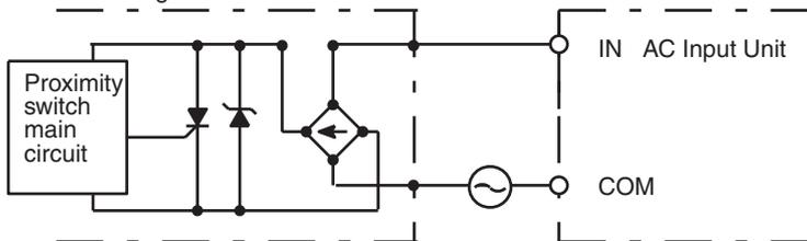
**Note** When using a reed switch as the input contact for an AC Input Unit, use a switch with an allowable current of 1 A or greater. If Reed switches with smaller allowable currents are used, the contacts may fuse due to surge currents.
