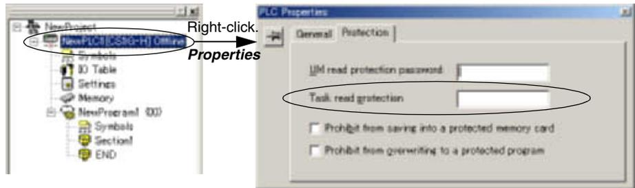
2. Select the tasks that will be password-protected and select the *Task read protect* Option in the *Program Properties* Tab.
