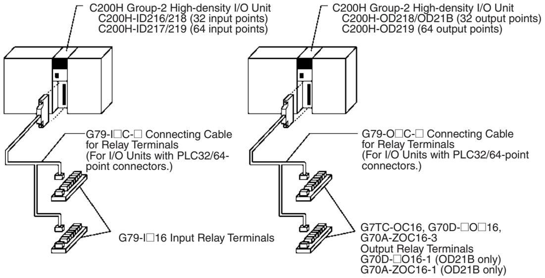
**CS-series Basic I/O Units with Connectors**
