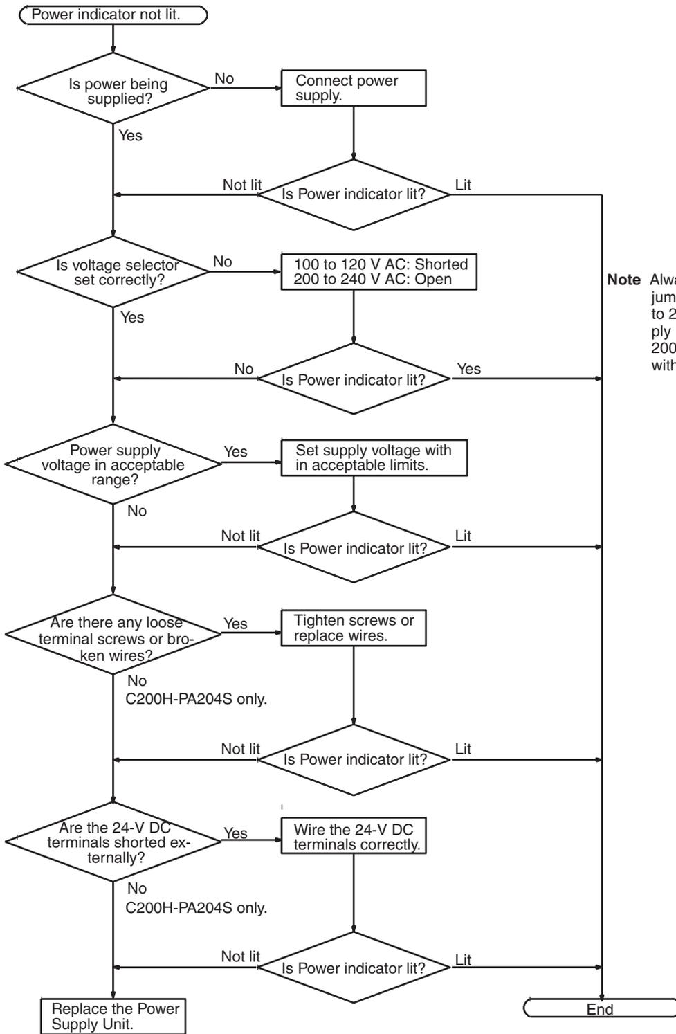
**Note** Always remove the short jumper before supplying 200 to 240 V AC. The Power Supply Unit will be destroyed if 200 to 240 V AC is supply with the jumper connected.
