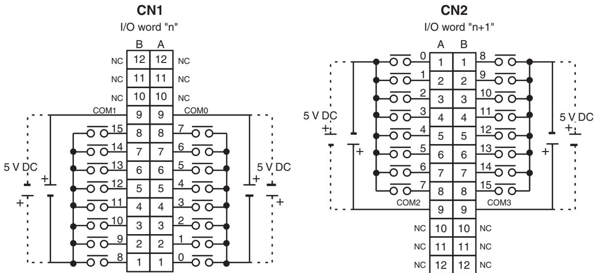
**Note** When pin 2 of the Unit's DIP switch is ON, input points 08 to 15 in connector 2 are high-speed inputs.
