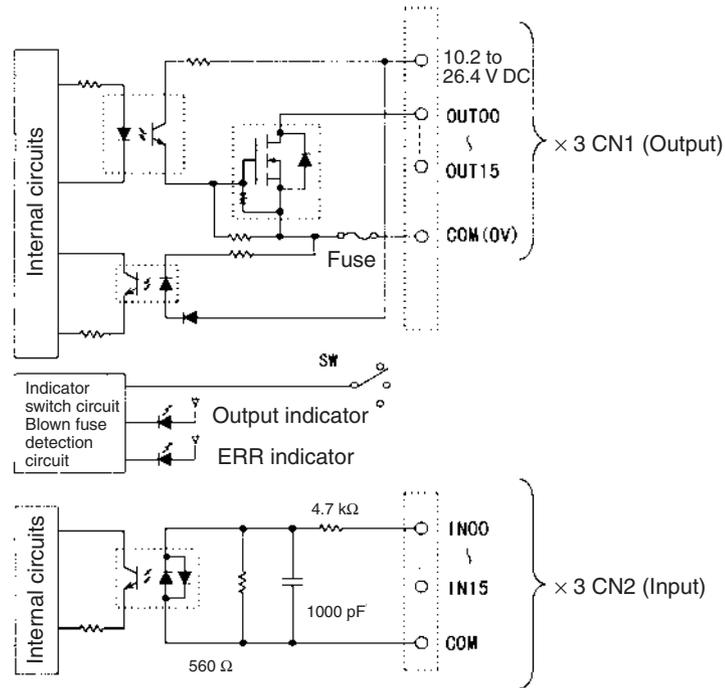
**Note** The ERR indicator will light if a fuse blows or if the external power supply is turned OFF, and the corresponding Flag in the Basic I/O Unit Information Area (A050 to A089) will turn ON.
