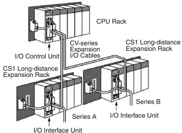
**Mounting the I/O Control Unit to a CS-series Expansion Rack**
