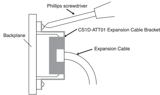
Tighten the screws to a torque of 0.5 N·m.
