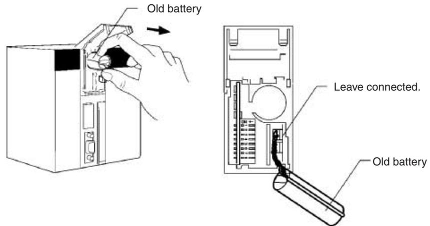
4. Insert the new battery into the battery compartment with the cable and connector facing outward.
