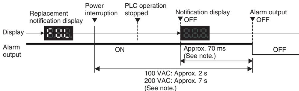
If replacement is already required, the display will turn OFF after the PC operation stops. When the display turns OFF, the alarm output will turn ON momentarily and then turn OFF again.
