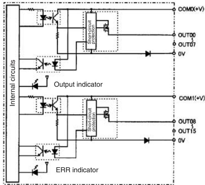
When overcurrent is detected, the ERR indicator will light, and the corresponding flag in the Basic I/O Unit Information Area (A050 to A089) will turn ON.
