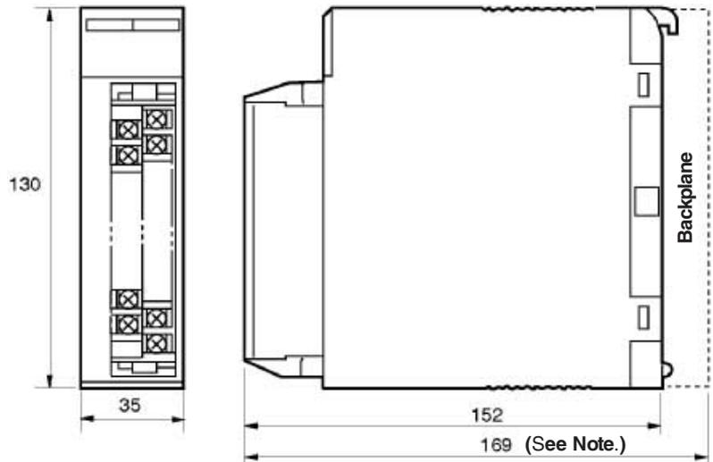
**Note** The heights of the Units including the Backplane are 5 mm greater on the CPU Backplane and CS-series Expansion Backplane (150 and 174 mm).
