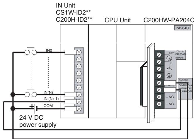
**External Display Device Connection Example**
