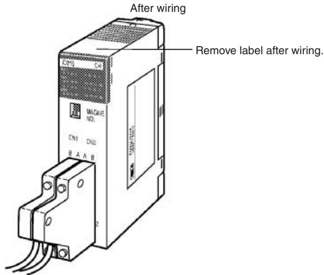
Tighten the connector-attaching screws to a torque of 0.2 N·m.
