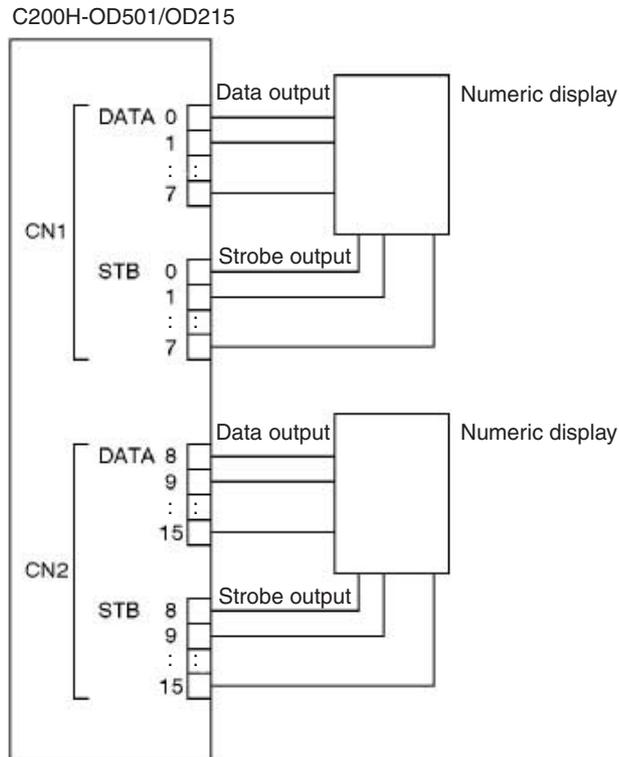
By combining data signals (DATA 0 to 7 and DATA 8 to 15) with strobe signals (STB 0 to 7/ STB 8 to 15, 128 bits (8 words) can be output to a numerical display device as shown in the following diagram.
