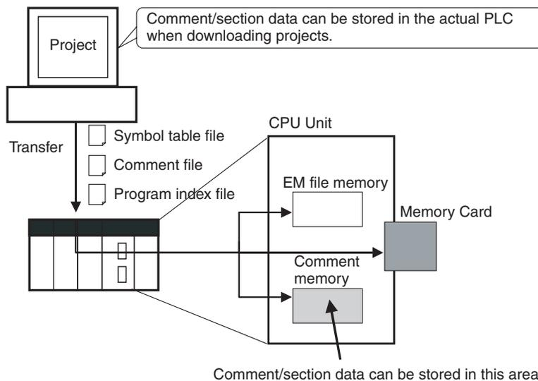
When downloading projects using the CX-Programmer Ver. 5.0, either of the following storage locations can be selected as the transfer destination for comment data and section data.
