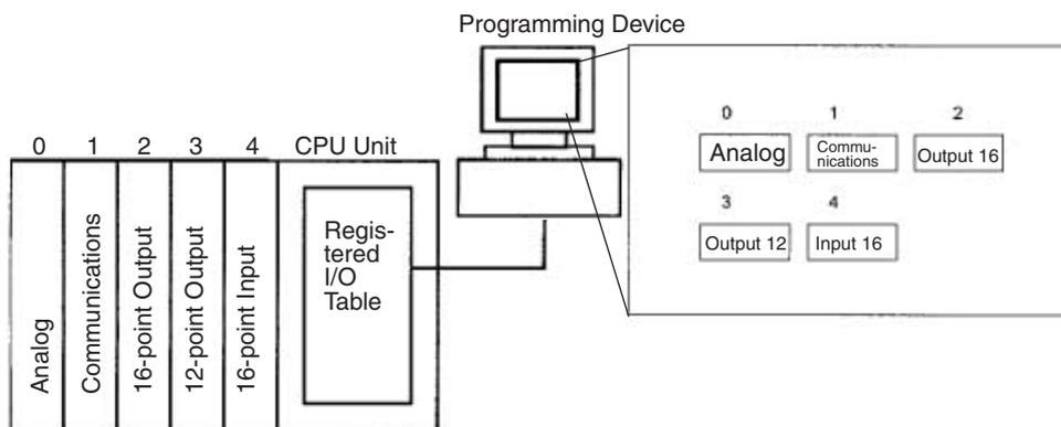
The I/O Verification Error Flag (A40209) will be turned ON if the models and locations of the Units actually mounted to the PLC (CPU Rack, Expansion I/O Racks, and Slave Racks) do not match the information in the Registered I/O Table.
