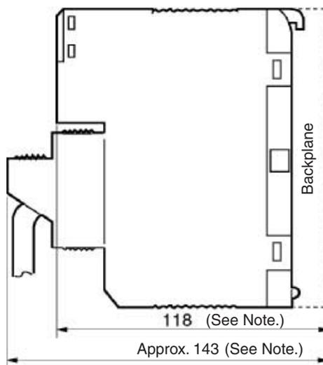
**Note** The height of the Unit including the Backplane is 5 mm greater on the CPU Backplane and CS-series Expansion Backplane (123 and 148 mm).
