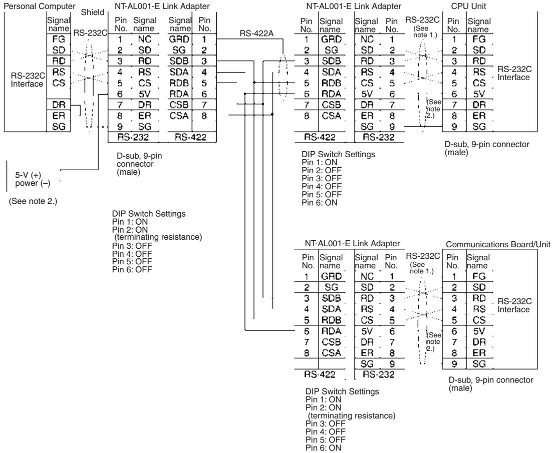
**Note 1.** We recommend using the following NT-AL001-E Link Adapter Connecting Cables to connect to NT-AL001-E Link Adapters.
