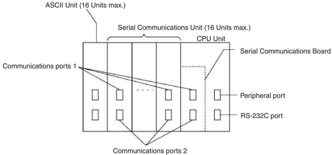
Expanding the system configuration as shown above allows a greater number of serial communications ports, and greater flexible and simpler support for different protocols.
