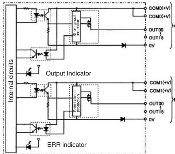
When the output current of any output exceeds the detection current, the output for that point will turn OFF. At the same time, the ERR indicator will light and the corresponding flag (one for each common) in the Basic I/O Unit Information Area (A050 to A089) will turn ON.
