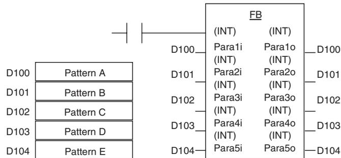
**Unit Version 4.0 or Later** Input-output variables can be used to passed large quantities of data, such as table data.
