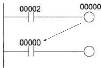
An output bit can be used in only one Output instruction that controls its status. If an output bit is used in two or more Output instructions, only the last instruction will be effective.
