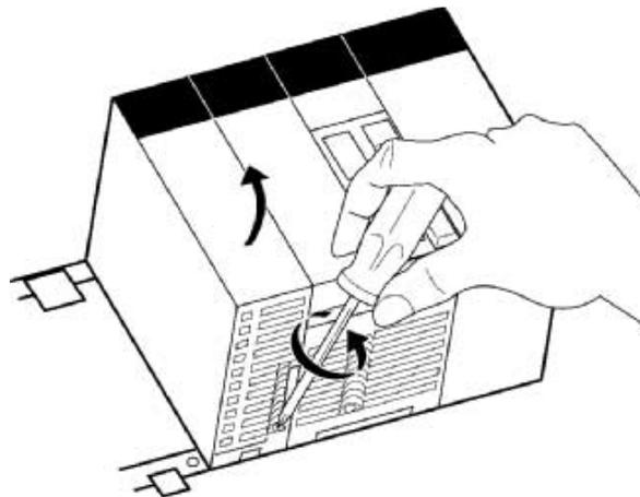
To remove a Group-B Unit, hold down the lock lever with a tool such as a screwdriver, rotate the Unit upward, and remove it.
