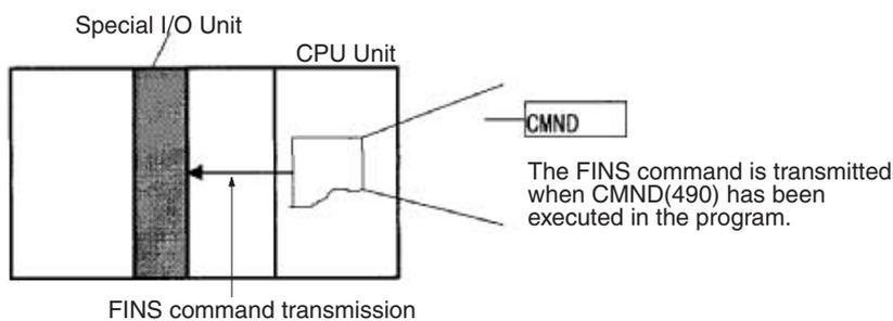
FINS commands can be transmitted to Special I/O Units in other PLCs in the network, not just the local PLC.
