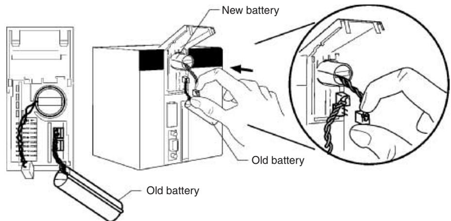
6. Remove the old battery's connector.
