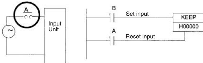
There are no restrictions in the order of using bit address or in the number of N.C. or N.O. conditions that can be programmed.
