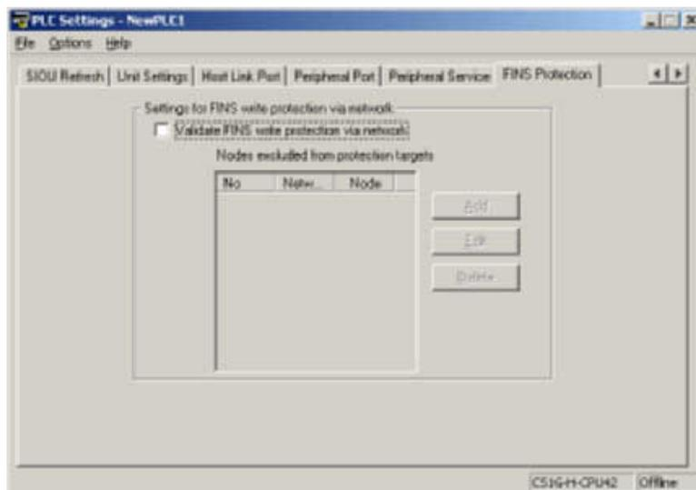
**Enabling FINS Write Protection (Use FINS Write Protection)**
