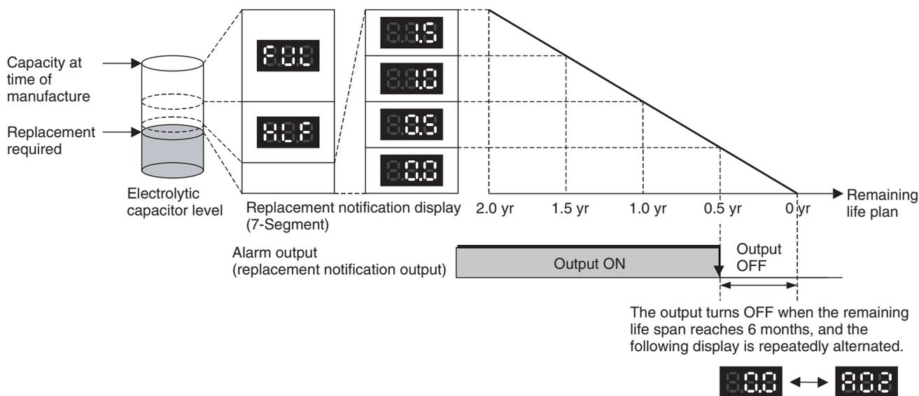
**Note** 1. The time remaining until replacement does not include periods when the power is turned OFF.
