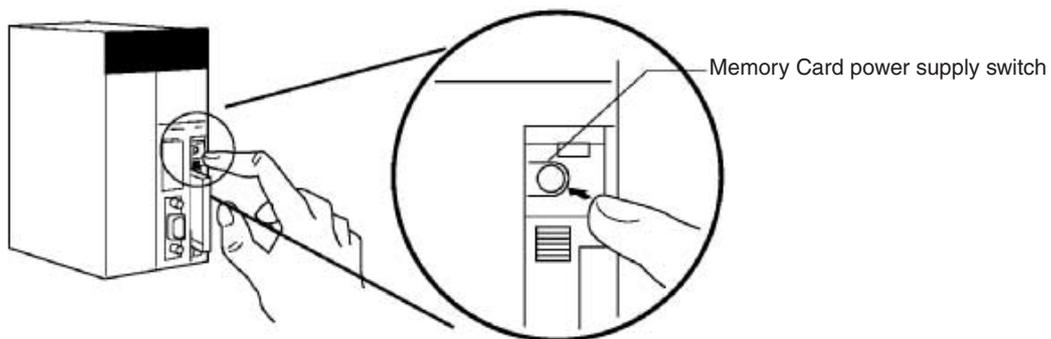
2. Press the Memory Card eject button after the BUSY indicator is no longer lit.
