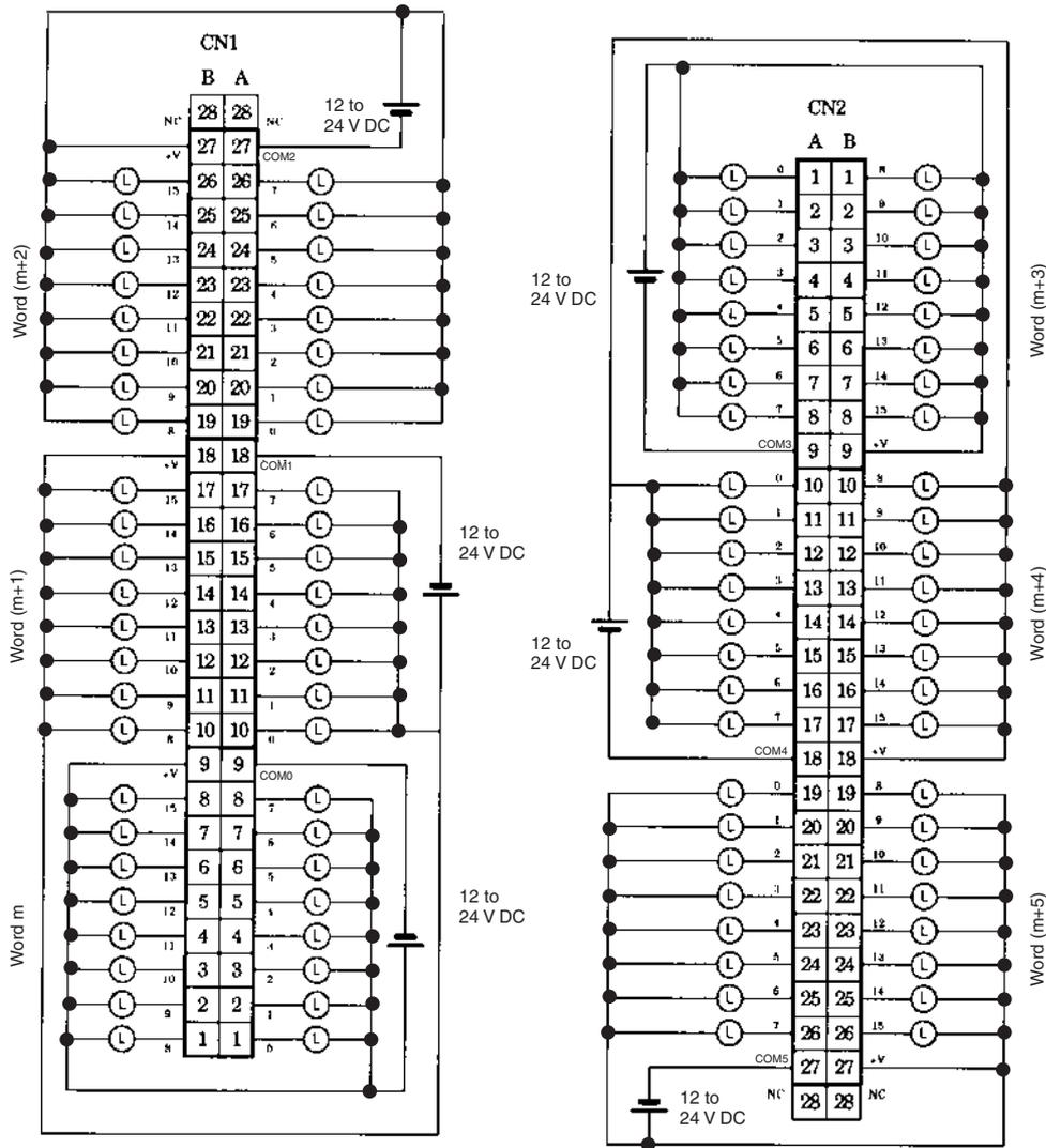
C200H-OD214 Transistor Output Unit (8 Points, Sourcing)
