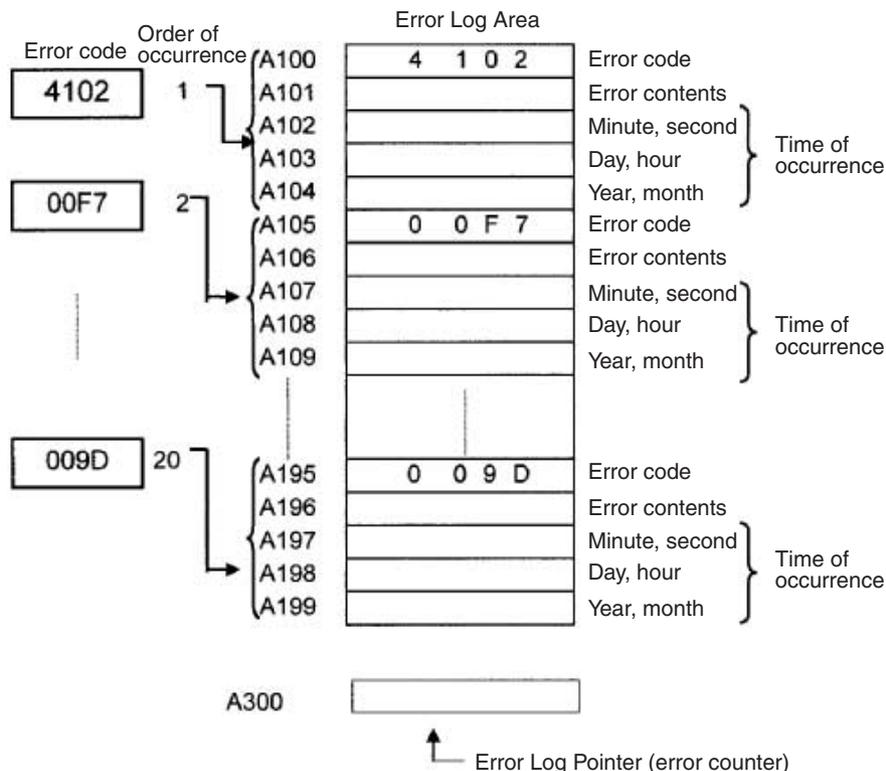
The number of records is stored in binary in the Error Log Pointer (A300). The data in the Error Log can be cleared from a Programming Device.
