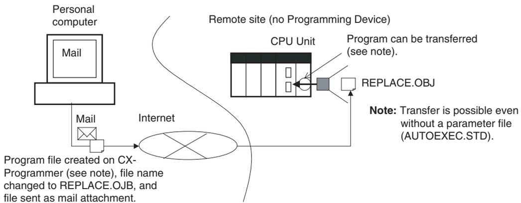
**Note** With CX-Programmer Ver. 3.0 or higher, a program file (.OBJ) can be created offline and saved on a computer storage media. Select **Transfer - To File** from the *PLC* Menu. This enable creating a program file offline without a PLC so that the name can be changed to enable sending the program file.
