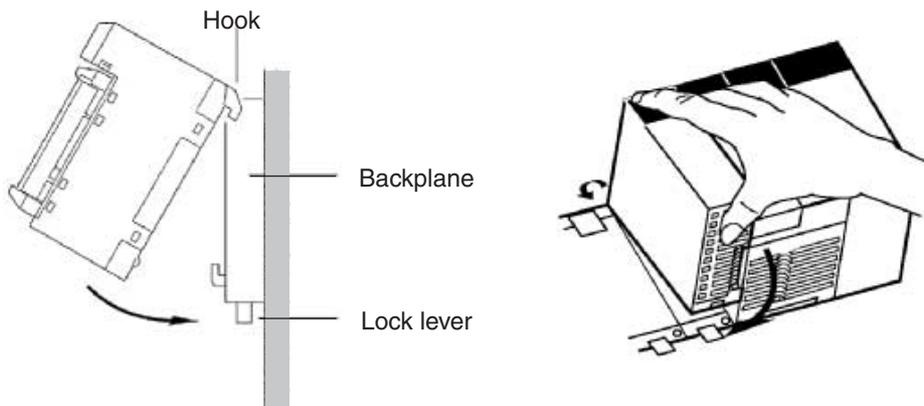
2. Make sure that the connector on the back of the Unit is properly inserted into the connector in the Backplane. (Groups A and B)
