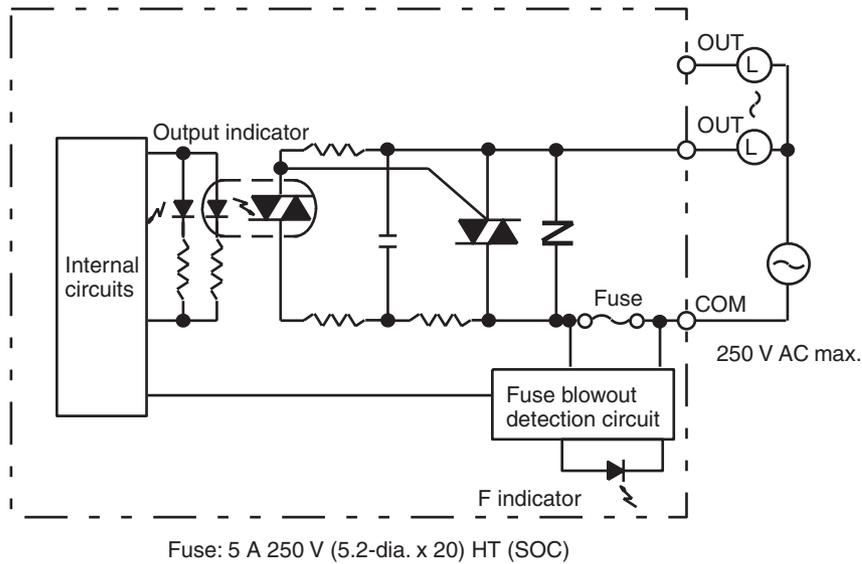
**Note** When the fuse blows, the F indicator lights and bit 08 turns ON. Bits 08 through 15 cannot be used as work bits.
