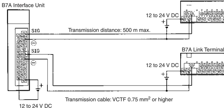
**High-speed Transmission Delays (3 ms): Shielded Cable**
