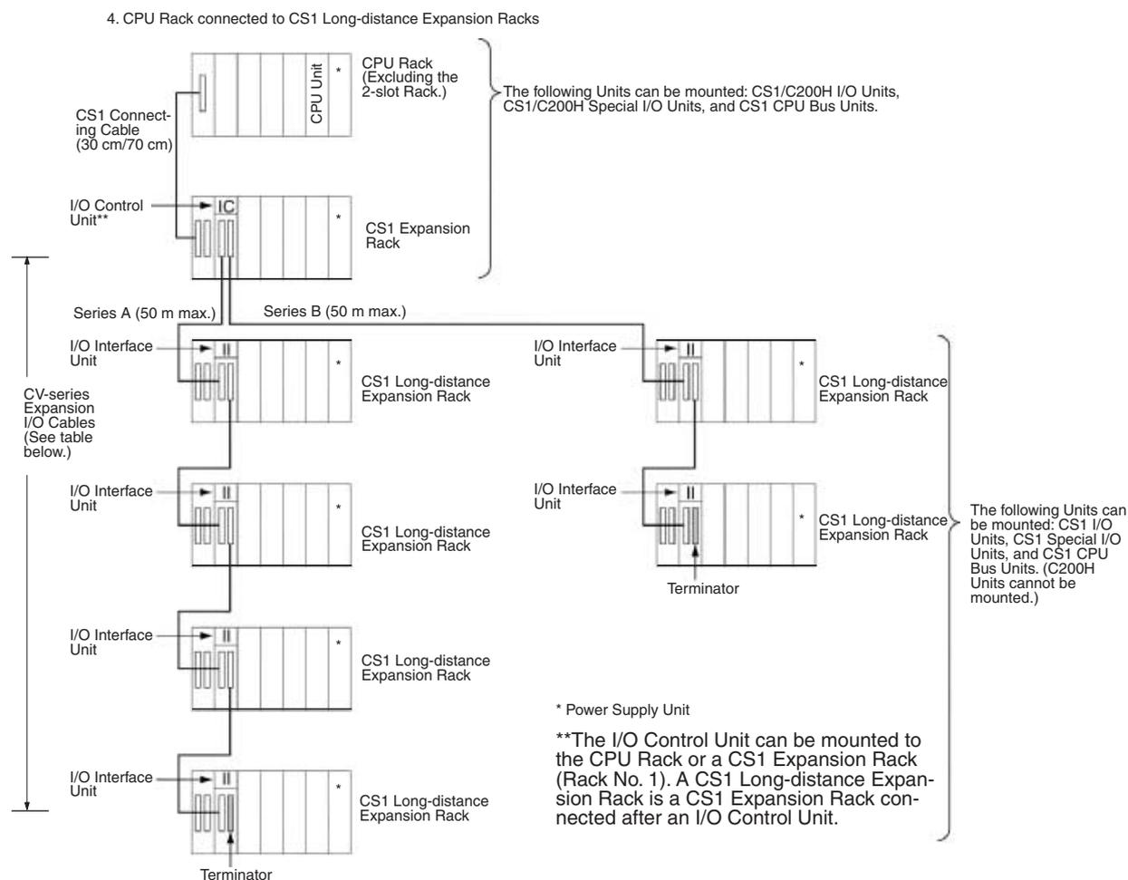
**Note** The following CV-series Expansion I/O Cables are used to connect to the CS-series Long-distance Expansion Racks (i.e., between the I/O Control Unit and the first I/O Interface Unit and between I/O Interface Units).
