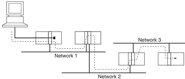
**Note** With CS/CJ-series CPU Units Ver. 2.0 or later, remote programming/monitoring is possible up to 8 levels away. Refer to 1-6-2 *Improved Read Protection Using Passwords* for details.
