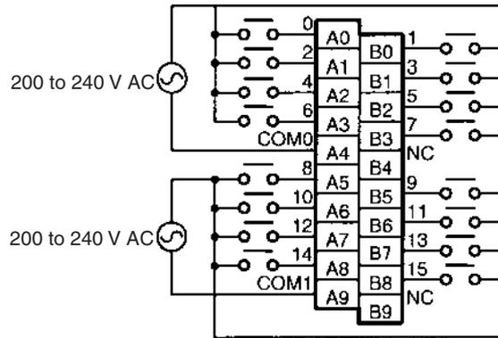
**Note** Terminal numbers A0 to A9 and B0 to B9 are used in this manual, but they are not printed on the Unit.
