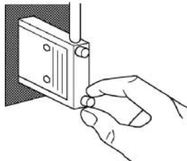
Do not route the I/O Connecting Cables through ducts that contain the I/O or power wiring.
