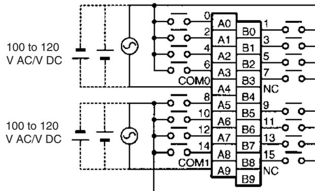
**Note** Terminal numbers A0 to A9 and B0 to B9 are used in this manual, but they are not printed on the Unit.
