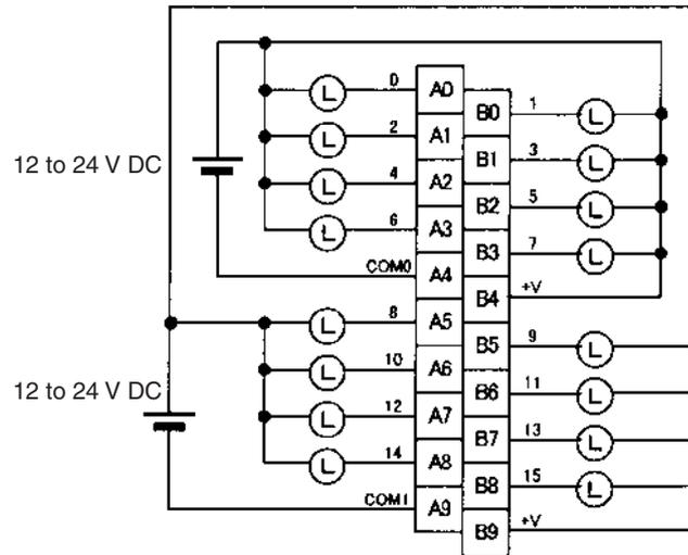
**Note** Terminal numbers A0 to A9 and B0 to B9 are used in this manual, but they are not printed on the Unit. When wiring, pay careful attention to the polarity. The load may operate incorrectly if the polarity is reversed.
