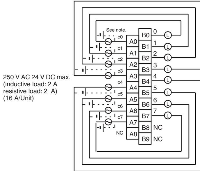
**Note:** There are no restrictions in the polarity when connecting a DC power supply.
