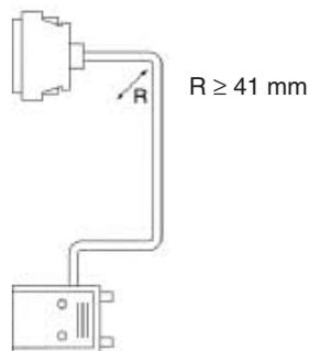
Cables for CS1 Long-distance Expansion Racks
