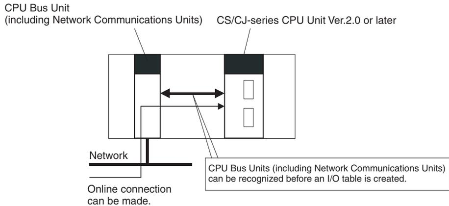
**Note** Network Communications Units include Ethernet Units, Controller Link Units, SYSMAC Link Units, and DeviceNet Units.
