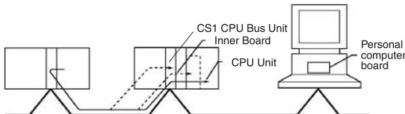
**Network-to-Serial Conversion or Network-to-Serial-to-Network Conversion**
