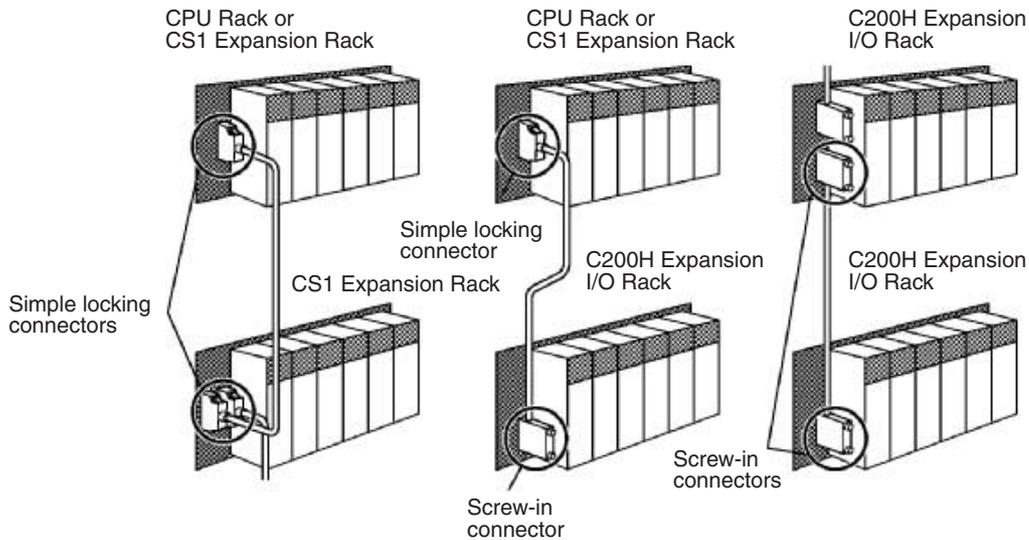
**Cables to CS-series Long-distance Expansion Racks**
