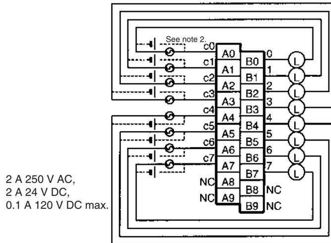
**Note:** There are no restrictions in the polarity when connecting a DC power supply.
