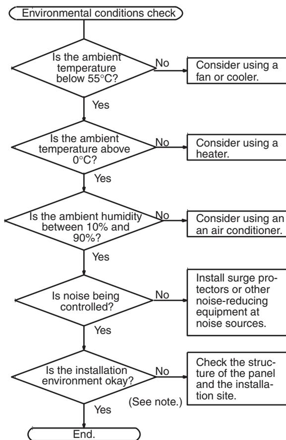
**Note** Check for corrosive gases, flammable gases, dust, dirt, salts, metal dust, direct light, water, oils, and chemicals.
