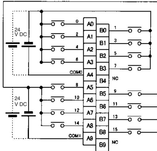
\*1 Polarity of the input power supply can be connected in either direction.
