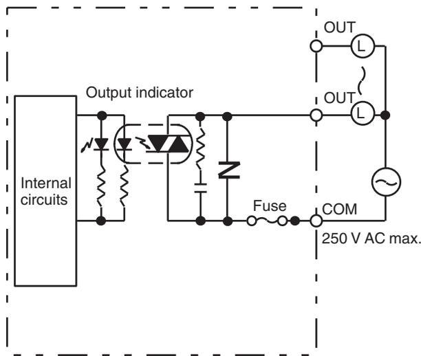
Fuse: 3 A 250 V (5.2-dia. x 20) MQ4 (SOC)
