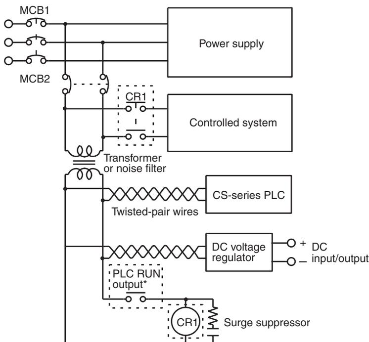
**Note** \*This configuration is possible with the C200HW-PA204R and C200HW-PA204R Power Supply Units only. When a Power Supply Unit without a RUN output is used, program the Always ON Flag (A1) as the execution condition for an output point from an Output Unit.
