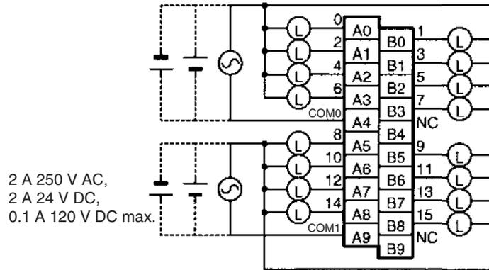
**Note** Terminal numbers A0 to A9 and B0 to B9 are used in this manual, but they are not printed on the Unit.
