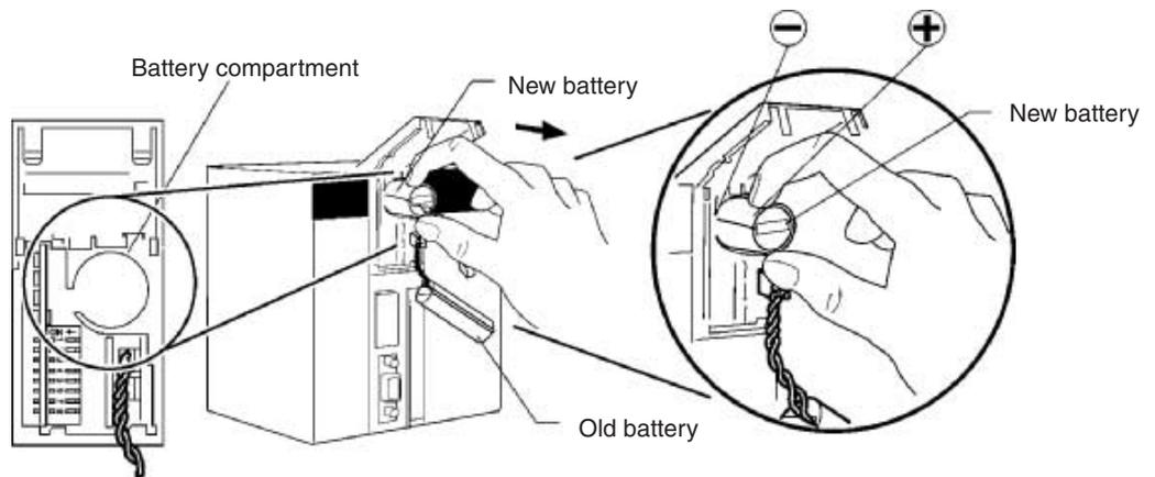
5. With the old battery connected, insert the new battery's connector in the open connector in the CPU Unit. Be sure that the connector is inserted so that its red wire is at the top and the white wire is at the bottom.
