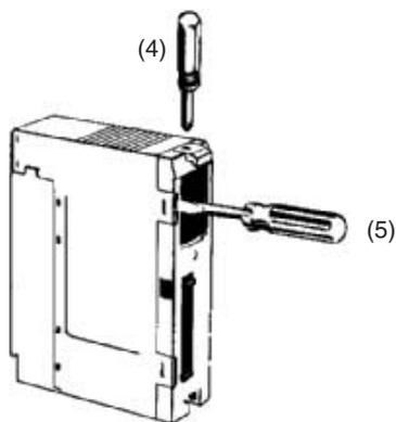
6. Pull out the printed circuit board.
