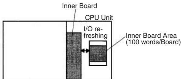
The function of the 100 words in the Inner Board Area depends upon the Inner Board being used. For details, refer to the Board's Operation Manual.
