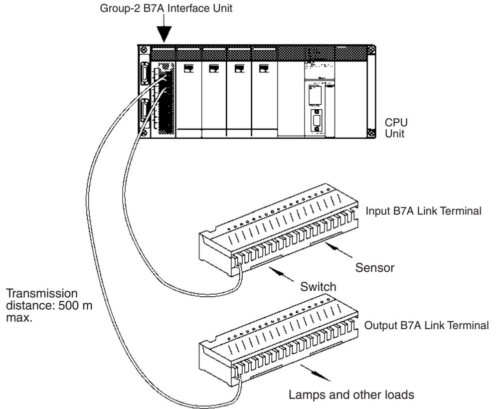
A B7A Interface Unit (C200H Group-2 High-density I/O Unit) used with two or four B7A Link Terminals allows the transmission and reception of 32-point or 64-point I/O data over two-conductor cables.
