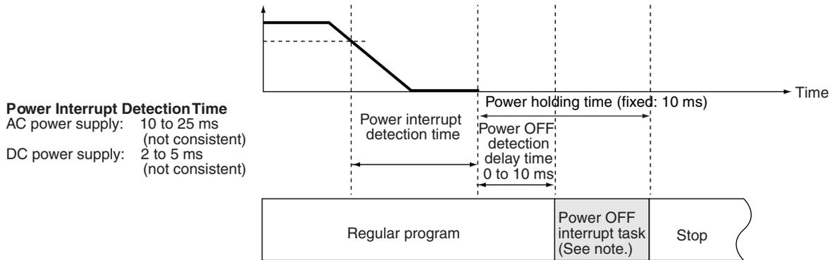
**Note** The execution time for the power OFF interrupt task must be less than the maximum time available, namely: 10 ms – power OFF detection delay time. Refer to *CS/CJ Series Programming Manual* for details on the power interrupt task and on CPU Unit operation when power is turned OFF.
