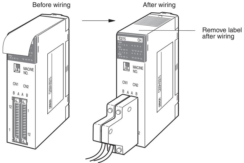
3. When solder-type connectors are being used, be sure not to accidentally short adjacent terminals. Cover the solder joint with heat-shrink tubing.
