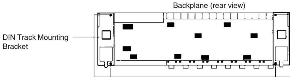
There are two Backplane mounting screws each on the left and right sides of the Backplane. Use these screws to attach the DIN Track Mounting Brackets to the Backplane. (Tighten to a torque of 0.9 N-m.)
