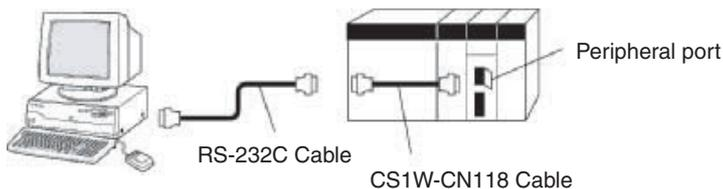
2. If cables with model numbers ending in -V instead of -CV are used to connect the computer running the CX-Programmer to the RS-232C port (in-
