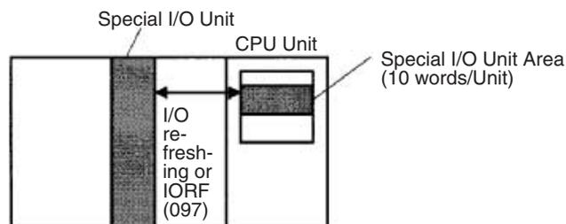
**Note** The addresses in the Special I/O Unit Area cannot be designated directly in programming or allocations inside C200H Special I/O Units.
