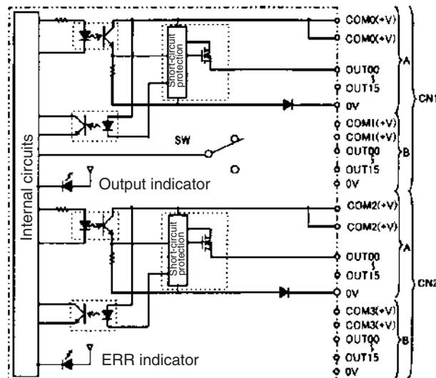
When overcurrent is detected, the ERR indicator will light. At the same time, the corresponding flag (one for each common) in the Basic I/O Unit Information Area (A050 to A089) will turn ON.
