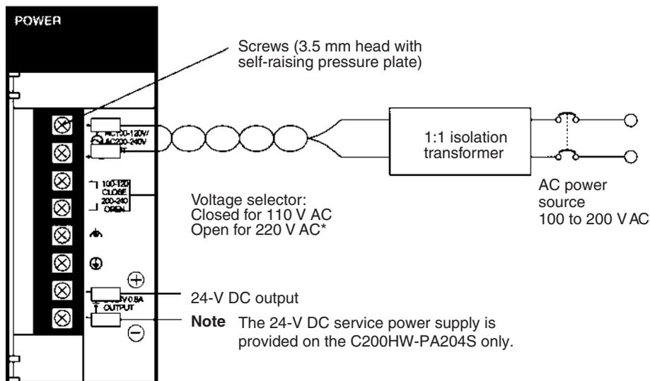
**Note** To prevent damage, be sure that the jumper bar on the voltage selector terminals has been removed before applying 220 V AC power.
