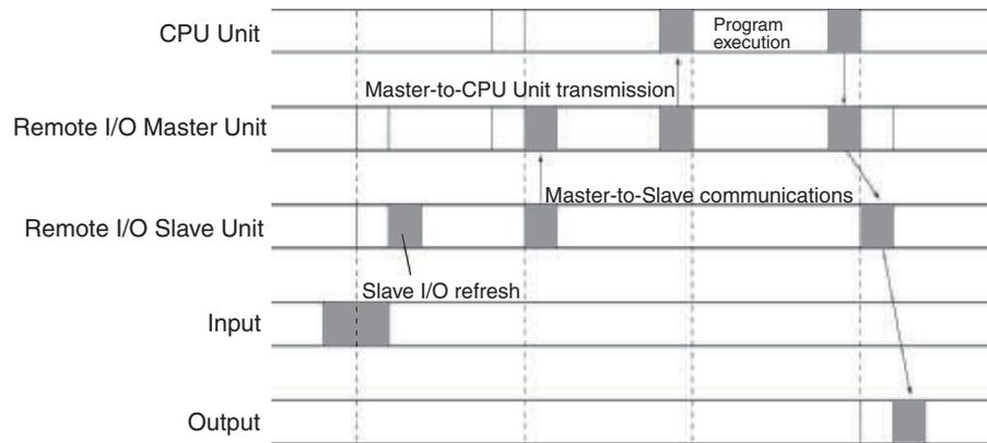
Remote I/O transmission time = (Remote I/O Slave transmission time per Slave + I/O Terminal transmission time) × 2
