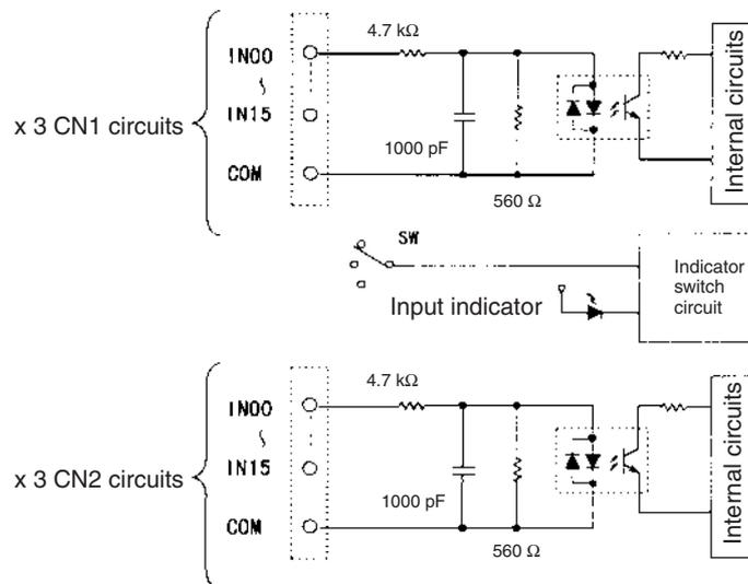
**Note** The Input ON and OFF response times for Basic I/O Units can be set to 0 ms, 0.5 ms, 1 ms, 2 ms, 4 ms, 8 ms, 16 ms, or 32 ms in the PLC Setup.
