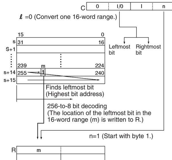
When two bytes are being converted, DMPX(077) will write the values to the bytes in R from right to left and will wrap around to the rightmost byte if the leftmost byte (byte 1) has been specified as the starting byte.
