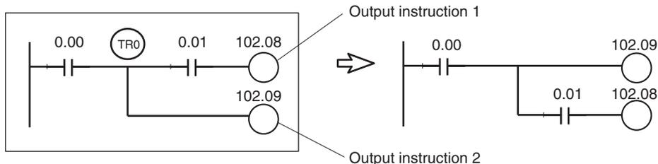
Example: A temporary storage bit TR0 output instruction and load (LD) instruction are needed at a branch point if the rungs are programmed without modification. A few steps can be eliminated by rewriting the rungs.
