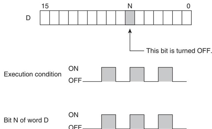
If the immediate refreshing version is not used, the status of the execution condition (power flow) is written to the specified bit in I/O memory. If the immediate refreshing version is used, the status of the execution condition (power flow) is written to the CPU Unit's output terminal as well as the output bit in I/O memory.
