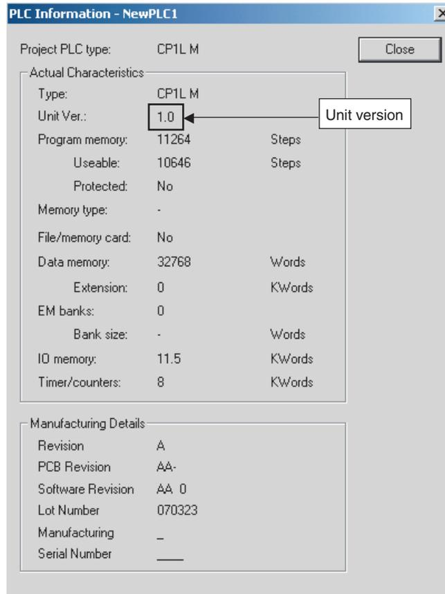
Use the above display to confirm the unit version of the CPU Unit.
