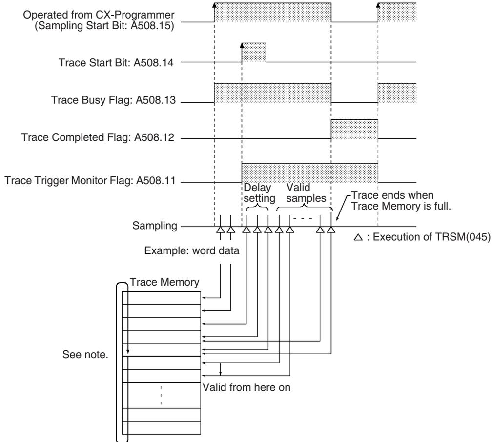
**Note** Trace Memory has a ring structure. Data is stored to the end of the Trace Memory area and then wraps to the beginning of the area, ending just before the first valid data sample.
