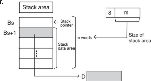
**Note** Use DISTC(566) to write stack data to the stack area.
