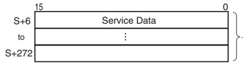
When there is Service Data (data other than the Attribute ID), the byte-order of this data is specified in bits 12 to 15 of C+1. Up to 534 bytes (267 words) can be set.
