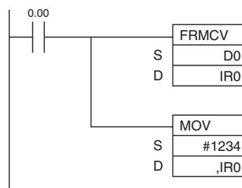
In this case, the value in D0 is 200 hex. The corresponding CV-series data area address is CIO 512. The CP-series PLC memory address for CIO 512 is 0000C0200 hex, so this value is stored in IR0. The destination operand in MOV(021) indirectly addresses the content of IR0, so #1234 is transferred to CIO 512.
