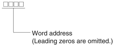
**Example:** The address of word 0010 (bits 00 to 15) in the CIO Area is given as shown below. This address is given as “CIO 10” in this manual.
