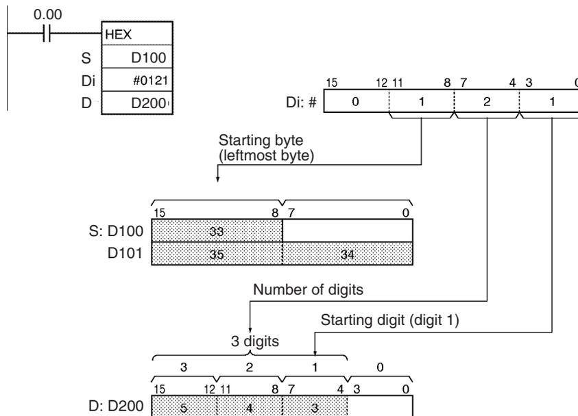
When CIO 0.00 is ON in the following example, HEX(162) converts the ASCII data in D100 beginning with the rightmost byte and writes the hexadecimal equivalents in D200 beginning with digit 1.
