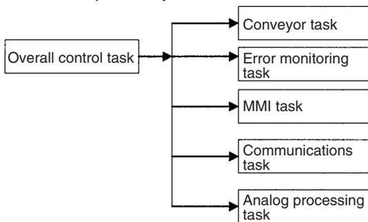
**Tasks Separated by Controlled Section**
