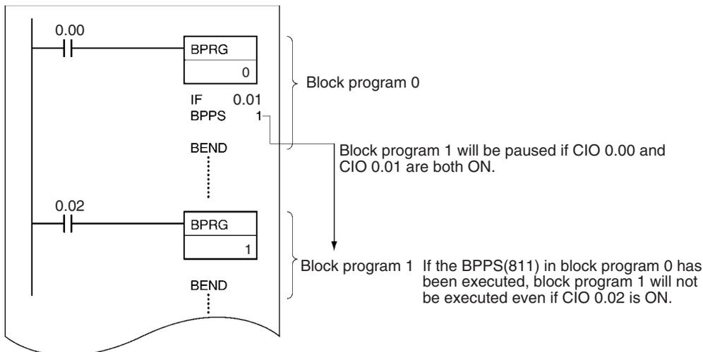
**Note** If the block program that is being paused appears after BPPS(811), it will not be executed. If the block program appears before BPPS(811), it will be paused starting the next cycle.
