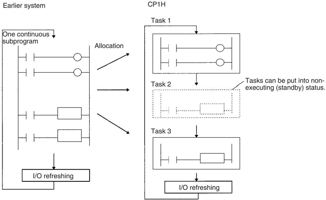
A task that has been executed will be executed in subsequent cycles, and a task that is on standby will remain on standby in subsequent cycles unless it is executed again from another task.
