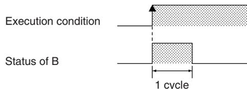
When the execution condition goes from ON to OFF, DIFD(014) turns B ON. When DIFD(014) is reached in the next cycle, B is turned OFF.
