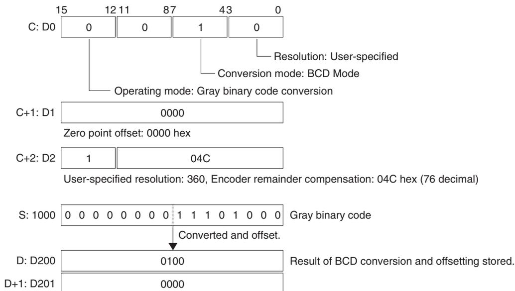
**■ Example 4: Converting to BCD Data with for an OMRON E6C2-AG5C Absolute Encoder (Resolution: 360/rotation, Encoder Remainder Compensation: 76) and Zero Point Offset of 000A Hex**
