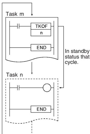
The specified task's task number is lower than the local task's task number ( $m > n$ ).
