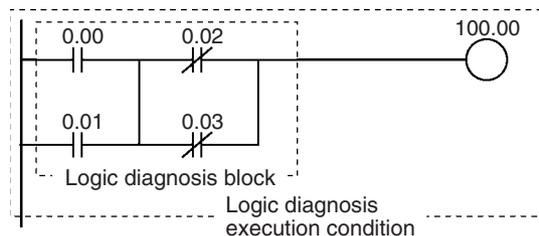
The logic diagnosis function is executed every cycle as long as the execution condition for FPD(269) is ON. The operation of the logic diagnosis function is independent of the time monitoring function.
