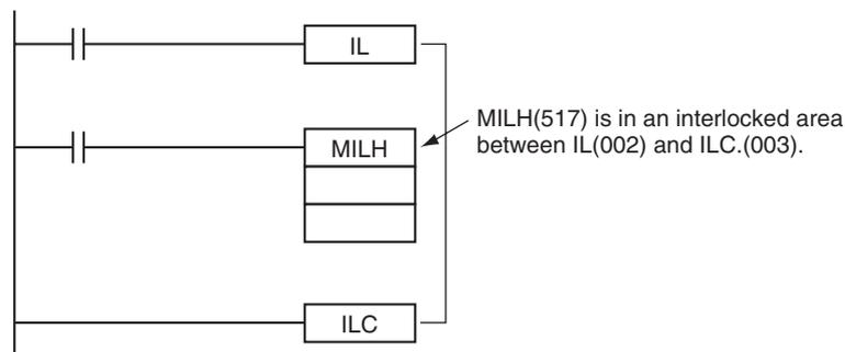
**Note** The different interlocks (IL-ILC, MILH-MILC, and MILR-MILC) can be used together as long as the interlocked program sections do not overlap.
