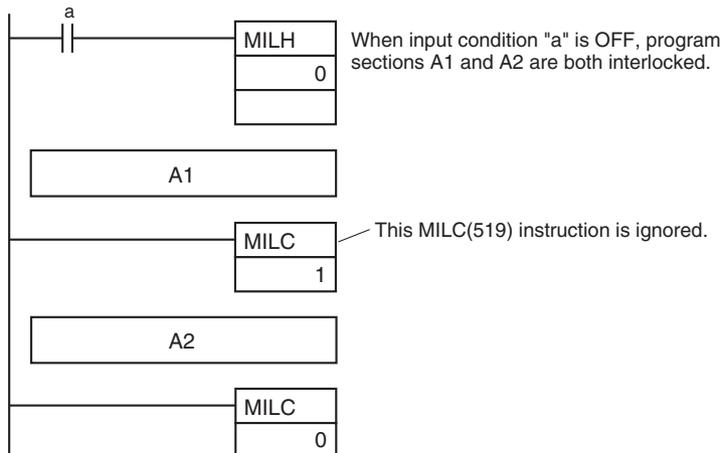
If there is an MILH(517) instruction between an IL(002) and ILC(003) pair and the IL(002) interlock is engaged, the MILH(517) instruction has no effect. In this case, the program section between IL(002) and ILC(003) will be interlocked.
