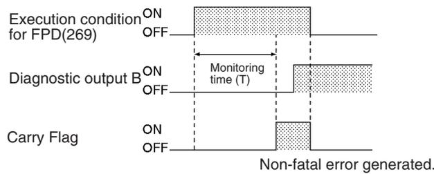
**Note** The diagnostic output must go ON within the monitoring time. The teaching function can be used set the monitoring time automatically.
