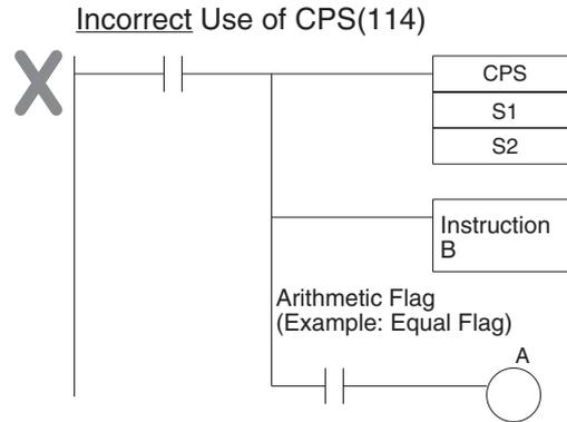
The immediate-refreshing variation (!CPS(114)) can be used with words allocated to external inputs specified in S<sub>1</sub> and/or S<sub>2</sub>. When !CPS(114) is executed, input refreshing will be performed for the external input word specified in S<sub>1</sub> and/or S<sub>2</sub> and that refreshed value will be compared.
