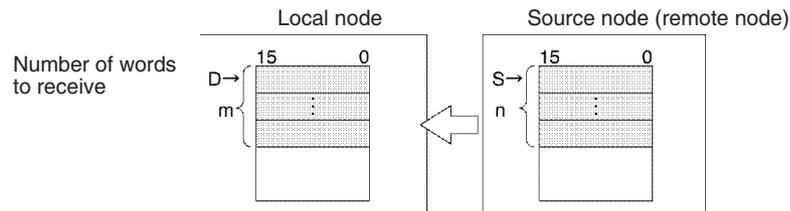
A response is required with RECV(098) because the response contains the data being received. If the response has not been received within the response monitoring time set in C+4, the request for data transfer will be retransmitted up to 15 times (retries set in bits 0 to 3 of C+3).
