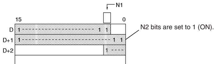
SETA(530) can be used to turn ON bits in data areas that are normally accessed by words only, such as the DM area.
