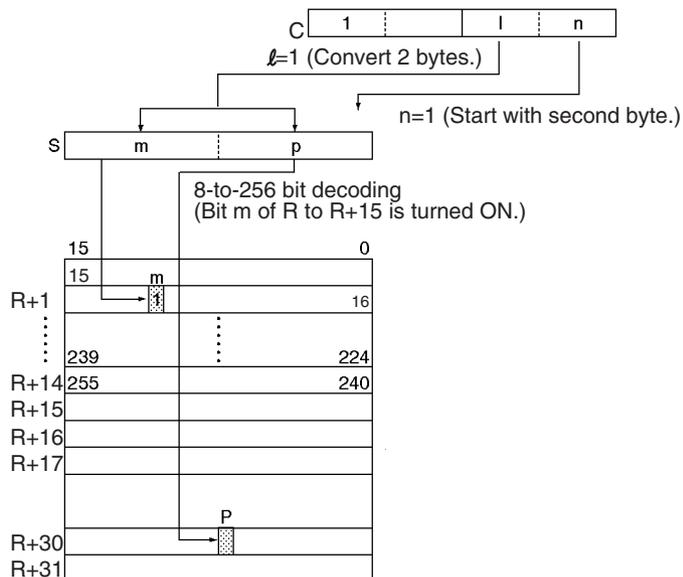
When two bytes are being converted, MLPX(076) will read the bytes in S from right to left and will wrap around to the rightmost byte if the leftmost byte (byte 1) has been specified as the starting byte.
