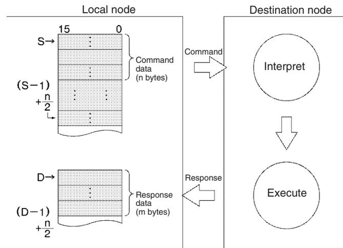
CMND(490) can be used to transmit command data to a particular serial port in the destination device as well as the device itself. CMND(490) operates just like SEND(090) if the FINS command code is 0102 (MEMORY AREA WRITE) and just like RECV(098) if the code is 0101 (MEMORY AREA READ).
