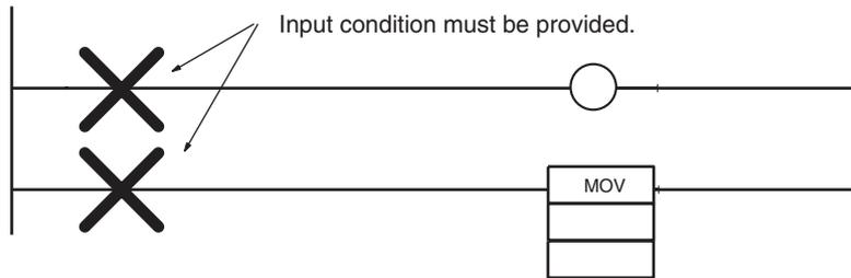
Insert an unused N.C. work bit or the ON Condition Flag (Always ON Flag) if the input must be kept ON at all times.
