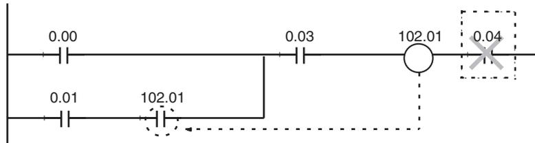
4. The same output bit cannot be programmed in an output instruction more than once. Instructions in a ladder program are executed in order from the top rung in a single cycle, so the result of output instruction in the lower rungs will be ultimately reflected in the output bit and the results of any previous instructions controlling the same bit will be overwritten and not output.
