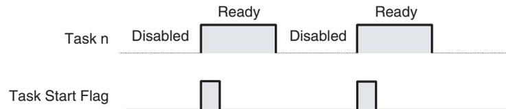
The Task Start Flag can be used to perform initialization processing whenever a task goes from Standby to RUN status, i.e., when a task on Standby is enabled using the TRON(820) instruction.
