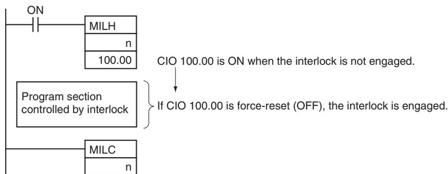
**Note** Program operation can be switched more efficiently by using interlocks with MILH(517) or MILR(518).
