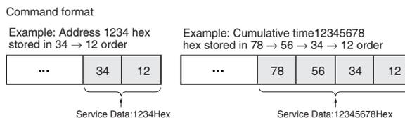
The following diagrams show how data is stored in the data areas when the service data is in 2-byte or 4-byte units.
