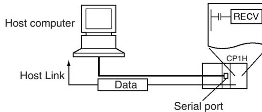
If RECV(098) is executed for the Serial Communications Option Board mounted on a CP-series CPU Unit or a CJ-series Serial Communications Unit, a command is sent from the serial port to the host computer. The command is a FINS message enclosed between a host link header and terminator. The FINS command is a MEMORY AREA READ command (command code 0101) and the host link header code is 0F hexadecimal.
