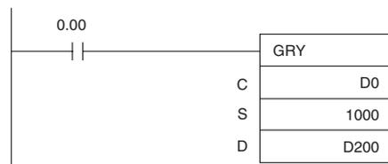
■ Example 1: Converting to Binary Data with an 8-bit Resolution and Zero Point Offset of 001A Hex
