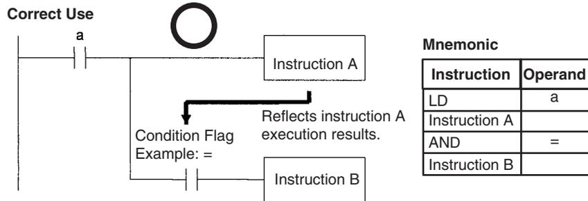
The same execution condition (a) is used for instructions A and B to execute instruction B based on the execution results of instruction A. In this case, instruction B will be executed according to the Condition Flag only if instruction A is executed.
