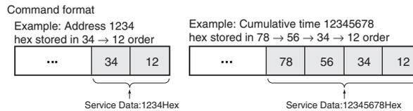
The following diagrams show how data is stored in the data areas when the service data is in 2-byte or 4-byte units.
