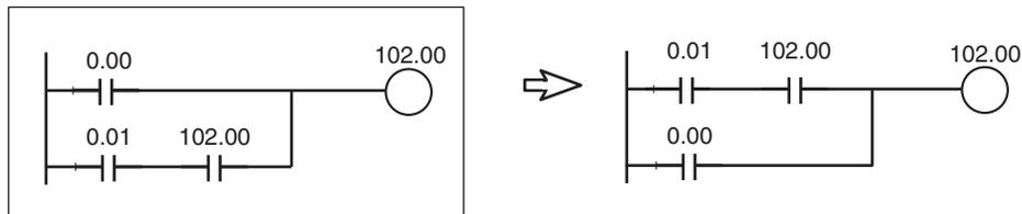
Example: An OR LD instruction will be needed if the rungs are programmed as shown without modification. A few steps can be eliminated by rewriting the rungs as shown.
