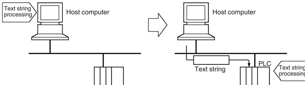
For example, production plan data such as product names can be transferred from the host computer to the PLC. Various operations such as inserting and rearranging text strings can be then be performed at the PLC, thereby reducing the data processing load at the host computer.
