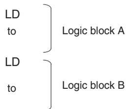
AND LD ..... Serial connection between logic block A and logic block B.
