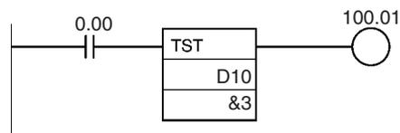
In the following example, CIO 100.02 is turned ON when CIO 0.01 is ON and bit 3 of D10 is OFF.
