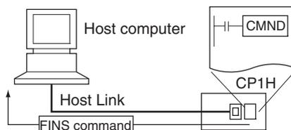
CMND(490) can be executed for the either port on the CPU Unit (Serial Communications Option Boards) or CJ-series Serial Communications Unit to send a command to the connected host computer. (Specify the serial port as 1 hex or 2 hex in bits 08 to 11 of C+2.) The command is a FINS message enclosed between a host link header and terminator. Any FINS command can be sent; the host link header code is 0F hexadecimal.
