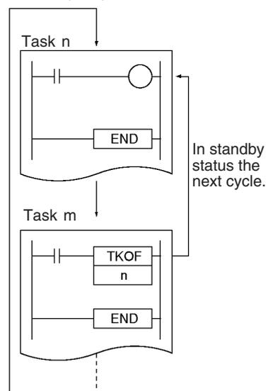
A regular task that has been set to be executed at startup will be put in executable status automatically when the PLC begins operation. All other regular tasks will be in non-executable status.
