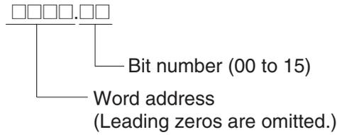
**Example:** The address of bit 03 in word 0001 in the CIO Area would be as shown below. This address is given as “CIO 1.03” in this manual.
