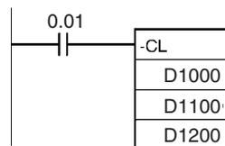
If the result of the subtraction is a negative number ( $M_i < S_u$  or  $M_{i+1}, M_i < S_{u+1}, S_u$ ), the result is output as a 2's complement. The Carry Flag (CY) will turn ON. To convert the 2's complement to the true number, a program which subtracts the result from 0 is necessary, as an input condition of the Carry Flag (CY). The Carry Flag turning ON thus indicates that the result of the subtraction is negative.
