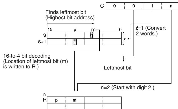
When two or more digits are being converted, DMPX(077) will write the values to the digits in R from right to left and will wrap around to the rightmost digit after the leftmost digit, if necessary.
