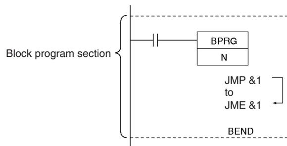
JMP(004) and JME(005) pairs must be in the same task because jumps between tasks are not allowed. An error will occur if a JME(005) instruction is not programmed in the same task as its corresponding JMP(004) instruction.
