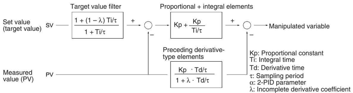
**Block Diagram for Target Value PID with Two Degrees of Freedom**
