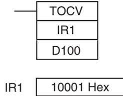
1. The CP-series PLC memory address is converted to its equivalent CP-series data area address.
