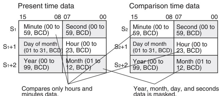
Previous data comparison instructions compared data in 16-bit units. The time comparison instructions are limited to comparing 8-bit time values.
