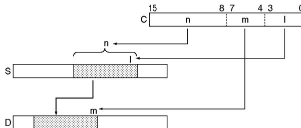
It is possible for the source words and destination words to overlap. By transferring data overlapping several words, the data can be packed more efficiently in the data area. (This is particularly useful when handling position data for position control.)
