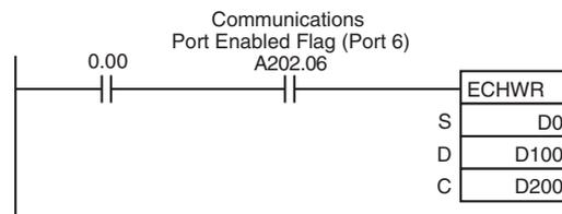
When CIO 0.00 and A202.06 (the Communications Port Enabled Flag for port 6) are ON, ECHWR(724) reads D0 to D2 from the I/O memory of the local CPU Unit and stores the data in D100 to D102 of the CJ-series CPU Unit with node address 7 on the DeviceNet Network.
