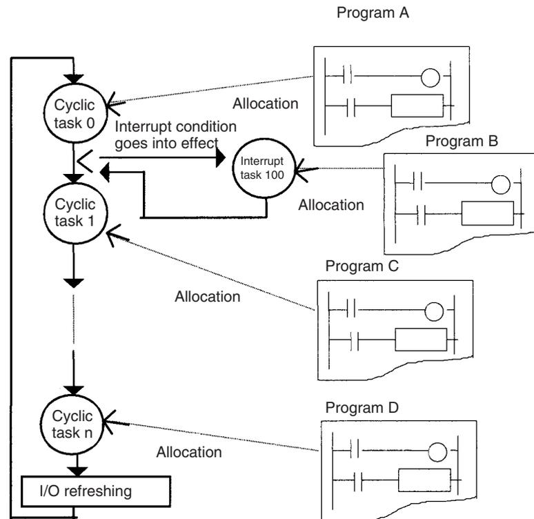
In the above example, programming would be executed in the following order: start of A, B, remainder of A, C, and then D. This assumes that the interrupt condition for interrupt task 100 was established during execution of program A. When execution of program B is completed, the rest of program A would be executed from the place where execution was interrupted.
