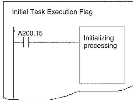
**Note** Even though a Standby cyclic task is shifted back to READY status through the TKON(820) instruction, this is not considered an initial execution and the Initial Task Execution Flag (A200.15) will not turn ON. The Initial Task Execution Flag (A200.15) will also not turn ON if a cyclic task is shifted from Disabled to RUN status or if it is put in Standby status by another task through the TKOF(821) instruction before the right to execute actually is obtained.
