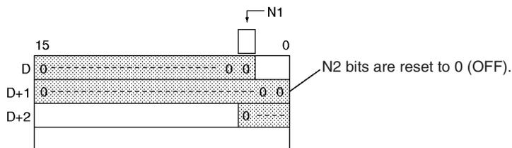
RSTA(531) can be used to turn OFF bits in data areas that are normally accessed by words only, such as the DM area.
