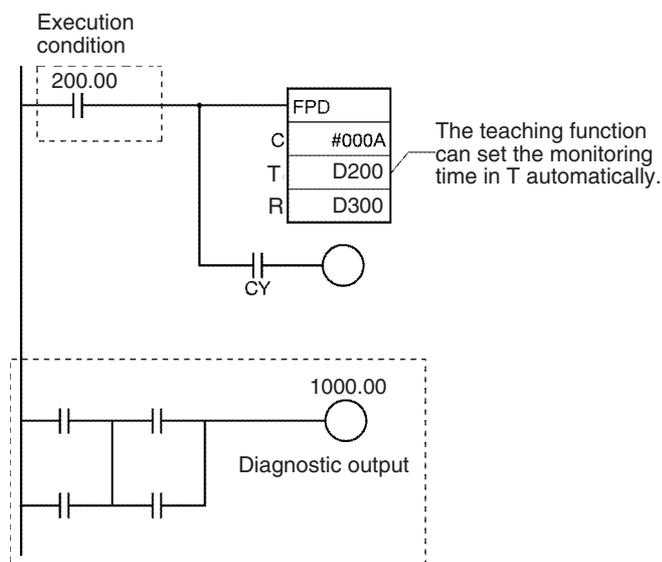
To start the teaching function, turn ON A598.00 (the FPD Teaching Bit). While A598.00 is ON, FPD(269) measures how long it takes for the diagnostic output (CIO 200.00) to go ON after the execution condition (CIO 1000.00) goes ON. If the measured time exceeds the monitoring time in T, the measured time is multiplied by 1.5 and that value is stored in T as the new monitoring time.
