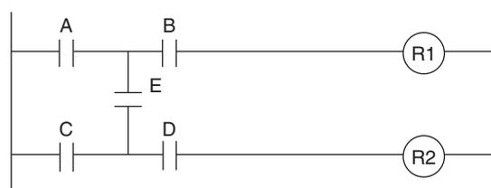
In circuit "a," coil R2 cannot be driven with contact D included.
