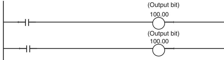
5. An input bit cannot be used in an OUTPUT instruction (OUT).
