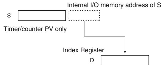
MOVRW(561) will set the PLC memory address of the timer or counter's PV in D. Use MOVR(560) to set the PLC memory address of the timer or counter Completion Flag.
