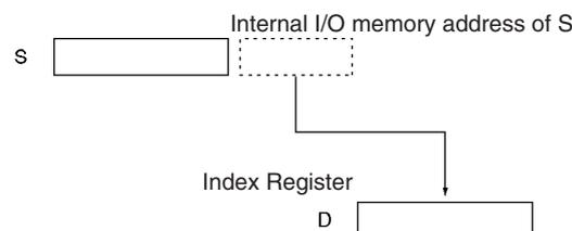
If a timer or counter is specified in S, MOVR(560) will write the PLC memory address of the timer/counter Completion Flag in D. Use MOVRW(561) to write the PLC memory address of the timer/counter PV in D.
