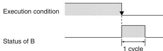
DIFU(013) and DIFD(014) have immediate refreshing variations (!DIFU(013) and !DIFD(014)). When an external output bit has been specified for B in one of these instructions, any changes to B will be refreshed when the instruction is executed and reflected immediately in the output bit for the CPU Unit built-in output.
