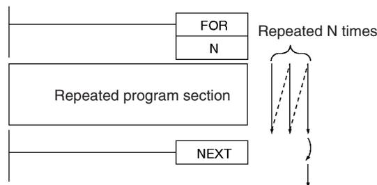
FOR-NEXT loops can be nested up to 15 levels. In the example below, program sections A, B, and C are executed as follows:
