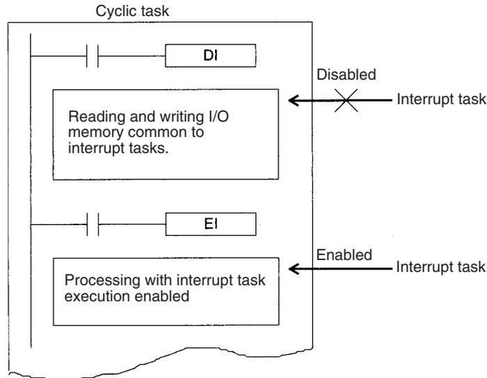
Problems may occur with data concurrency even if DI(693) and EI(694) are used to disable interrupt tasks during execution of an instruction that requires response reception and processing (such as a network instruction or serial communications instruction).
