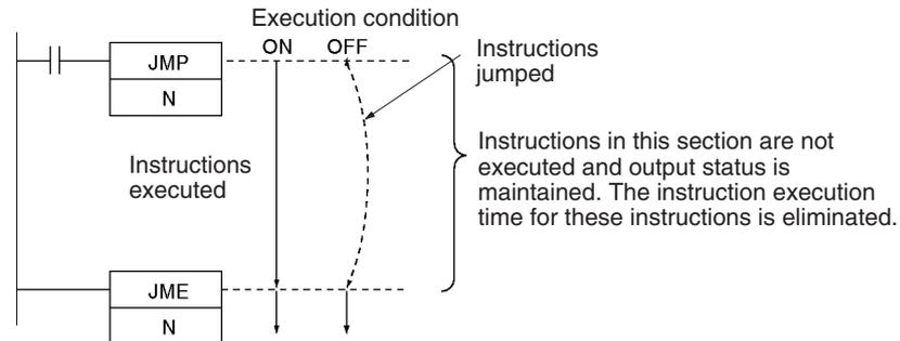
Because all of instructions between JMP(004) and JME(005) are skipped when the execution condition for JMP(004) is OFF, the cycle time is reduced by the total execution time of the skipped instructions. In contrast, NOP(000) processing is performed for instructions between JMP0(515) and JME0(516), so the cycle time is not reduced as much with those jump instructions.
