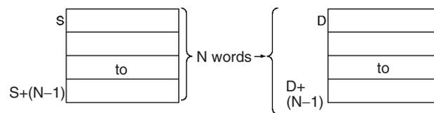
It is possible for the source words and destination words to overlap, so XFERC(565) can perform word-shift operations.
