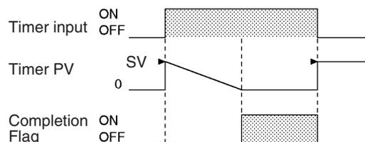
The following timing chart shows the behavior of the timer's PV and Completion Flag when the timer input is turned OFF before the timer times out.
