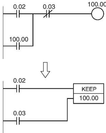
Self-maintaining bits programmed with KEEP(011) will maintain status even in an interlock program section, unlike the self-maintaining bit programmed without KEEP(011).
