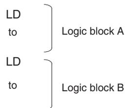
OR LD ..... Parallel connection between logic block A and logic block B.
