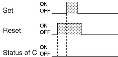
KEEP(011) has an immediate refreshing variation (!KEEP(011)). When an external output bit has been specified for B in a !KEEP(011) instruction, any changes to B will be refreshed when !KEEP(011) is executed and reflected immediately in the output bit for the CPU Unit built-in output.
