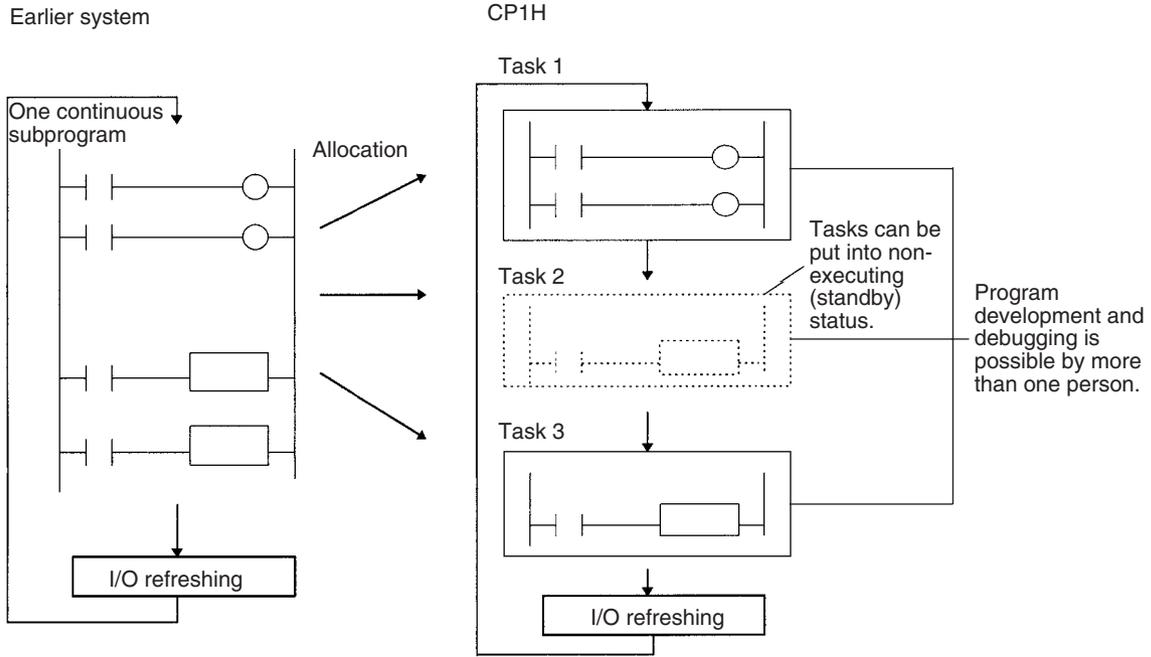
**Note** Unlike earlier programs that can be compared to reading a scroll, tasks can be compared to reading through a series of individual cards.
