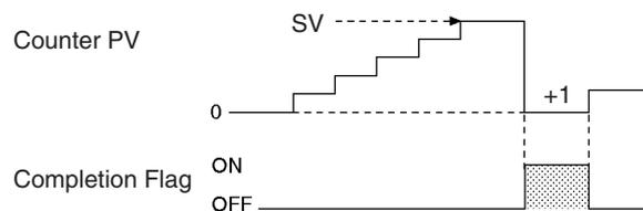
When decrementing, the Completion Flag will be turned ON when the PV is decremented from 0 up to the SV and it will be turned OFF again when the PV is decremented from the SV to SV-1.
