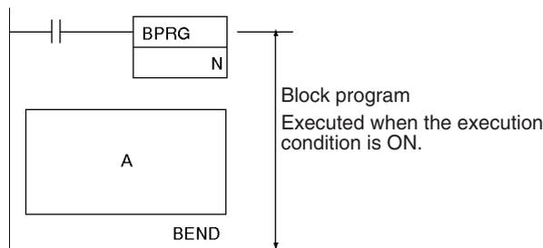
When the execution condition for BPRG(096) is OFF, the block program will not be executed and no execution time will be required for the instruction in the block program.
