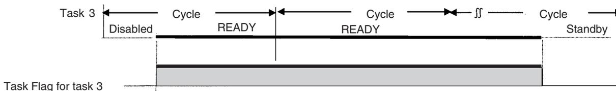
**Note** Task Flags are used only with cyclic tasks and not with interrupt tasks. With an interrupt task, A441.15 will turn ON if an interrupt task executes after the start of operation, and the number of the interrupt task that required for maximum processing time will be stored in two-digit hexadecimal in A441.00 to A441.07.
