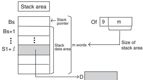
**Note** Use DISTC(566) to write stack data to the stack area.
