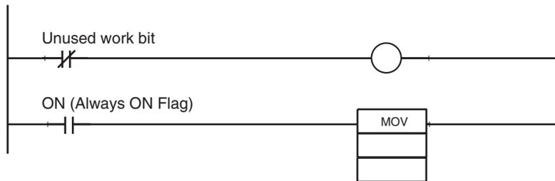
3. An input bit must always be inserted before and never after an output instruction like an output bit. If it is inserted after an output instruction, then a location error will occur during the CX-Programmer program check.
