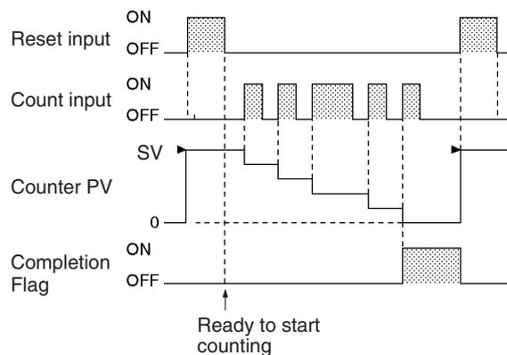
The reset input will take precedence and the counter will be reset if the reset input and count input are both ON at the same time. (The PV will be reset to the SV and the Completion Flag will be turned OFF.)
