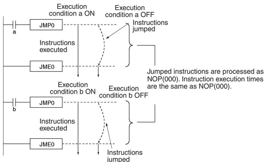
Unlike JMP(004), CJP(510), and CJPN(511) which jump directly to the first JME(005) instruction in the program, all of the instructions between JMP0(515) and JME0(516) are executed as NOP(000). The execution time of the jumped instructions will be reduced, but not eliminated. The jumped instructions themselves are not executed and their outputs (bits and words) maintain their previous status.
