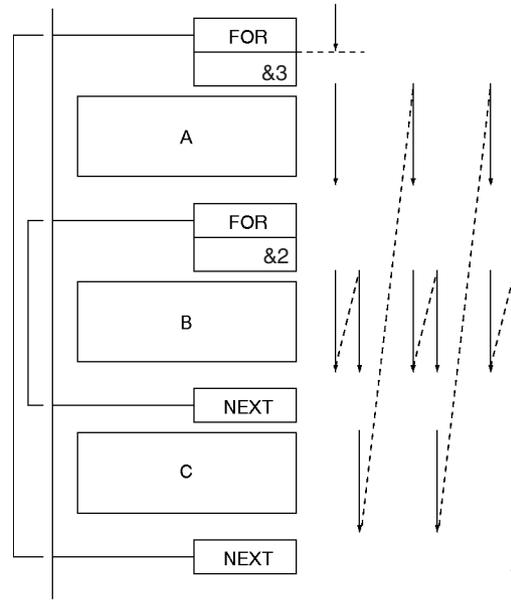
Use BREAK(514) to escape from a FOR-NEXT loop. Several BREAK(514) instructions (the number of levels nested) are required to escape from nested loops. The remaining instructions in the loop after BREAK(514) are processed as NOP(000) instructions.
