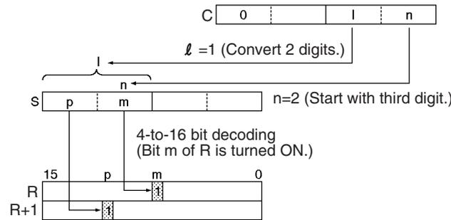
When two or more digits are being converted, MLPX(076) will read the digits in S from right to left and will wrap around to the rightmost digit after the leftmost digit, if necessary.
