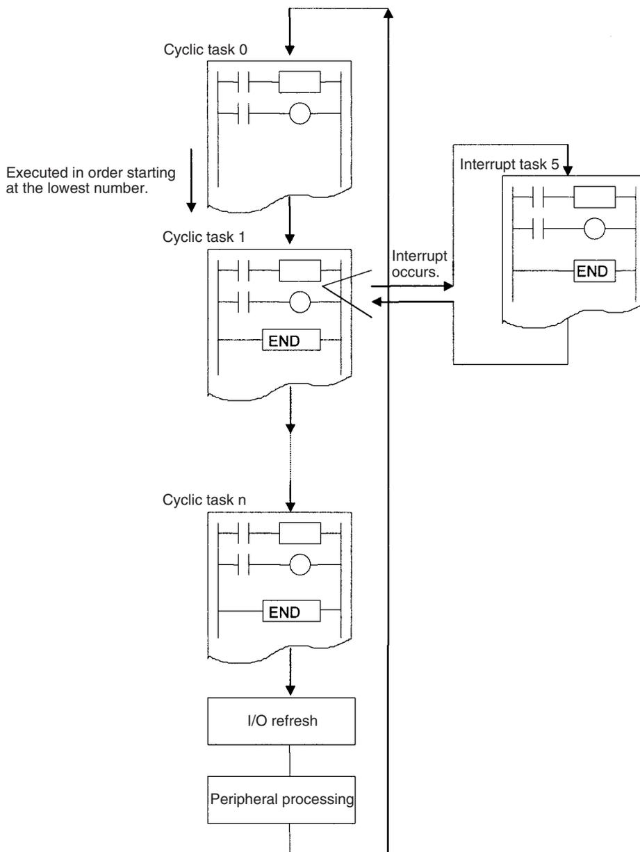
**Note** All Condition Flags (ER, CY, Equals, AER, etc.) and instruction conditions (interlock ON, etc.) will be cleared at the beginning of a task. Therefore Condition Flags cannot be read nor can INTERLOCK/INTERLOCK CLEAR (IL/ILC) instructions, JUMP/JUMP END (JMP/JME) instructions, or SUBROUTINE CALL/SUBROUTINE ENTRY (SBS/SBN) instructions be split between two tasks.
