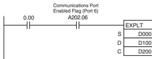
When CIO 0.00 and A202.06 (the Communications Port Enabled Flag for port 06) are ON, EXPLT(720) reads the Total ON Time (s) or Number of Contact Operations from a DRT2 Slave (I/O Terminal). In this case, the Total ON Time or Number of Contact Operations for input 3 are read.
