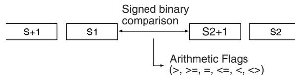
**Note** CPSL(115) treats the data in S<sub>1</sub> and S<sub>2</sub> as double signed binary data which ranges from 8000 0000 to 7FFF FFFF (-2,147,483,648 to 2,147,483,647 decimal).
