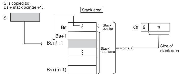
Each time that the content of S is copied to a word in the stack data area, the stack pointer in Bs is automatically incremented by +1.
