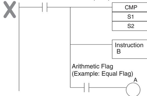
The immediate-refreshing variation (ICMP(020)) can be used with words allocated to external inputs specified in  $S_1$  and/or  $S_2$ . When ICMP(020) is executed, input refreshing will be performed for the external input word specified in  $S_1$  and/or  $S_2$  and that refreshed value will be compared.
