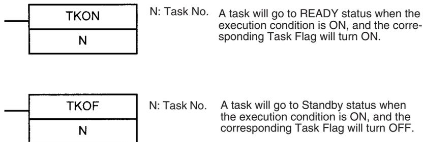
The TASK ON and TASK OFF instructions can be used to change any cyclic task (including extra cyclic tasks) between READY and Standby status at any time.
