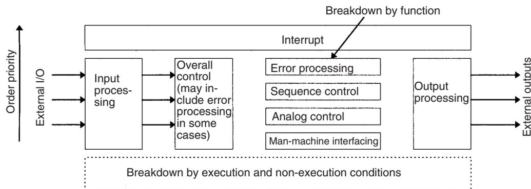
2. Be sure to break down and design programs in a manner that will ensure autonomy and keep the amount of data exchanged between tasks (programs) to an absolute minimum.
