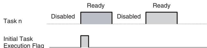
The Initial Task Execution Flag tells whether or not the cyclic tasks are being executed for the first time. This flag can thus be used to perform initialization processing within the tasks.
