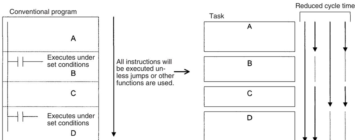
**Note** Standby status simply means that a task will be skipped during task execution. Changing to Standby status will not end the program.
