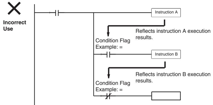
Make sure each of the results is picked up once by an OUTPUT instruction to ensure that execution results for instruction B will be not be picked up.
