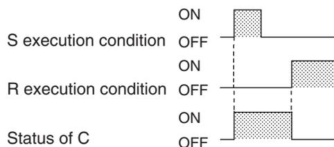
If S and R are ON simultaneously, the reset input takes precedence.
