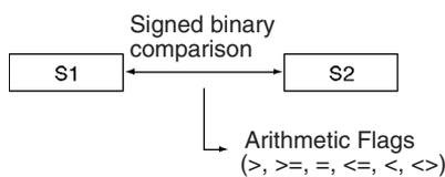
**Note** CPS(114) treats the data in S<sub>1</sub> and S<sub>2</sub> as signed binary data which ranges from 8000 to 7FFF (-32,768 to 32,767 decimal).
