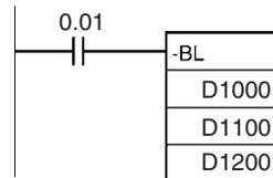
If the result of the subtraction is a negative number (Mi < Su or Mi+1, Mi < Su+1, Su), the result is output as a 10's complement. The Carry Flag (CY) will turn ON. To convert the 10's complement to the true number, a program which subtracts the result from 0 is necessary, as an input condition of the Carry Flag (CY). The Carry Flag turning ON thus indicates that the result of the subtraction is negative.
