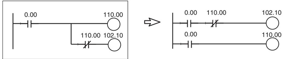
Example: CIO 102.10 in the above diagram cannot be output. By rewriting the rung, as shown above, CIO 102.10 can be turned ON for one cycle.
