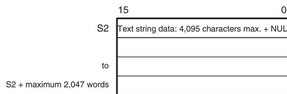
**Note** The data from S1 to S1 + the maximum 2,047 words and from S2 to S2 + the maximum 2,047 words must be in the same area.
