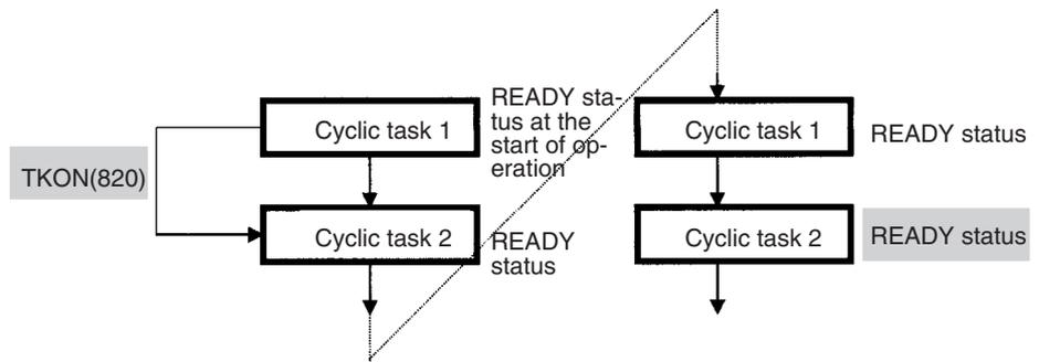
A cyclic task that is in Standby status will maintain that status in subsequent cycles. The task will have to be activated using the TKON(820) instruction in order to switch from Standby to READY status.
