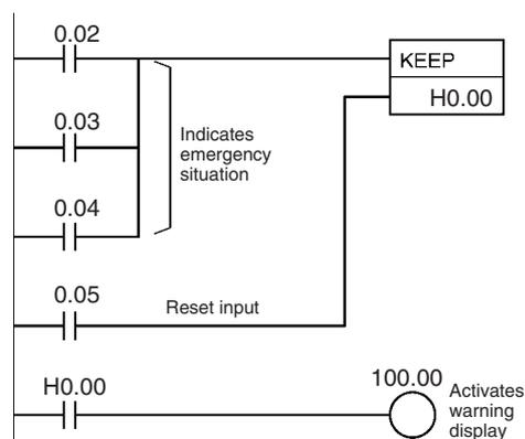
The status of I/O Area bits can be retained in the event of a power interruption by turning ON the IOM Hold Bit and setting IOM Hold Bit Hold in the PLC Setup. In this case, I/O Area bits used in KEEP(011) will maintain status after restarting the PLC following a power interruption, just like holding bits. Be sure to restart the PLC after changing the PLC Setup; otherwise the new settings will not be used.
