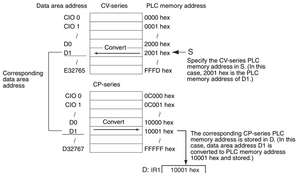
**Note** If there is no CP-series equivalent to the specified CV-series PLC memory address, an error will occur, the Error Flag will be turned ON, and the address will not be converted.
