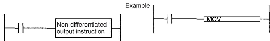
Input instructions that create logical starts and intermediate instructions read bit status, make comparisons, test bits, or perform other types of processing every cycle. If the results are ON, power flow is output (i.e., the execution condition is turned ON).
