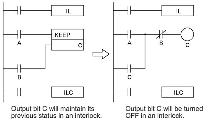
KEEP(011) can be used to create flip-flops as shown below.
