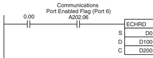
When CIO 0.00 and A202.06 (the Communications Port Enabled Flag for port 6) are ON, ECHRD(723) reads D0 to D2 from the I/O memory of the CJ-series CPU Unit with node address 7 on the DeviceNet Network and stores the data in D100 to D102 of the local CPU Unit.
