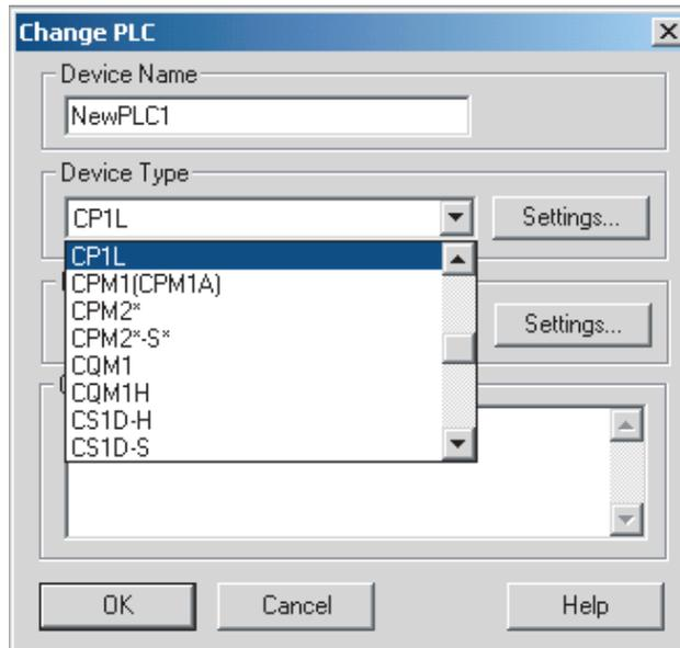
2. Click the **Settings** Button and, when the Device Type Settings Dialog Box is displayed, select the CPU type.
