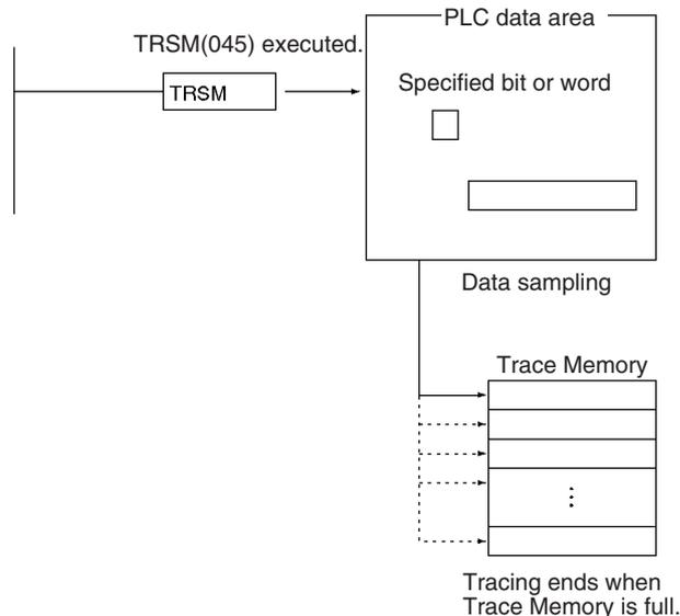
This instruction only indicates when the specified data will be sampled. All other settings and data trace operations are set with the CX-Programmer. The other two ways to control data sampling are sampling at the end of each cycle and sampling at a specified interval (independent of the cycle time).
