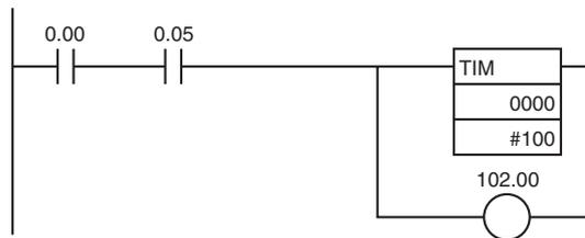
5. Output bits can also be used as input bits.
