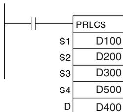
In this example, RPLC\$(654) is used to read three characters.
