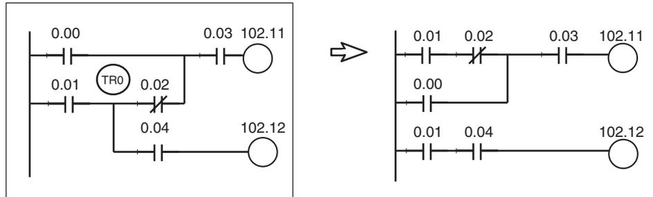
Example: The program can be written as shown in the diagram at the left where TR0 receives the branch. The same value is obtained, however, by the rungs at the right, which are easier to understand. It is recommended, therefore, that the rungs at the left be rewritten to the rungs at the right.
