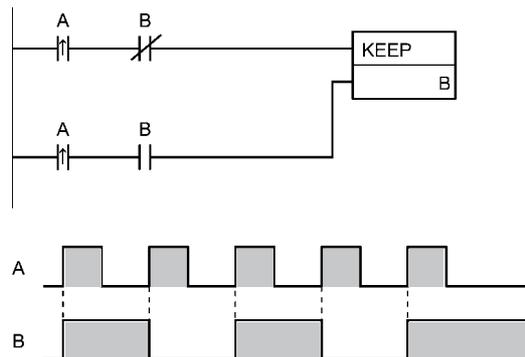
If a holding bit is used for B, the bit status will be retained even during a power interruption. KEEP(011) can thus be used to program bits that will maintain status after restarting the PLC following a power interruption. An example of this that can be used to produce a warning display following a system shut-down for an emergency situation is shown below.
