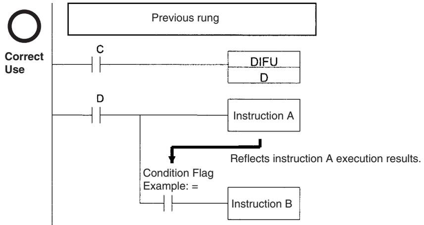
**Note** The CP1H CPU Units support instructions to save and load the Condition Flag status (CCS(282) and CCL(283)). These can be used to access the status of the Condition Flags at other locations in a task or in a different task.
