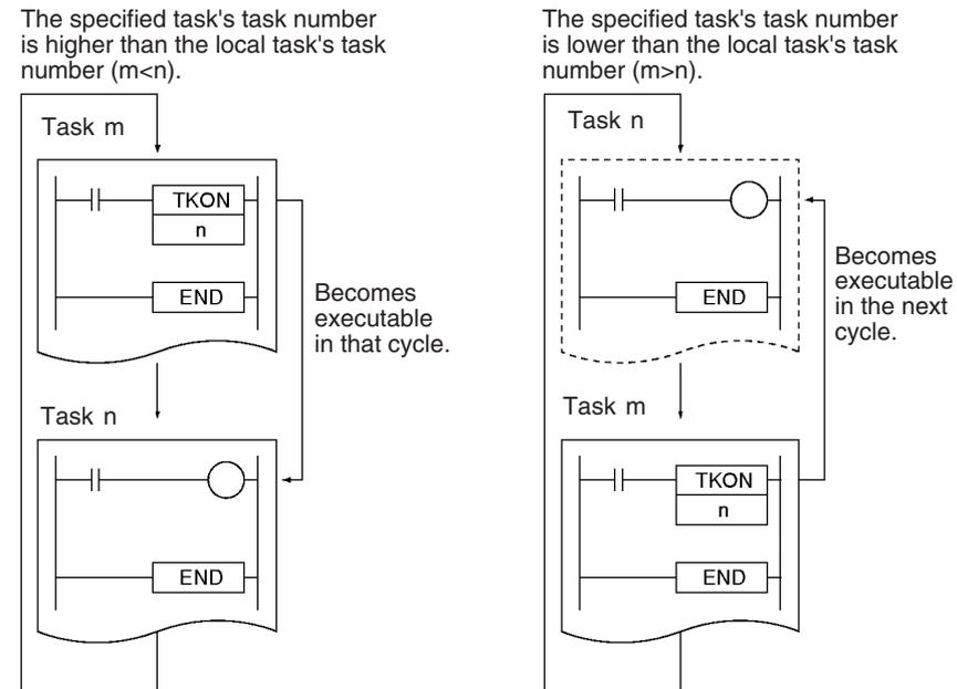
TKON(820) will be treated as NOP(000) if the specified task is already executable or the local task is specified.
