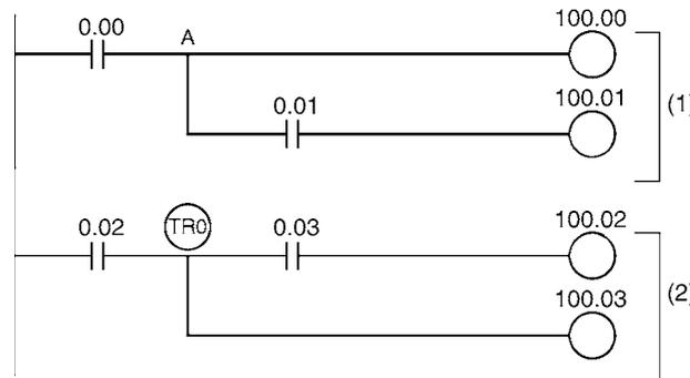
In instruction block (1), the ON/OFF status at point A is the same as for output CIO 100.00, so AND 0.01 and OUT 100.01 can be coded without requiring a TR bit. In instruction block (2), the status of the branching point and that of output CIO 100.02 are not necessarily the same, so a TR bit must be used. In this case, the number of steps in the program could be reduced by using instruction block (1) in place of instruction block (2).
