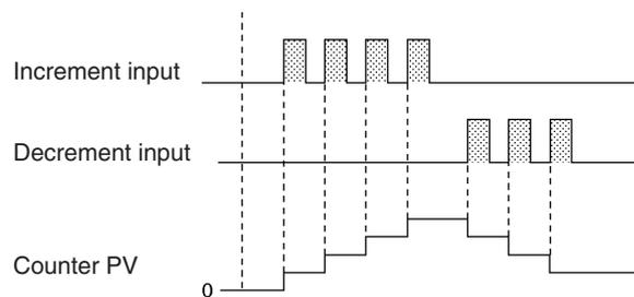
When incrementing, the Completion Flag will be turned ON when the PV is incremented from the SV back to 0 and it will be turned OFF again when the PV is incremented from 0 to 1.
