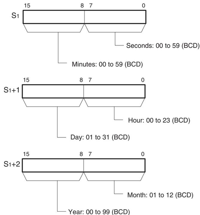
**Note** When using the CPU Unit's internal clock data for the comparison, set S<sub>1</sub> to A351 to specify the CPU Unit's internal clock data (A351 to A353).
