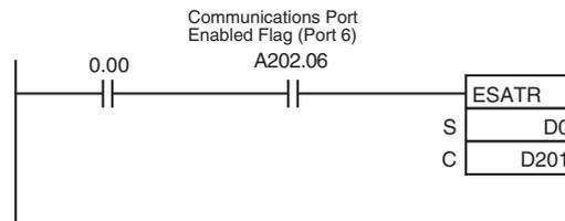
When CIO 0.00 and A202.06 (the Communications Port Enabled Flag for port 06) are ON, EXPLT(720) writes the Number of Contact Operations set value for input 2 in a DRT2 Slave (I/O Terminal).
