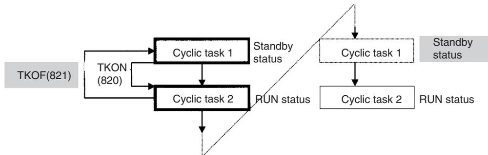
If a TKOF(821) instruction is executed for the task it is in, the task will stop being executed where the instruction is executed, and the task will shift to Standby status.
