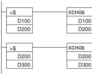
Two text strings beginning with D100 and D200 are compared in ASCII order from lower to higher. If the text string beginning with D100 is higher in ASCII order than the one beginning with D200, then the position of the two text strings will be reversed.
