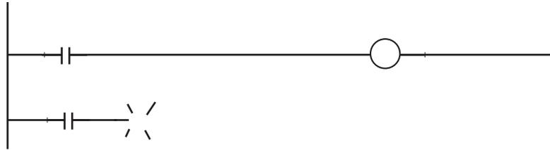
2. Output bits, timers, counters and other output instructions cannot be connected directly to the left bus bar. If one is connected directly to the left bus bar, a rung error will occur during the programming check by the CX-Programmer. (The program can be executed, but the OUT and MOV(021) will not be executed.)
