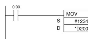
In this case, IR0 contains 10001 hex. The data area address corresponding to PLC memory address 10001 hex is D1, so #1234 is transferred to D1.
