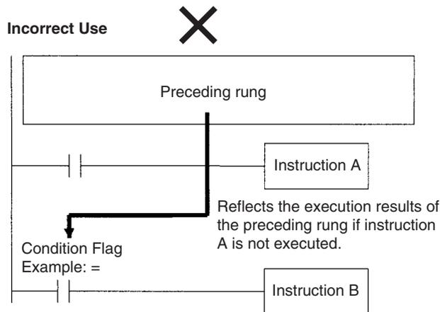
If the Condition Flag is connected directly to the left bus bar, instruction B will be executed based on the execution results of a previous rung if instruction A is not executed.
