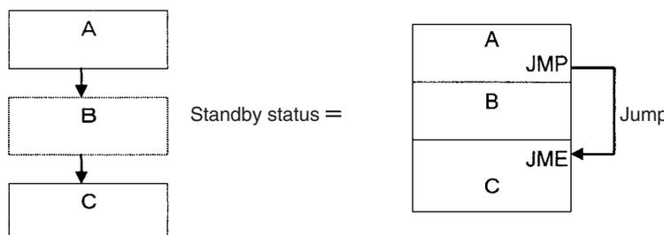
Instructions will not be executed in Standby status, so instruction execution time will not be increased. Programming that does not need to be executed all the time can be made into tasks and assigned Standby status to reduce cycle time.
