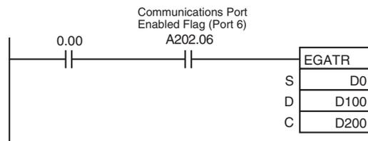
When CIO 0.00 and A202.06 (the Communications Port Enabled Flag for port 06) are ON, EGATR(721) reads the general status of the DRT2 Slave (I/O Terminal). In this case, the Total ON Time or Number of Contact Operations for input 3 are read.
