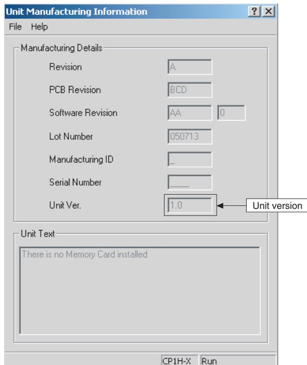
Use the above display to confirm the unit version of the CPU Unit connected online.
