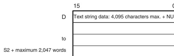
**Note** (1) The data from S1 to S1 + the maximum 2,047 words, from S2 to S2 + the maximum 2,047 words, and from D to D + the maximum 2,047 words must be in the same area.
