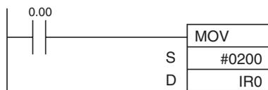
In this case, the PLC memory address 0200 hex is stored in Index Register IR0.
