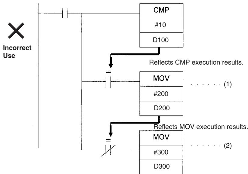
The Equals Flag will turn ON if D100 in the rung above contains #10. #200 will be moved to D200 for instruction (1), but then the Equals Flag will be turned OFF because the #200 source data is not 0000 hex. The MOV instruction at (2) will then be executed and #300 will be moved to D300. A rung will therefore have to be inserted as shown below to prevent execution results for the first MOVE instruction from being picked up.
