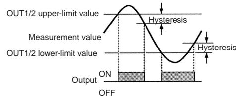
The three types of output operations shown above can be combined as desired. The following are examples of possible combinations.
