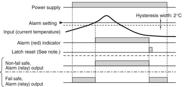
Note: The output latch is reset using the output latch reset button on the Temperature Monitoring Relay or the external input terminal.
