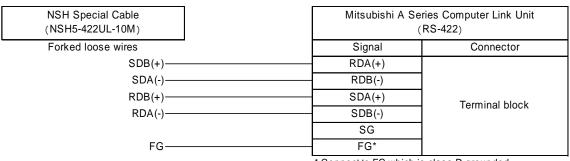
Connect to FG which is class D grounded.
