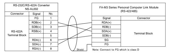
**Note:** If the PT cannot be grounded for some reason, shield wire also needs to be connected to FG of the NS-AL002.
