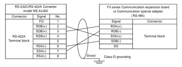
If NS cannot be grounded for some reason, shield wire also needs to be connected to FG of NS-AL002.
