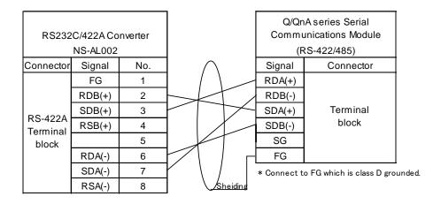
If the functional ground (FG) of the PT cannot be grounded for some reason, the shielding wire needs to be connected to the FG of NS-AL002.
