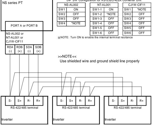
DIP SW Configuration for RS-232C/422A Converter Unit
