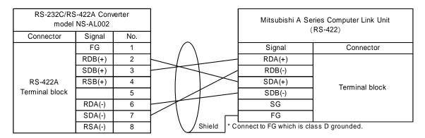
Note: If NS cannot be grounded for some reason, shield wire also needs to be connected to FG of NS-AL002.
