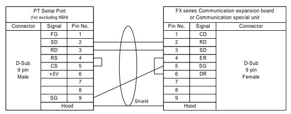
OMRON XW2Z-S002 (2m long) cable is also applicable. Even cable connection of XW2Z-S002 is not same as the connection diagram above, it is applicable because both NS and FX do not check control signals.
