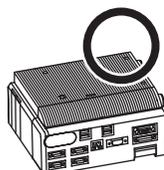
To reserve ventilation path, the feet must be mounted to the side panel that is positioned at the base.
