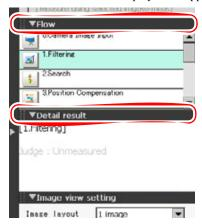
**2** When displaying both flow and detail result, you can change the size of the display area of the flow and the detail result by dragging [Detail result].
