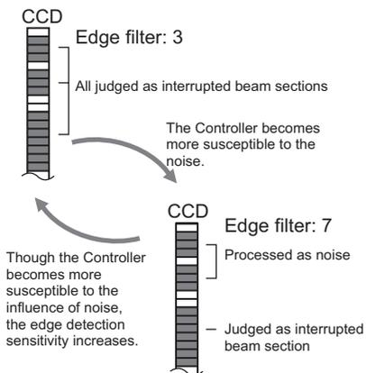
The edge filter for judging the interrupted beam section can be adjusted to suit your specific measurement requirements and the measurement object.
