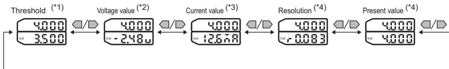
\*1: In the IC lead pitch and IC lead width judgment modes, standard values and tolerances are displayed according to the threshold switch setting.
