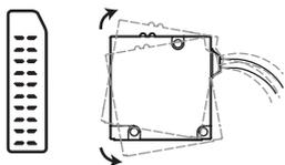
Move the emitter in the direction in which the display is missing to adjust.
