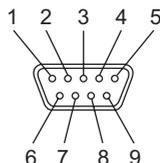
Connect the ZX-GIF\_\_ to the PC using a 9-pin D-sub (female-female) cross cable.
