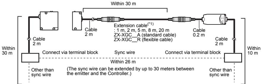
\*1: Up to two extension cables can be connected. However, be sure to limit the total extension cable length between the receiver and the Controller to 30 meters (including the receiver cable).
