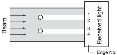
Note, however, that when the lower edge or upper edge of the beam is cut off, the lower edge or bottom edge also is counted as an edge.
