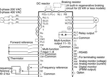
$^{\star}$  Factory default settings for relay output are NC contact for AL1 and NO contact for AL2.
