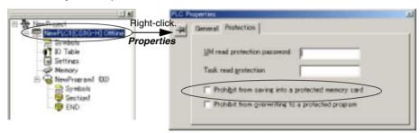
Either select PLC - Transfer - To PLC to transfer the program or select PLC - Protection - Set Password and click the OK button.
