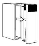
3. Align the Inner Board with the groove and slide it into the compartment.
