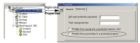
2. Either select *PLC - Transfer - To PLC* to transfer the program or select *PLC - Protection - Set Password* and click the **OK** button.
