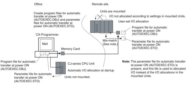
To solve this problem, the CX-Programmer had to be connected to the CPU Unit onsite to recreate the I/O tables or to delete the I/O tables to enable using the automatic I/O allocation at power ON method.
