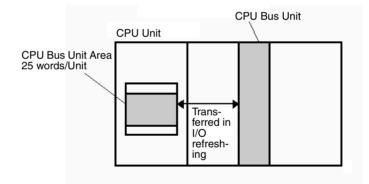
**Note** With CJ1-H CPU Units, the CPU BUS I/O REFRESH instruction (DLNK(226)) can be executed in the ladder program to refresh the CIO Area words allocated to the CPU Bus Unit of a specified unit number.
