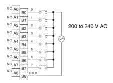
Note Terminal numbers A0 to A9 and B0 to B9 are used in this manual, but they are not printed on the Unit.
