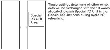
**Note** Whenever disabling a Special I/O Unit's cyclic refreshing, be sure that the I/O for that Unit is refreshed with IORF(097) or FIORF(225) (CJ1-H-R CPU Units only) in the program at least every 11 seconds during operation. A CPU Unit service monitoring error will occur in the Special I/O Unit if it is not refreshed every 11 seconds.
