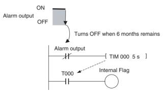
The Flag is programmed to allow for the delay in the alarm output at system startup. The Flag does not turn ON when the alarm output is ON (normal operation). When the alarm output turns OFF (replacement required), the Flag turns ON, and the replacement notification can be monitored from the system.
