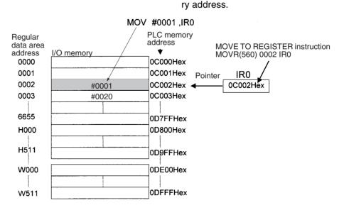
**Note** The PLC memory addresses are listed in the diagram above, but it isn't necessary to know the PLC memory addresses when using Index Registers.
