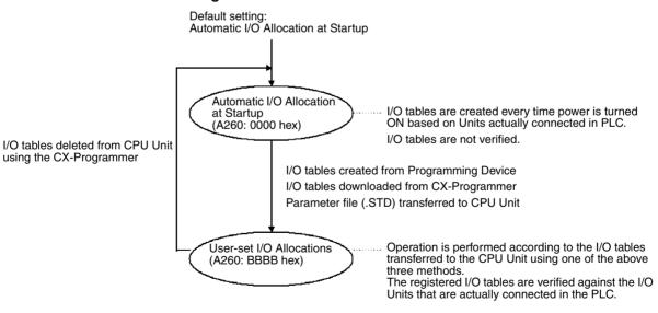
You cannot return to automatic I/O allocation at startup by using the Programming Console. To return to automation I/O allocation, the I/O tables must be deleted from the CPU Unit using the CX-Programmer. When the I/O tables are deleted, all settings for first words for Racks will also be deleted.
