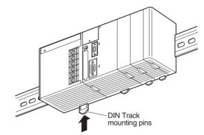
4. Install a DIN Track End Plate on each end of the PLC. To install an End Plate, hook the bottom on the bottom of the track, rotate the Plate to hook the top of the Plate on the top of the track, and then tighten the screw to lock the Plate in place.
