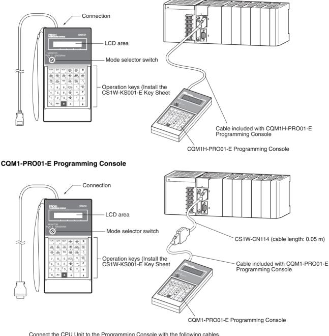
Connect the CPU Unit to the Programming Console with the following cables. CS1W-CN114 (Cable length: 0.05 m)
