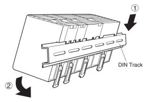
3. Lock the pins on the backs of the CJ-series Units.
