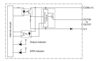
When overcurrent is detected, the ERR indicator will light, and the corresponding flag in the Basic I/O Unit Information Area (A050 to A069) will turn ON.
