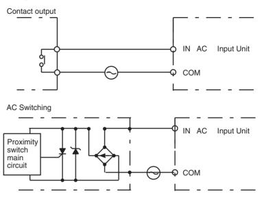
**Note** When using a reed switch as the input contact for an AC Input Unit, use a switch with an allowable current of 1 A or greater. If Reed switches with smaller allowable currents are used, the contacts may fuse due to surge currents.
