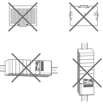
**Note** Always use the standard installation method. A nonstandard installation will decrease heat dissipation, and may delay the replacement notification signal (in particular for Power Supply Units with Replacement Notification), or degrade or damage the internal elements.
