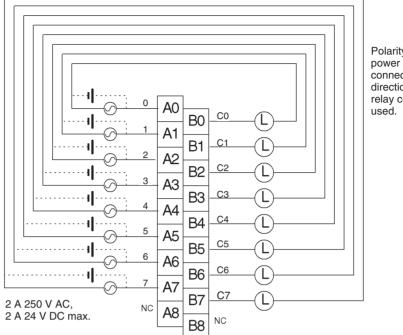
Polarity of the DC power supply can be connected in either direction because relay contacts are used.
