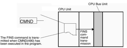
FINS commands can be transmitted to CPU Bus Units in other PLCs in the network, not just the local PLC.
