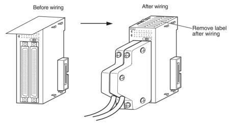
3. When solder-type connectors are being used, be sure not to accidentally short adjacent terminals. Cover the solder joint with heat-shrink tubing.
