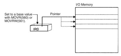
**Note** It is possible to specify regions outside of I/O memory and generate an Illegal Access Error when indirectly addressing memory with Index Registers. Refer to *Appendix D Memory Map of PLC Memory Addresses* for details on the limits of PLC memory addresses.
