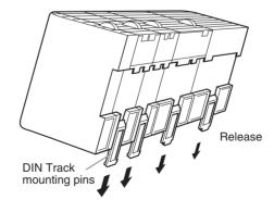
2. Fit the back of the PLC onto the DIN Track by inserting the top of the track and then pressing in at the bottom of the PLC, as shown below.
