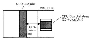
Each CPU Bus Unit is allocated 25 words based on its unit number, as shown in the following table.
