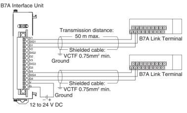
Power Supply on Both Sides (Separate Power Supplies)
