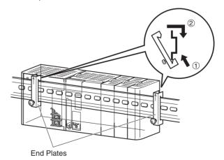
Use the DIN Track and DIN Track End Plates shown below.
