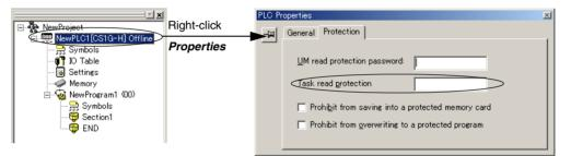
2. Select the tasks that will be password-protected and select the *Task read protect* Option in the *Program Properties* Tab.
