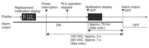
If replacement is already required, the display will turn OFF after the PC operation stops. When the display turns OFF, the alarm output will turn ON momentarily and then turn OFF again.
