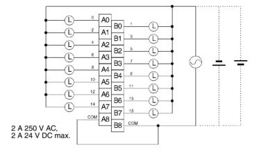
Note Terminal numbers A0 to A9 and B0 to B9 are used in this manual, but they are not printed on the Unit.
