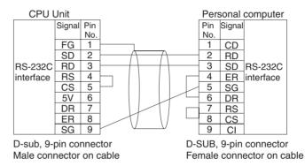
**Note** Refer to *Connection Examples* on page 655 when converting between RS-232C and RS-422A/485 to connect multiple nodes. Refer to *Recommended Wiring Methods* on page 660 when making your own RS-232C cable.
