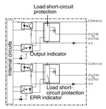
• The ERR indicator will light and the corresponding bit in A050 to A069 (Basic I/O Unit Information, two points per bit) will turn ON if an overcurrent or line disconnection is detected.
