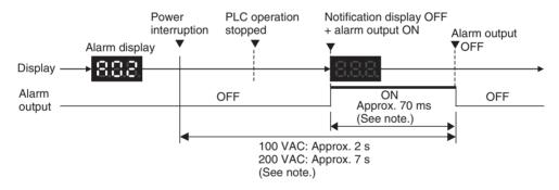
**Note** The values shown are reference values (calculated for a no-load status on the Power Supply Unit's output).
