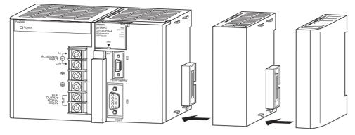
Make sure that the total power consumption of the Units is less than the maximum capacity of the Power Supply Unit.
