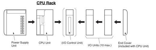
**Note** Connect the I/O Control Unit directly to the CPU Unit to enable connecting Expansion Racks.
