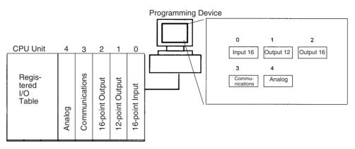
The I/O Setting Error Flag (A40110) will be turned ON if the models and locations of the Units actually mounted to the PLC (CPU Rack and Expansion Racks) do not match the information in the Registered I/O Table.
