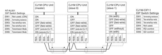
**Note** Refer to *Serial PLC Link Connection Examples (CJ1M CPU Units Only)* on page 658 for wiring diagrams and settings when using CJ1W-CIF RS-422A Converters only.
