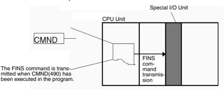
FINS commands can be transmitted to Special I/O Units in other PLCs in the network, not just the local PLC.
