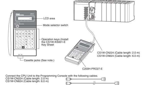
Note The cassette jacks are not used with CJ-series CPU Units.
