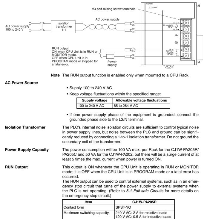
24 V DC: 2 A for resistive loads 24 V AC: 2 A for inductive loads
