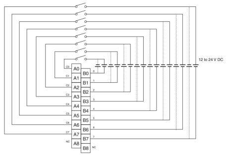
Polarity of the input power supply can be connected in either direction.
