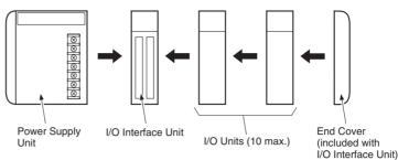
Note Connect the I/O Interface Unit directly to the Power Supply Unit.
