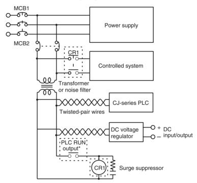
An external relay (CR1) is connected to the RUN output from the Power Supply Unit as shown in the following diagram.
