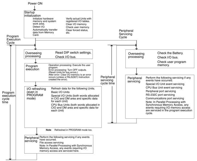
**Note** Always disconnect the Programming Console from the peripheral port during actual system operation in a Parallel Processing Mode. If the Programming Console is left attached, excess time will be allocated to increase key response for the Programming Console, adversely affecting performance.
