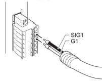
**Note** To remove the signal lines from the connector, press down on the orange tab while pulling out the signal line, as shown in the following diagram.
