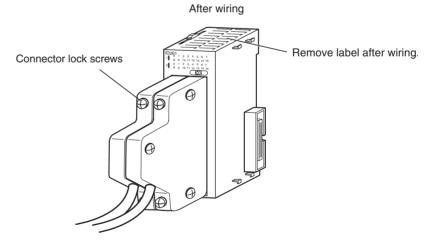
Tighten the connector-attaching screws to a torque of 0.2 N·m.
