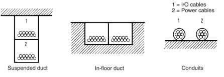
If the I/O wiring and power wiring must be routed in the same duct, use shielded cable and connect the shield to the GR terminal to reduce noise.
