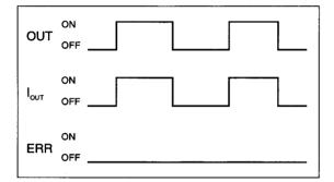
OUT: OUTPUT instruction I<sub>OUT</sub>: Output current ERR: Alarm output, ERR indicator I<sub>lim</sub>: Detection current Tj: Junction temperature of transistor Tstd: Thermal shutdown temperature Tr: Reset temperature
