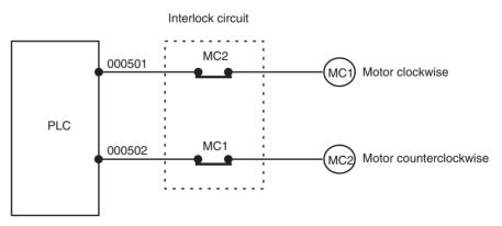
This circuit prevents outputs MC1 and MC2 from both being ON at the same time even if both CIO 000500 and CIO 000501 are both ON, so the motor is protected even if the PLC is programmed improperly or malfunctions.
