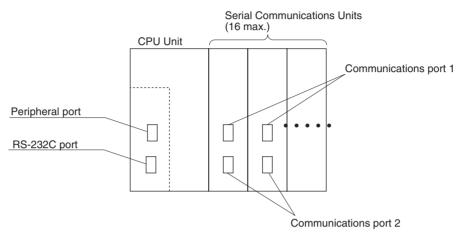
Expanding the system configuration as shown above allows a greater number of serial communications ports, and greater flexible and simpler support for different protocols.
