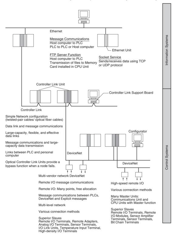
The following network systems can be configured when using CJ-series Units.
