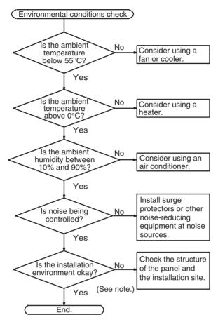
Note Check for corrosive gases, flammable gases, dust, dirt, salts, metal dust, direct light, water, oils, and chemicals.
