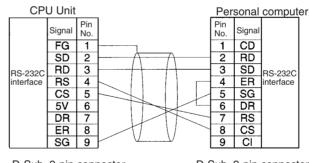
D-Sub, 9-pin connector Male connector on cable
