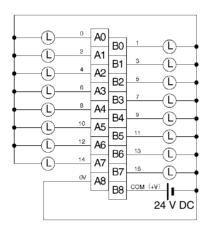
When wiring, pay careful attention to the polarity of the external power supply. The load may operate if the polarity is reversed.
