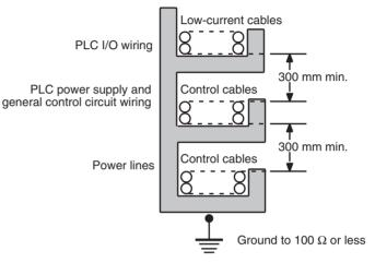
If the I/O wiring and power cables must be placed in the same duct, they must be shielded from each other using grounded steel sheet metal.
