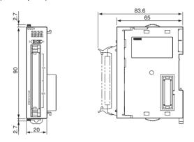
**32-point Basic Mixed I/O Units, Fujitsu-compatible Connector** CJ1W-MD231 (16 inputs/16 outputs)
