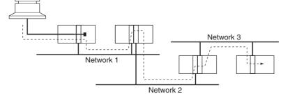
Message transfer between PLCs on a network 3 levels away (including the local network) for the same or different types of networks.
