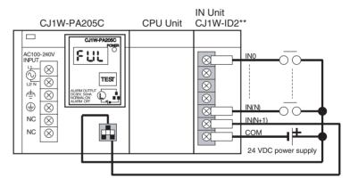
The alarm output (replacement notification output) is an NC contact. Therefore, wire the alarm output using an NC contact or other means to turn ON an error indicator or LED display as shown in the following diagram.
