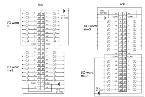
• When wiring, pay careful attention to the polarity of the external power supply. The load may operate if the polarity is reversed.
