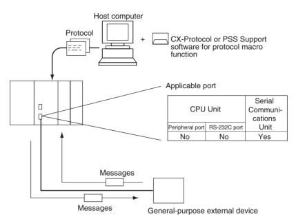
CompoWay/F (Host Function) The CJ-series CPU Unit can operate as a host to send CompoWay/F commands to OMRON components connected in the system. CompoWay/F commands are executed by using the CompoWay/F send/receive sequences in the standard protocols of the protocol macro function.
