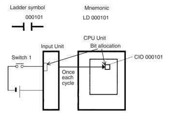
**Immediate Refreshing** When the immediate refreshing variation of an instruction is specified by inputting an exclamation point just before the instruction, and the instruction's operand is an input bit or word, the word containing the bit or the word itself will be refreshed just before the instruction is executed. This immediate refreshing is performed in addition to the normal I/O refreshing performed once each cycle.
