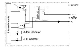
When overcurrent is detected, the ERR indicator will light, and the corresponding flag in the Basic I/O Unit Information Area (A050 to A069) will turn ON.
