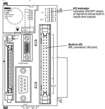
Models with Built-in I/O (CJ1M-CPU2)
