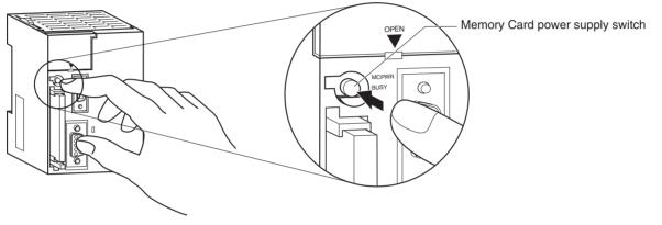
2. Press the Memory Card eject button after the BUSY indicator is no longer lit.
