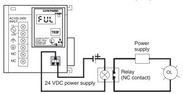
Note 1. The OL display will also light if the PLC's power supply fails.
