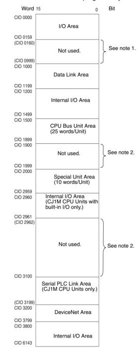
It is possible to use CIO 0080 to CIO 0999 for I/O words by making the appropriate settings for the first words on the Racks. Settings for the first words on the Racks can be made using the CX-Programmer to set the first
