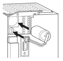
The battery error will automatically be cleared when a new battery is inserted.
