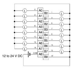
When wiring, pay careful attention to the polarity of the external power supply. The load may operate incorrectly if the polarity is reversed.
