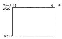
Holding Area (HR) Words in the Holding Area can be used only in the program. These words retain their content when the PLC is turned on or the operating mode is switched between PROGRAM mode and RUN or MONITOR mode.
