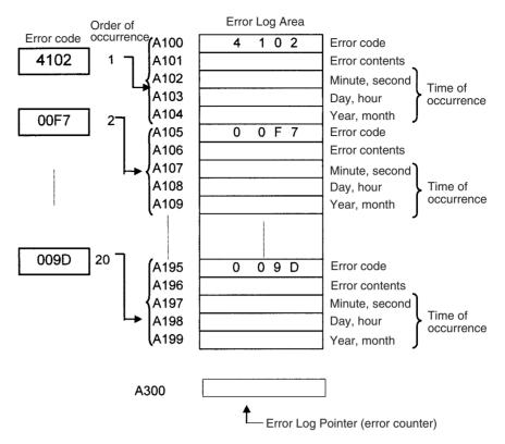
**Note** The Error Log Pointer can be reset by turning ON the Error Log Pointer Reset Bit (A50014), effectively clearing the error log displays from the Programming Consoles or CX-Programmer. The contents of the Error Log Area will not be cleared by resetting the pointer.
