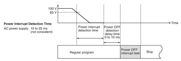
**Note** The execution time for the power OFF interrupt task must be less than the maximum time available, namely: 10 ms – power OFF detection delay time. Refer to *10-3 Power OFF Operation* for details on CPU Unit operation when power is turned OFF.
