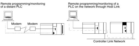
Remote programming/monitoring of a PLC on a network up to 3 levels away (including the local net-work) for the same or different types of networks is possible through Host Link.
