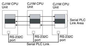
Addresses not used for Serial PLC Links can be used only in the program, the same as the Work Area.
