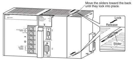
3. Attach the End Cover to the Unit on the far right side of the Rack.
