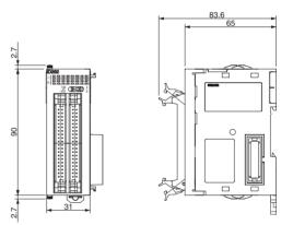
**64-point Basic Mixed I/O Units, Fujitsu-compatible Connector** CJ1W-MD261 (32 inputs/32 outputs)
