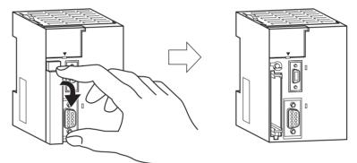
2. Insert the Memory Card with the label facing to the left. (Insert with the  $\Delta$  on the Memory Card label and the  $\Delta$  on the CPU Unit facing each other.)
