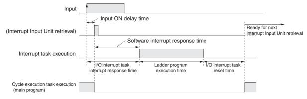
The time from when the I/O interrupt task ladder program execution is completed until the cycle execution task resumes execution is  $60 \ \mu s$ .
