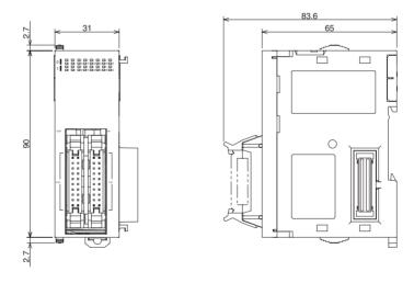
Input Units, Output Units, 24-V DC Input/Transistor Output Units, TTL I/O Units
