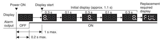
When replacement is already required, the alarm display will follow the initial display. The alarm output will turn ON approximately 0.2 seconds after the power is turned ON, and then turn OFF after approximately 5 seconds.
