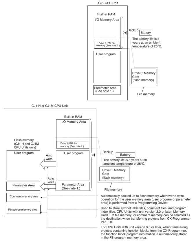
Note 1. The Parameter Area stores system information for the CPU Unit, such as the PLC Setup. An attempt to access the Parameter Area by an instruction will generate an illegal access error.
