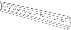
Secure the DIN Track to the control panel using M4 screws separated by 210 mm (6 holes) or less and using at least 3 screws. The tightening torque is 1.2 N·m.
