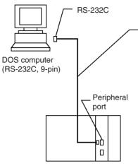
Connecting Cables for Peripheral Port
