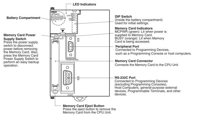
**Note** Always connect the connector covers to protect them from dust when not using the peripheral or RS-232C port.
