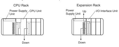
• The following diagram shows examples of proper Rack connections. Connect the simple lock connectors to the I/O Control Unit on the CJ-series CPU Rack and the I/O Interface Unit on the CJ-series Expansion Rack.
