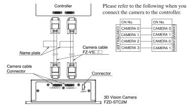
% The camera cable (FZ-VS,FZ-VSL,FZ-VSB) is polarized, so, make sure that the end bearing a name plate is connected to the Controller.
