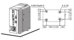
\* When mounting the controller on its bottom, it must be fixed without removing the feet to reserve ventilation path.
