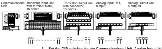
5. Set the DIP switches for the Communications Unit, Analog Input Unit, and Analog Output Unit.
