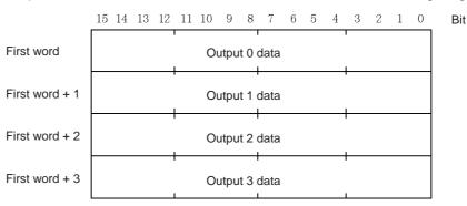
When a negative voltage is to be output, specify the conversion data as the two's complement. To obtain a two's complement from an absolute value, the NEG instruction is useful.
