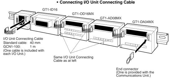
To connect each pair of Units, connect I/O Unit interface communications connector 2 on the Unit closer to the Communications Unit to I/O Unit interface communications connector 1 on the Unit closer to the end Unit.
