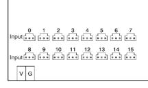
Connector Pin Arrangement The arrangement of the connectors is shown in the following diagram.
