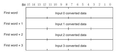
If the converted data is a negative number, it is stored as a two's complement. Data for range codes that include one digit after the decimal point are stored without the decimal point, i.e., 10 times the actual value is stored. Some examples are provided in the following table.
