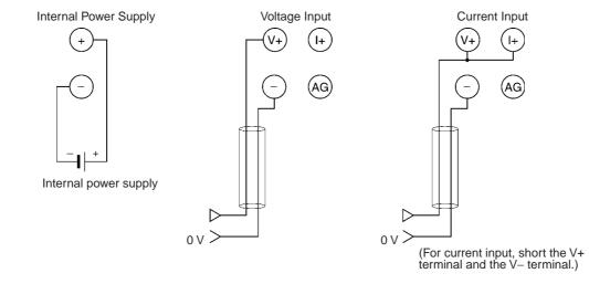
Input Ranges and Converted Data The Analog Input Unit converts analog input data to digital values. The digital values depend on the input signal ranges, as shown in the following diagrams. When the input exceeds the specified range, the AD conversion data will be fixed at either the lower limit or upper limit.
