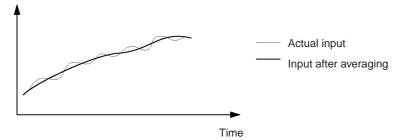
**Note** The time required for refreshing converted data remains 1 ms/point when the averaging function is enabled. The first communications data after the power is turned ON will be output after averaging eight samples.
