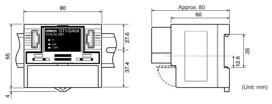
**Note** The vertical center of the Unit is 4.9 mm lower than the center of the DIN track. The Unit therefore extends downward 41.4 mm (including the mounting hook) from the DIN track center.
