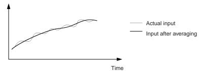
**Note** The time required for refreshing converted data remains one ms/point when the averaging function is enabled. The first communications data after the power is turned ON will be output after averaging eight samples.
