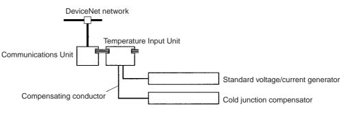
Use a calibrated thermocouple in a cold junction compensator and a compensating conductor. If using an R, S, or B thermocouple, a K thermocouple can be used instead. Set the cold junction compensator to 0°C, but disable the setting (i.e., keep the contact open) until the bias compensation described in step 10 is completed. Do not touch the Temperature Input Terminal or the compensating conductors.
