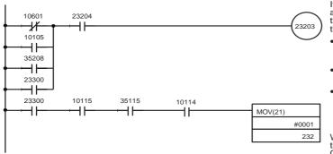
If any of the following occur after the Counter Unit setting and start-up have been completed (and 23204 is ON), the Step Advance Bit 23300 turns ON in order to reset the settings for the Counter Unit.
