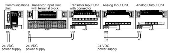
Note Be sure to separate the communications power supply, the internal power supply for the Communications Unit and the CPU Bus Unit, and the power supplies for the I/O Units. If the same power supply is used, malfunction due to noise may occur.
