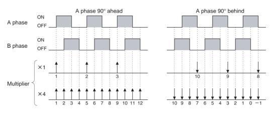
**Note** When using differential phase pulse input at a multiple function setting of  $\times 4$ , the count number for each revolution of the encoder will be 4 times the resolution of the encoder. Use an encoder that is compatible with the counting range.
