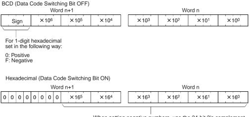
When setting negative numbers, use the 24-bit 2's complement (the last 24 bits of the 32-bit 2's complement). Example: To set -10,000-10,000 (decimal)  $\rightarrow$  FFFF D8F0 Hex (32 bit 2's complement)  $\rightarrow$ FF D8F0 Hex (24 bit 2's complement)
