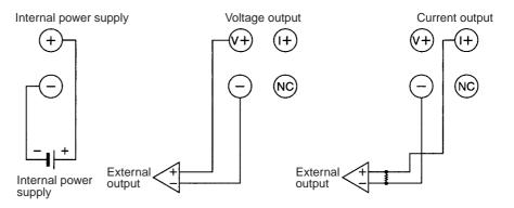
Output Ranges and Converted Data The Analog Output Unit converts the digital output data to analog values. The analog values depend on the output signal ranges, as shown in the following diagrams.
