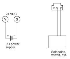
**Note** V terminals and V connector pins, as well as G terminals and G connector pins, are internally connected. When the I/O power is being supplied from a terminal block, the power can be supplied to the output devices from the V and G connectors. Current supplied in this way, however, must be less than 2 A.
