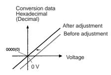
The possible range of offset adjustment depends on the input range. Refer to the following table.
