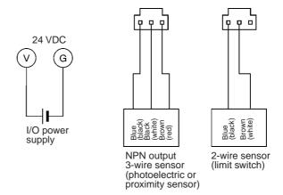
Wire colors in parentheses are the previous JIS colors for photoelectric and proximity sensors.
