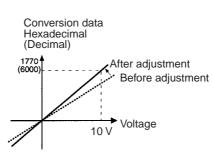
The possible range of gain adjustment depends on the input range. Refer to the following table.
