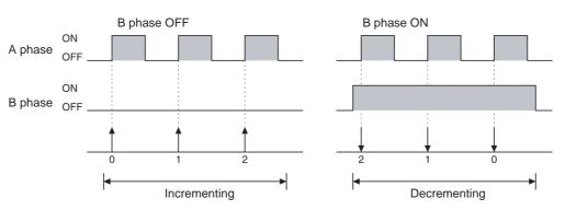
**Note** Switching B phase (direction input) ON and OFF, must be carried out with A phase (pulse input) switched OFF.
