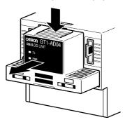
2. Insert the new Cassette as far as possible into the space, taking care about its orientation. After doing so, try to gently pull the Cassette outwards to check whether it is secure.
