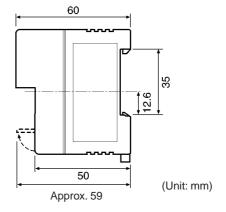
**Note** The vertical center of the Unit is 4.9 mm lower than the center of the DIN track. The Unit therefore extends downward 41.4 mm (including the mounting hook) from the DIN track center.
