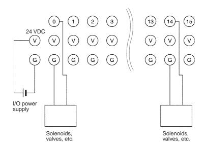
**Note** V terminals and G terminals are internally connected. When the I/O power is being supplied, the power can be supplied to the output devices from the V terminals and G terminals. Current supplied in this way, however, must be less than 4 A.
