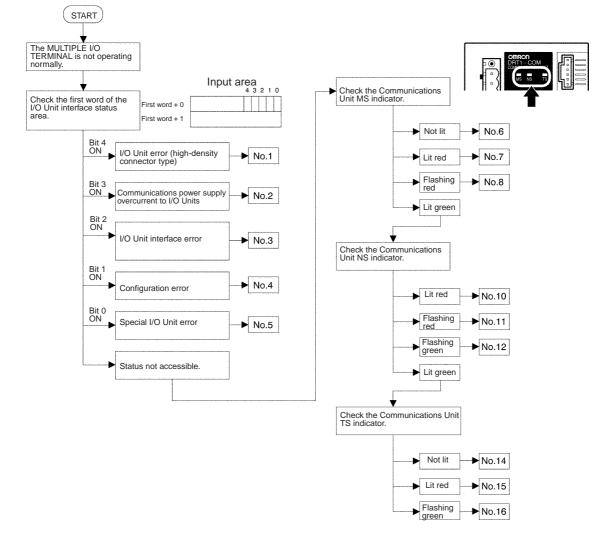
Status Area Error Processing A MULTIPLE I/O TERMINAL status area is available in the first two words of the MULTIPLE I/O TERMINAL input area in the Master. The contents and causes of errors can be found by checking this area.
