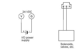
**Note** V terminals and V connector pins, as well as G terminals and G connector pins, are internally connected. When the I/O power is being supplied from a terminal block, the power can be supplied to the output devices from the V and G connectors. Current supplied in this way, however, must be less than 2 A.
