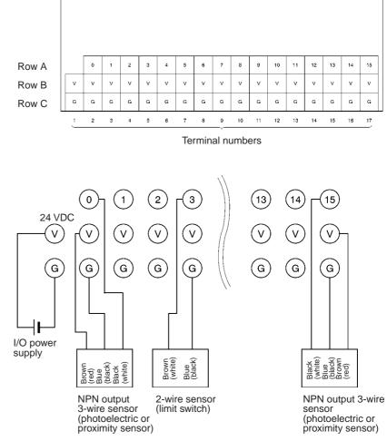
Wire colors in parentheses are the previous JIS colors for photoelectric and proximity sensors.
