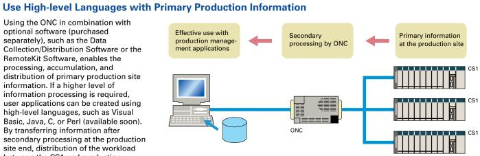
between the CS1 and production management system and links to the production management database enable a smooth flow of information.
