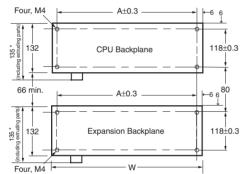
\* The CS1D Backplane does not have any extruding parts.
