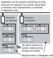
enables easy removal from network or changes to connections.
