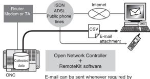
E-mail can be sent whenever required by installing a single ONC in the facility (e.g., gas turbine power generation plants).
