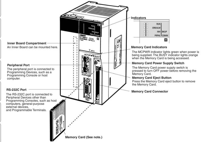
With the CS1 PLCs, Memory Cards and specified ranges of the EM Area can be used as file memory. File memory can be used to store the entire user program, I/O memory contents, and/or parameter area contents.
