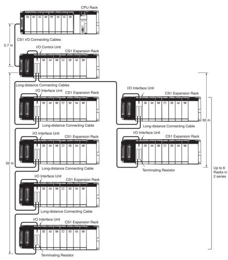
Note: C200H Units cannot be mounted to Long-distance Expansion Racks. (They can be mounted to the CS1 Expansion Rack with the I/O Control Unit mounted.)
