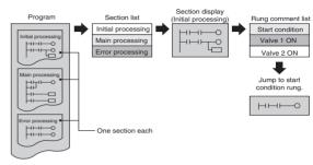
It is possible to jump to a specified section while viewing the overall program in a section list.
