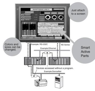
A SYSMAC CS/CJ-series PLC's Ladder Program can be monitored from an NSseries Programmable Terminal after the System is started.
