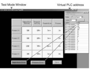
The test function enables debugging screens without NS and PLC Hardware.
