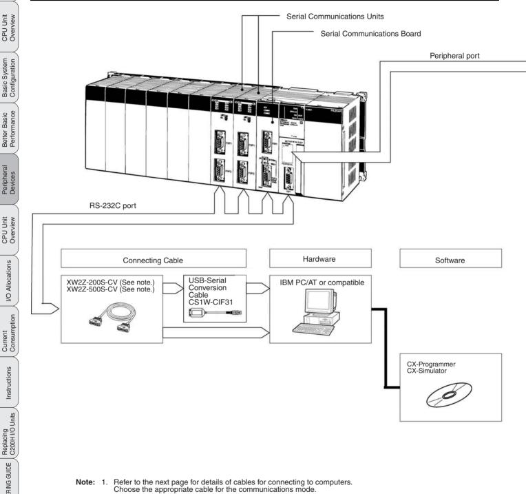
2. The following cables can be used for a Host Link connection (but not a peripheral bus connection): XW2Z-200S-V XW2Z-500S-V
