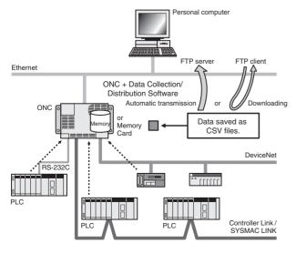
Example: Data collected using the Data Collection/Distribution Software can be displayed in Excel as shown below. A sample CSV file is shown set to collect data when bit 00 in CIO 0000 turns ON. The date can be added each time data is collected, and field names can be attached.
