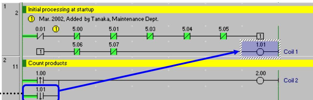
(6)The focus moves to the coil 1.01. As it turned out, the cause was the contact 0.01 that was not turned on.
