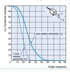
F3UV-XA + F3UV-HM + F32-300 (output characteristics at 300 mW/cm² when sensitivity is set)
