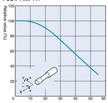
$\begin{array}{c} \text{Angle (degrees)} \\ \text{Note: X-direction output fluctuation is } \pm 10\% \text{ F.S.} \\ \text{or less through } 360^{\circ} \text{ revolution} \end{array}$
