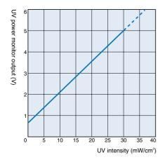
F3UV-A03 (output characteristics when output at 3 mW/cm² is set to 5 V)
