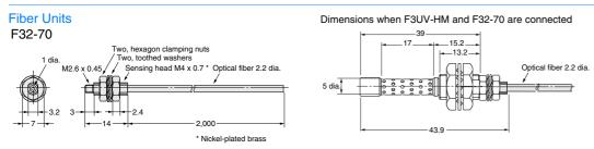
Note: free-cutting is possible. Free-cutting is not possible on units that are not marked with
