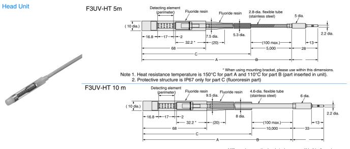
\* When using mounting bracket, please use within this dimensions Note 1. Heat resistance temperature is 150°C for part A and 110°C for part B (part inserted in unit). 2. Protective structure is IP67 only for part C (fluororesin part)
