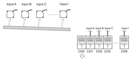
The operation and/or measurement results are output as judgement output or linear output.
