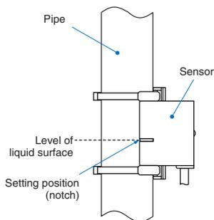
2. After Sensor installation adjust the detecting sensitivity using the (12-step) sensitivity adjuster in the way shown below.
