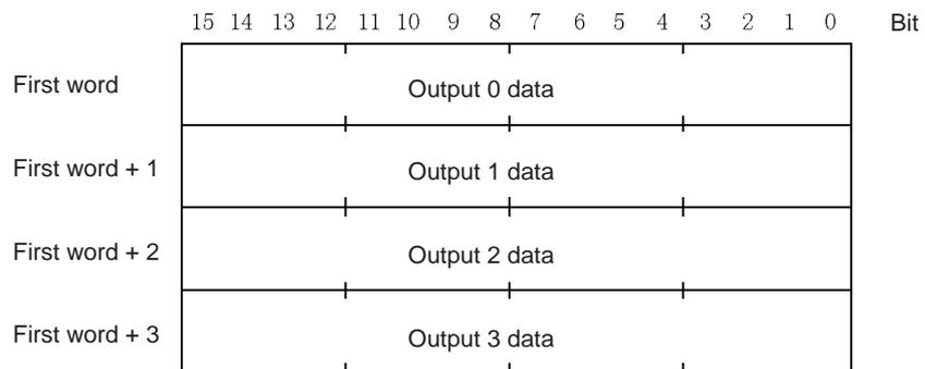
When a negative voltage is to be output, specify the conversion data as the two's complement. To obtain a two's complement from an absolute value, the NEG instruction is useful.
