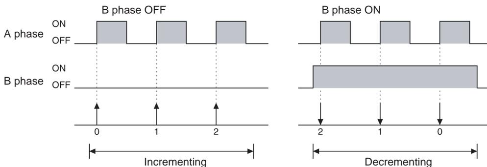
**Note** Switching B phase (direction input) ON and OFF, must be carried out with A phase (pulse input) switched OFF.
