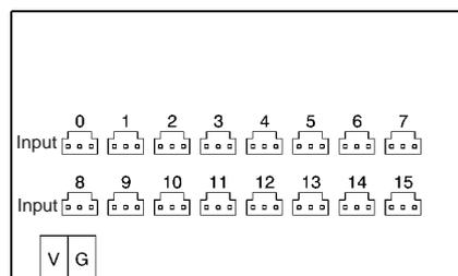
**Connector Pin Arrangement**
