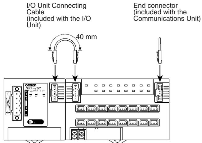
Connect the I/O Units in order, in the way shown in the above diagram. A maximum of 8 Units can be connected.
