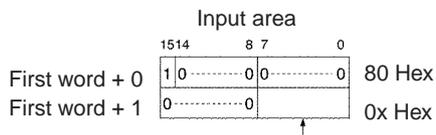
Bits corresponding to the addresses of I/O Units that are actually connected will be turned ON (1). Bits 0 to 7 correspond to addresses 0 to 7.
