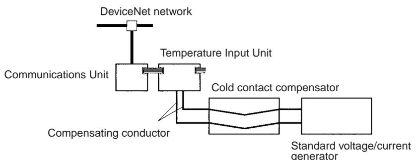
Use a calibrated thermocouple in the cold junction compensator and a compensating conductor, and set the cold junction compensator to 0°C.
