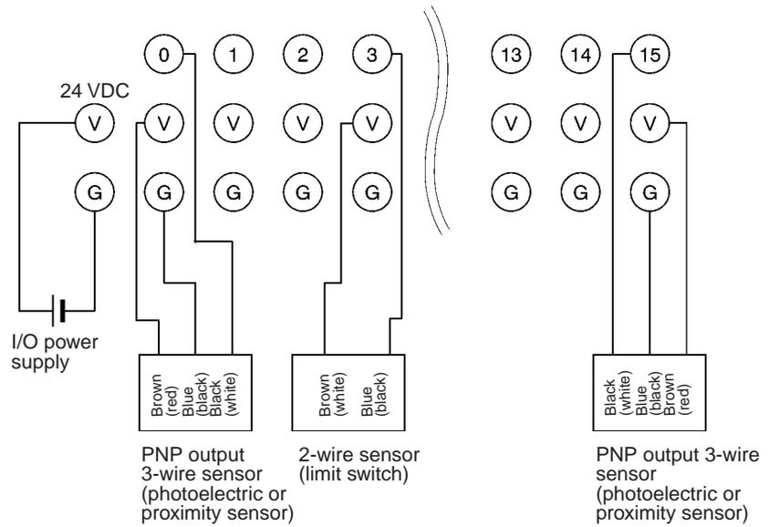
Wire colors in parentheses are the previous JIS colors for photoelectric and proximity sensors.
