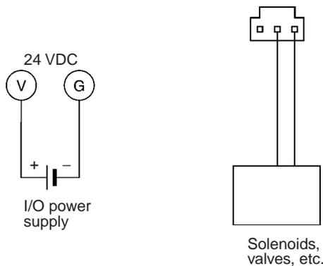
**Note** V terminals and V connector pins, as well as G terminals and G connector pins, are internally connected. When the I/O power is being supplied from a terminal block, the power can be supplied to the output devices from the V and G connectors. Current supplied in this way, however, must be less than 2 A.
