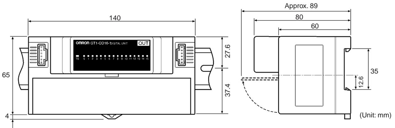
**Note** The vertical center of the Unit is 4.9 mm lower than the center of the DIN track. The Unit therefore extends downward 41.4 mm (including the mounting hook) from the DIN track center.
