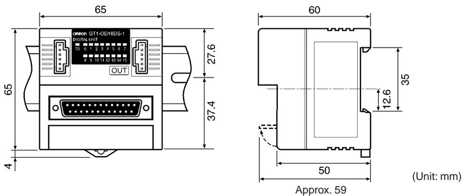
**Note** The vertical center of the Unit is 4.9 mm lower than the center of the DIN track. The Unit therefore extends downward 41.4 mm (including the mounting hook) from the DIN track center.
