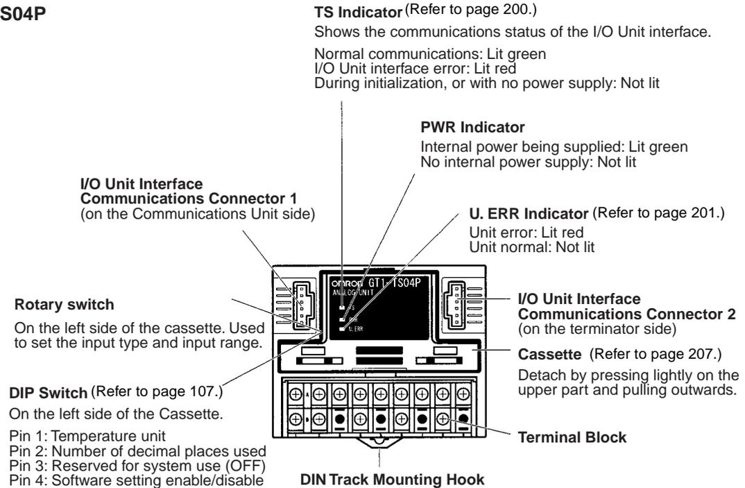
**DIP Switch and Rotary Switch Settings**
