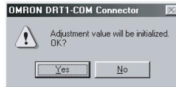
The calibration data stored in the EEPROM in the Temperature Input Unit will be cleared.
