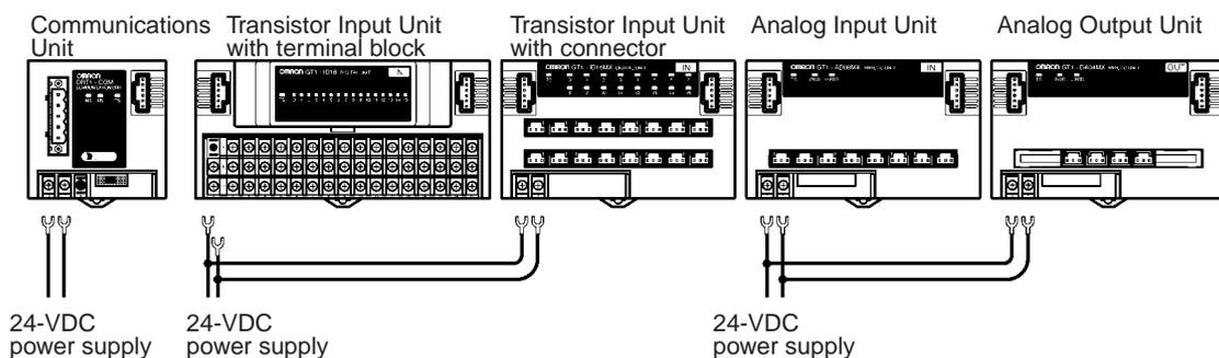
Note Be sure to separate the communications power supply, the internal power supply for the Communications Unit and the CPU Bus Unit, and the power supplies for the I/O Units. If the same power supply is used, malfunction due to noise may occur.
