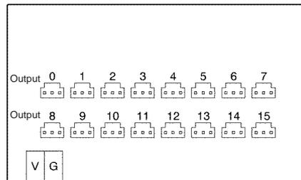
Connector Pin Arrangement
