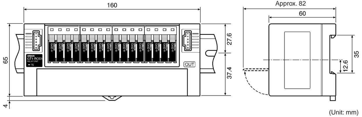
**Note** The vertical center of the Unit is 4.9 mm lower than the center of the DIN track. The Unit therefore extends downward 41.4 mm (including the mounting hook) from the DIN track center.
