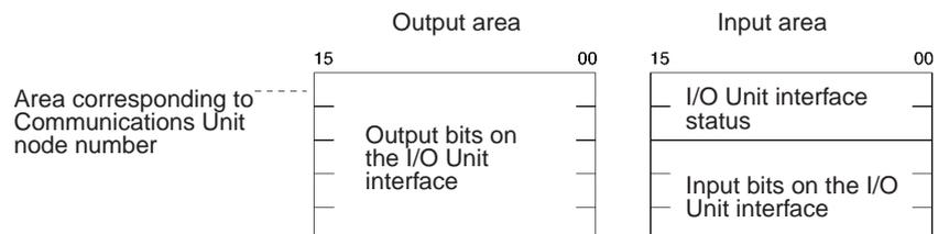
The input and output bits for the I/O Unit interface are allocated in the DeviceNet input and output areas in 16-point (one word) increments. With 8-point I/O Units, these bits are allocated using the rightmost byte (bits 0 to 7), and the leftmost byte (bits 8 to 15) will be 00 Hex.
