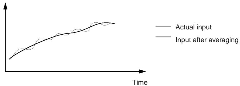
**Note** The time required for refreshing converted data remains one ms/point when the averaging function is enabled. The first communications data after the power is turned ON will be output after averaging eight samples.
