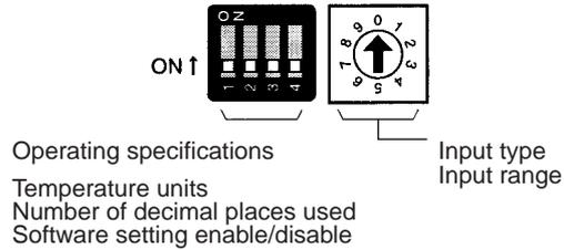
**Note** Before detaching or attaching the Cassette or making DIP switch or rotary switch settings, be sure that the power supply to the I/O Unit (including power supply to I/O Unit interface) is OFF.
