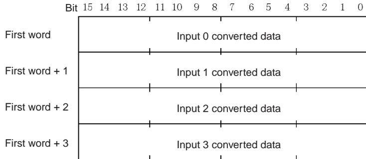
If the converted data is a negative number, it is stored as a two's complement. Data for range codes that include one digit after the decimal point are stored without the decimal point, i.e., 10 times the actual value is stored. Some examples are provided in the following table.
