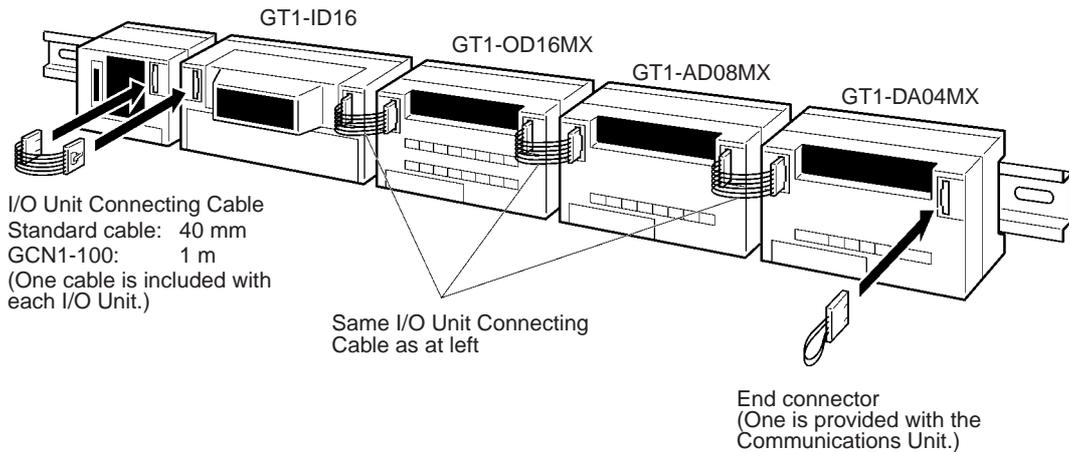
To connect each pair of Units, connect I/O Unit interface communications connector 2 on the Unit closer to the Communications Unit to I/O Unit interface communications connector 1 on the Unit closer to the end Unit.
