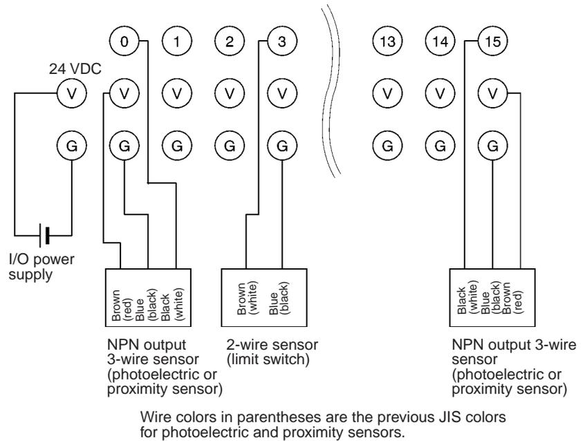
**Note** V terminals and G terminals are internally connected. When the I/O power is being supplied, the power can be supplied to the input devices from the V terminals and G terminals. Current supplied in this way, however, must be less than 1 A.
