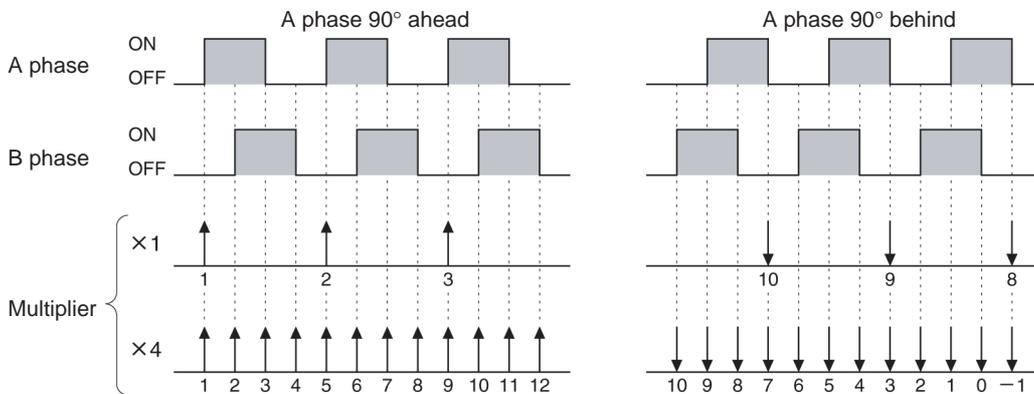
**Note** When using differential phase pulse input at a multiple function setting of ×4, the count number for each revolution of the encoder will be 4 times the resolution of the encoder. Use an encoder that is compatible with the counting range.
