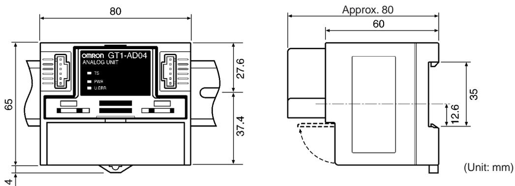
**Note** The vertical center of the Unit is 4.9 mm lower than the center of the DIN track. The Unit therefore extends downward 41.4 mm (including the mounting hook) from the DIN track center.
