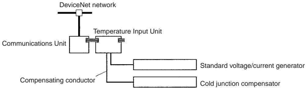
Use a calibrated thermocouple in a cold junction compensator and a compensating conductor. If using an R, S, or B thermocouple, a K thermocouple can be used instead. Set the cold junction compensator to 0°C, but disable the setting (i.e., keep the contact open) until the bias compensation described in step 10 is completed. Do not touch the Temperature Input Terminal or the compensating conductors.
