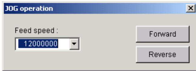
Select a speed in Reference Units per Minute and select Forward or Reverse. The servo should rotate at the speed set in the Feed Speed input box.
