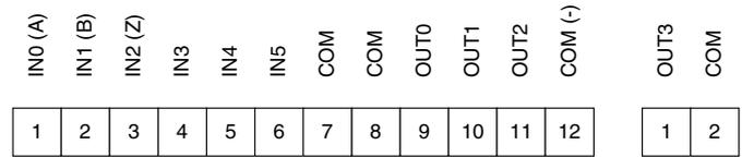
Connector: WAGO 733-112 (wire cross section 0.08 to 0.50 mm<sup>2</sup>)
