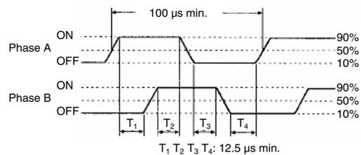
The minimum pulse width for input IN00002 (Z-phase input) is as follows:
