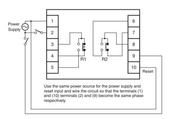
Note: The R2 relay can be switched between instantaneous and time-limit contacts and thus the contact symbol is shown as follows: 🚉
