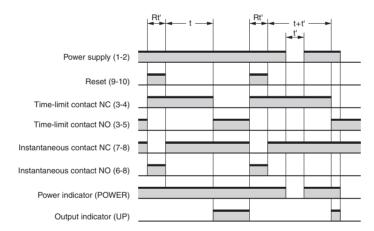
**Note:** t is the set time, Rt' is the reset application time, and t' is the power interruption time.
