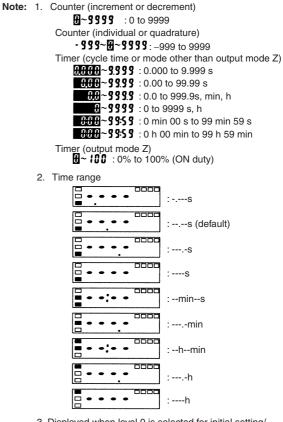
3. Displayed when level 0 is selected for initial setting/communications protection in the protect level.
