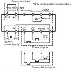
Note: (2) and (6) are connected internally.
