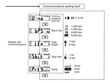
**Note:** Settings made in the communications setting level are enabled when the power is turned ON again.
