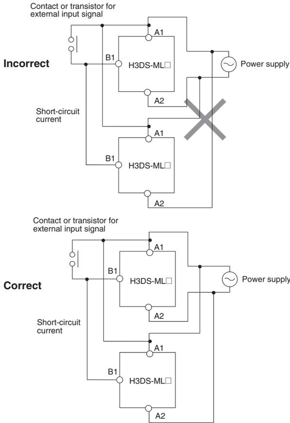
The H3DS Series is provided with a transformerless power supply system.
