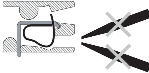
Do not move the screwdriver side to side in the clamp hole. The clamp spring may be deformed if the screwdriver is moved sideways.
