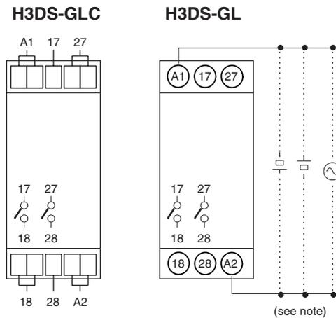
**Note:** DC supply voltage does not require the designation of polarity.
