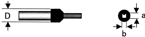
**Note: 1.** If the overall diameter of the wire is less than 1.8 mm, do not insert the wire past the conductor. Refer to the following diagrams.
