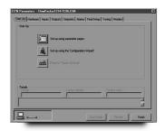
ThermoTools is equipped with extended help functionality, that covers everything from getting started to becoming familiar with the advanced functionality. The 'configuration wizard' can be used to configure controllers for 'basic' applications. The wizard will ask you a sequence of questions about the type of controller set up that you require based on the most commonly used parameters. This allows you to create a quick and easy set up.
