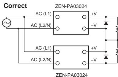
**Note:** When the load is an operational amplifier or other device allowing series operation, a startup failure may occur when the Power Supply is turned ON and internal circuits may be damaged. Connect a diode as shown in the figure to prevent this.
