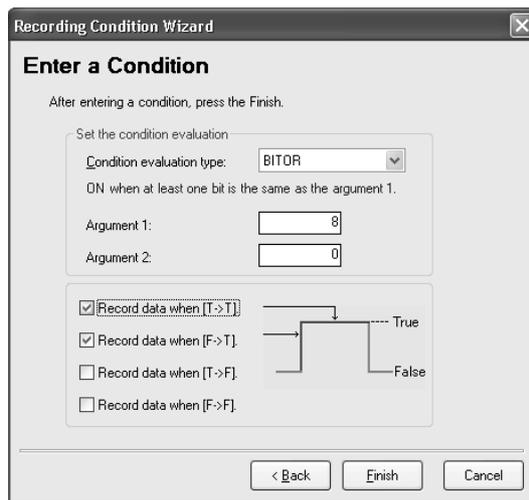
**Note** (1) Evaluations are calculated based on the word contents of the address specified for the variable, not on the converted value for the data type of the variable.
