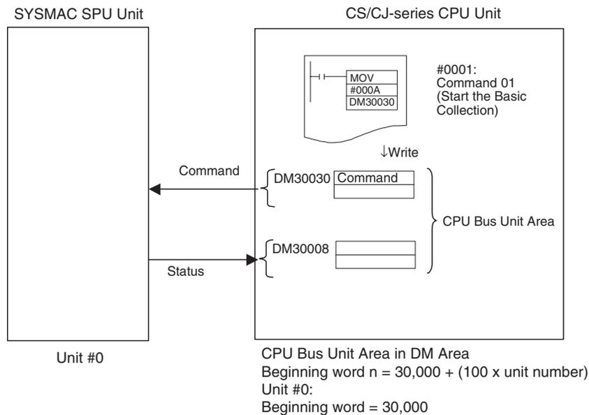
This method can be used, for example, to start and stop data collection from the ladder program in the CPU Unit.
