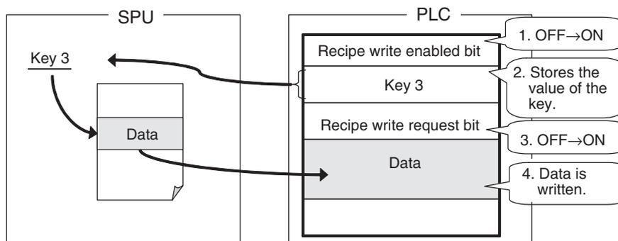
The memory area where the value of the key is stored can be set in Key Area of the environment settings.
