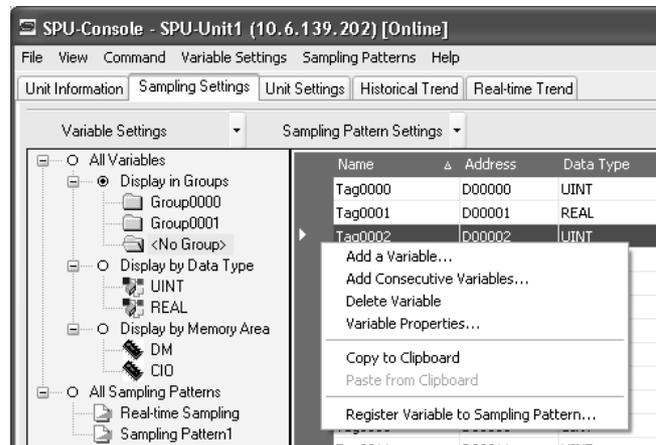
4. Enter the new settings in the Variable Properties Dialog Box and click the **OK** Button. For details on these operations, refer to *17-3-2 Operations in the Variable Properties Dialog Box*.
