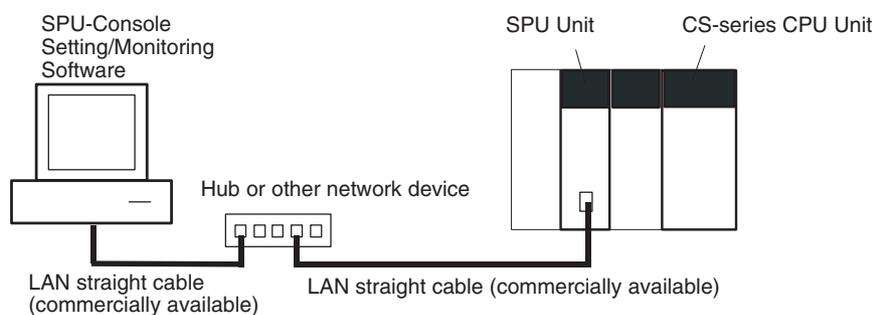
**Note** Do not connect to the network more than one SYSMAC SPU Unit for which initial settings have not been made. IP addresses will be duplicated, and communications may not be possible. Disconnect the LAN cable from all SYSMAC SPU Units except for one and set one SYSMAC SPU Unit at a time.
