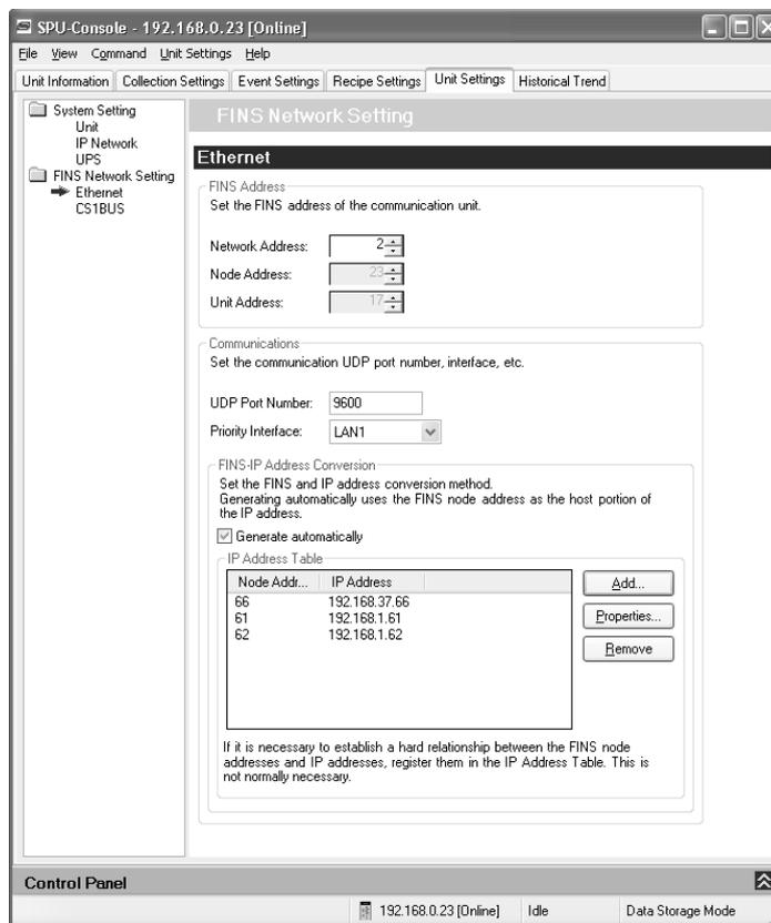
**Note** Set the same Ethernet network address for the FinsGateway on the computer and in the SYSMAC SPU Unit.
