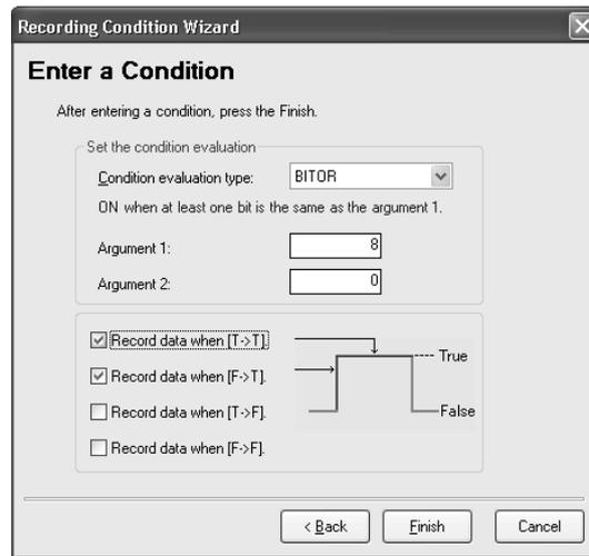
**Note** Evaluations are calculated based on the word contents of the address specified for the variable, not on the converted value for the data type of the variable.
