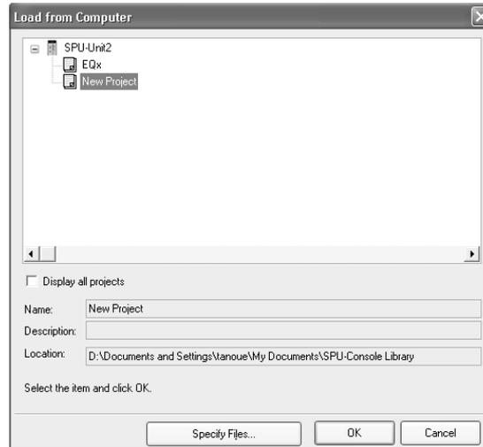
2. In the Load from Computer Dialog Box, select the project to be read and click the **OK** Button. If *Display all projects* is selected, all of the projects managed by the Project Explorer will be displayed. Select this checkbox when reading projects of other SYSMAC SPU Units.
