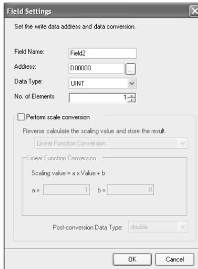
2. Set the field parameters in the Field Settings Dialog Box. The following table describes the field parameters.
