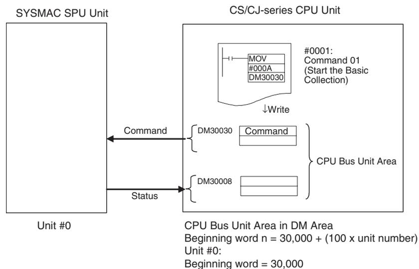
For example, SYSMAC SPU Unit commands can be used to specify operations such as starting and stopping data collection.
