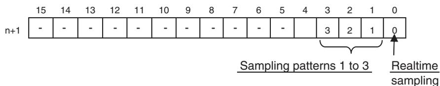
**Collection Start Specification, Collection Stop Specification, Collection Request (CPU Unit to SPU Unit)**
