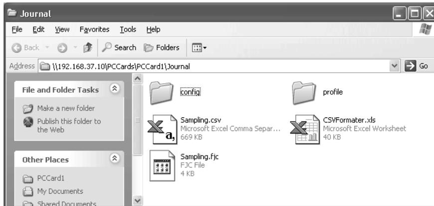
2. Double-click the sampling file that is to be displayed. Excel will be started and the contents of the sampling file will be displayed. If the CSV file extension is associated with an application other than Excel, the associated application will be started.
