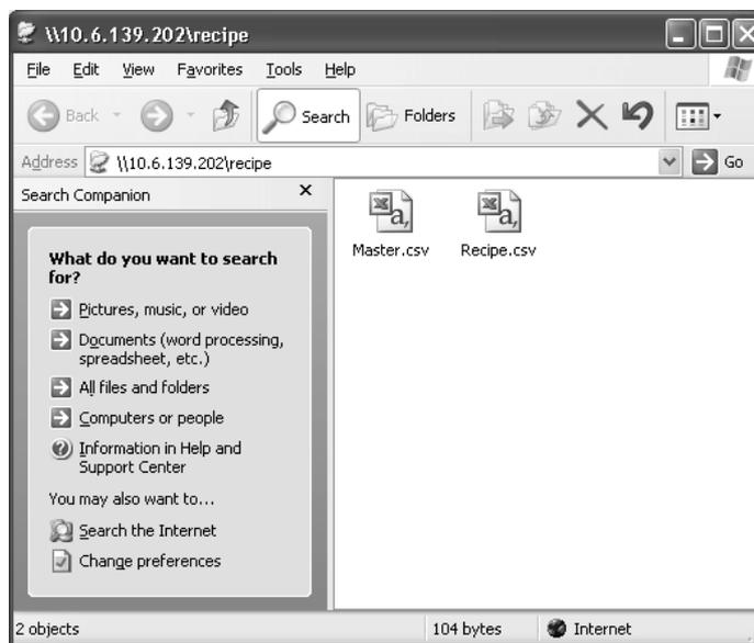
The method to access the recipe folder in the SYSMAC SPU using a computer is described below.
