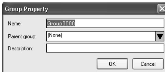
2. Add the group's name in the Name Field. In the *Parent group* Field, select the group to be the parent of the group level. (This does not need to be specified.) A description of the group can be entered in the *Description* Field. (This entry can be omitted.)
