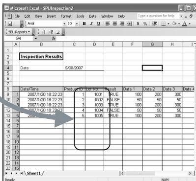
Multiple records will be displayed in cells downward from the specified cell.
