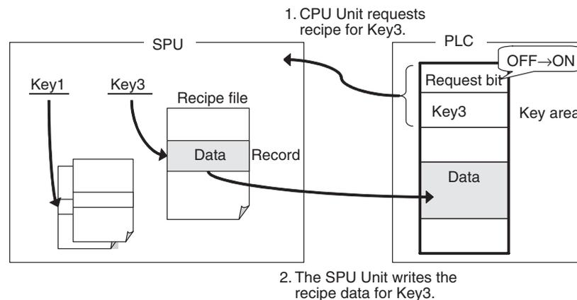
Recipe data is internally managed in the following structure. Each recipe is characterized by a recipe file and a record. In the example shown in the following figure, recipe data for Key3 is record 3 of the recipe file Data\_A.csv.
