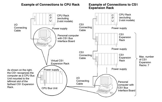
**Note** 1. Connect the computer to the last CS1 Expansion Rack.
