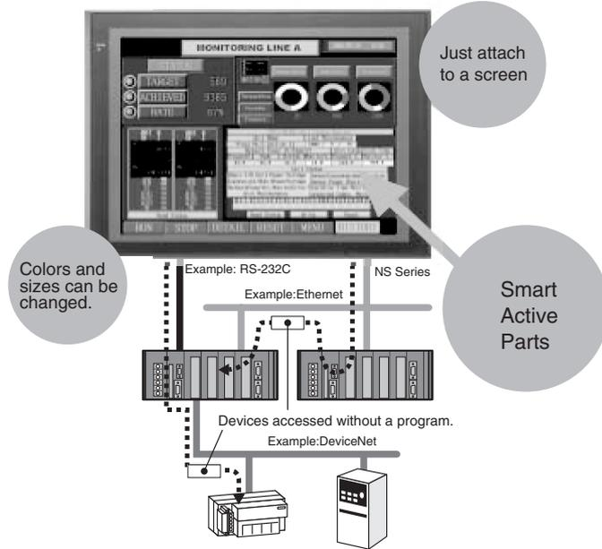
**A SYSMAC CS/CJ-series PLC's Ladder Program can be monitored from an NS-series Programmable Terminal after the System is started.**
