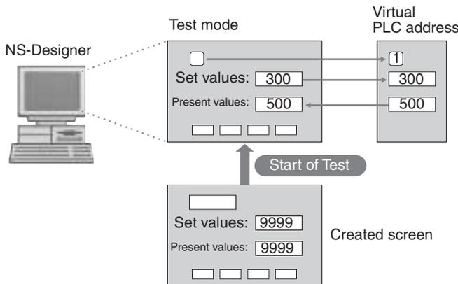
Operating (clicking with the mouse) the functional objects on the test screen will change the corresponding address in the virtual PLC. Conversely, changing the content of a virtual PLC address will change the corresponding functional objects. It is also possible to confirm pop-up screens. This function can be used to confirm the actual operation of a screen during the edition.
