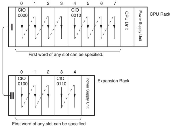
With CX-Programmer version 3.2, up 3 first slot words can be specified.
