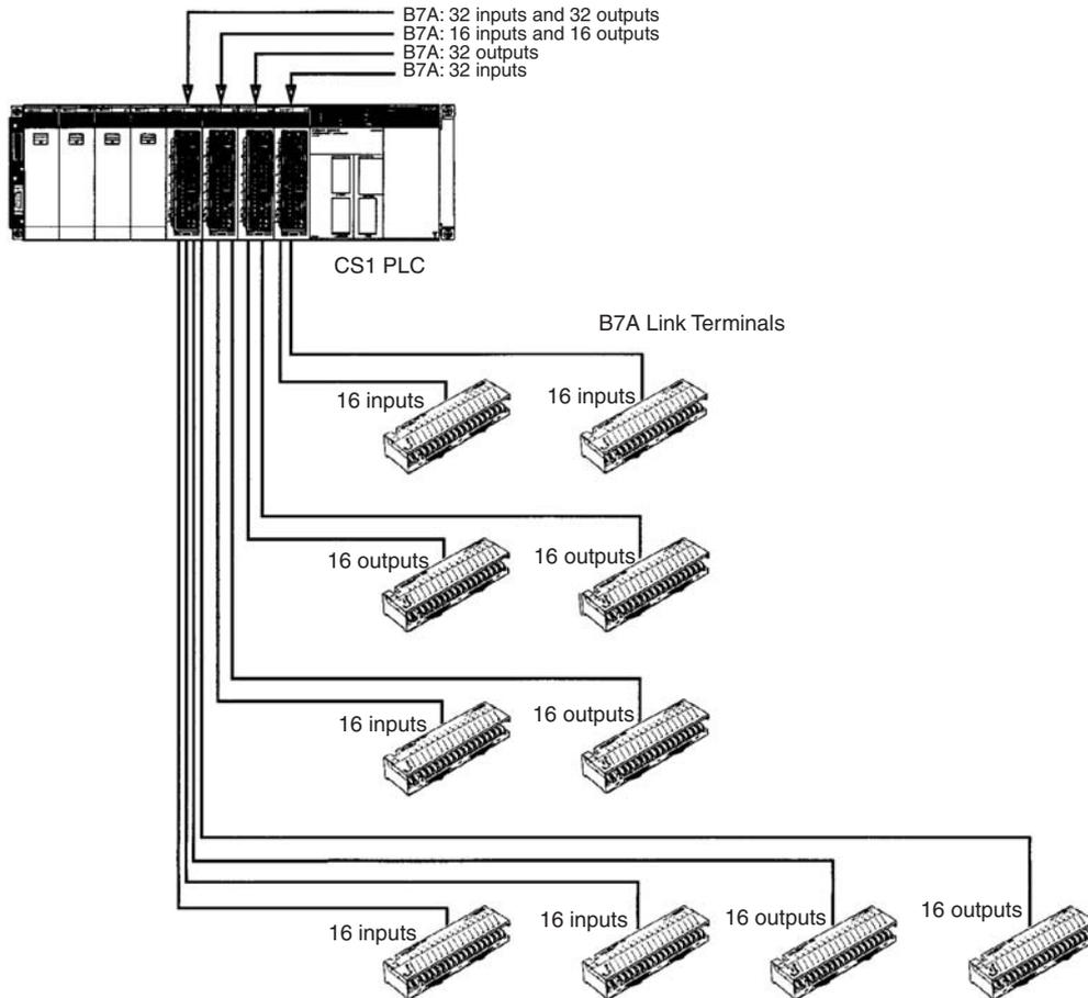
**Note:** Refer to the B7A Link Terminal catalog (Q101) for details on B7A Link Terminals.
