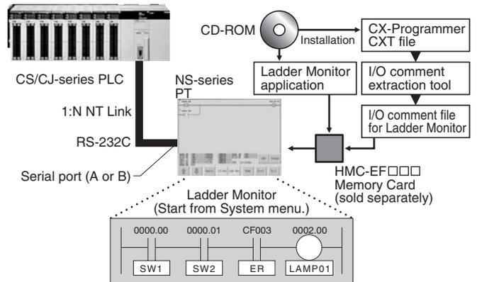
Note: The PLC operation can be monitored only if the PLC is a CS/CJ-series PLC connected to serial port A or serial port B of the Programmable Terminal with 1:N NT Link protocol.
