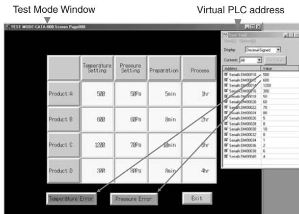
The test function enables debugging screens without NS and PLC Hardware.
