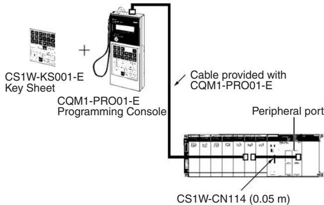
**Note:** The above configuration is also possible for the C200H-PRO27-E with a Programming Console Cable, such as the C200H-CN222.
