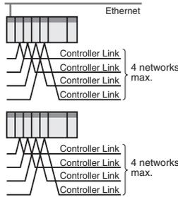
New CS/CJ-series Controller Link Units (Wired/Optical Ring) enable connection of up to 8 Controller Link Units for each CPU Unit. This enables easy centralized control of a group of Controller Link sub-networks from the one PLC.
