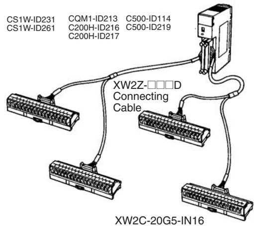
**■ XW2Z Connecting Cables for Connector-Terminal Block Conversion Units**
