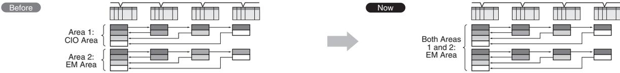
Area 1 and Area 2 had to be allocated in separate Memory Areas for user-set data links. Therefore, allocating all data links in the EM Area was not possible.
