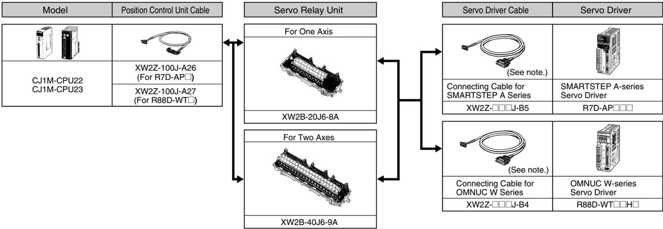
**Note:** When using the Unit for two axes, two Servo Driver Cables are required for each Servo Relay Unit.
