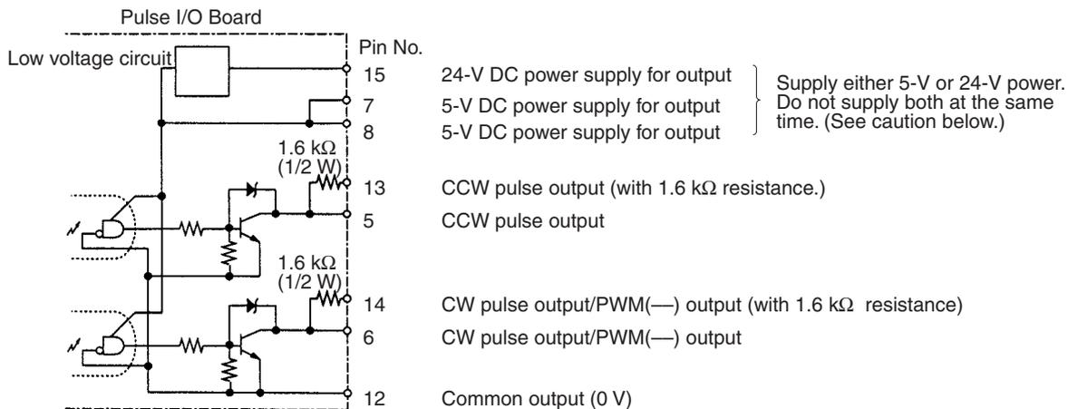
**Caution** Do not supply both 5-V and 24-V DC power at the same time. Doing so will damage the internal circuits.
