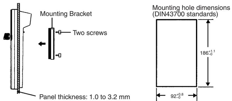
Allow at least 80 mm for the cable connector above the Programming Console.
