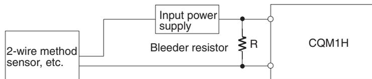
$$R = 7.2 / (2.4 I - 3) \text{ k}\Omega \text{ max.} \quad \begin{array}{l} I: \text{Device's leakage current (mA)} \\ R: \text{Bleeder resistance (k}\Omega\text{)} \end{array}$$
