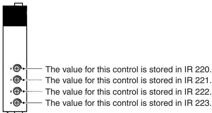
**⚠ Caution** While the power is turned ON, the contents of IR 220 to IR 223 are constantly refreshed with the values of the corresponding controls. Be sure that these words are not written to from the program or a Programming Device.
