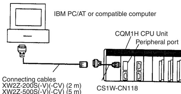
**Connecting to RS-232C Port using RS-232C Cable**
