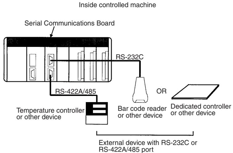
Both RS-232C and RS-422A/485 ports are provided. The RS-422A/485 port enables 1:N connections to general-purpose external devices without going through Converting Link Adapters. The 1:N connections can be used with protocol macros or 1:N-mode NT Links.
