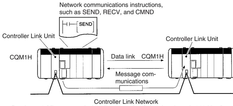
Baud rate: 2 Mbps; transmission distance: 1 km (when baud rate is 500 kbps); max. No. of nodes: 32.
