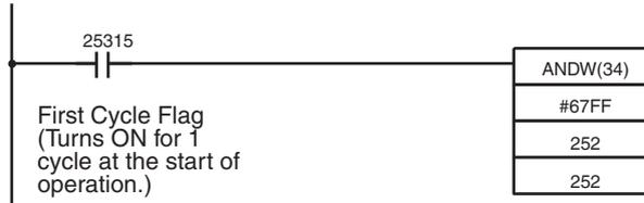
If the setting shown below is made in the PC Setup (DM 6655 bits 12 to 15), battery errors (a non-fatal error) will not be detected even if the internal battery expires.
