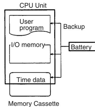
**Note** Do not remove the battery except when replacing it. If the battery is not replaced within 5 minutes after removal, internal data may be lost. For details on the replacement method, refer to *9-1 Battery Replacement*.
