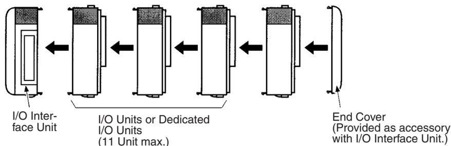
There is no Backplane for the CQM1H. The PC is constructed by connecting Units together using the connectors on the sides.
