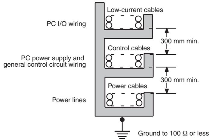
If the I/O wiring and power cables must be placed in the same duct, they must be shielded from each other using grounded steel sheet metal.
