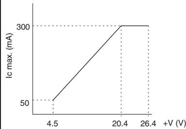
Max. Switch Capacity (Total for Unit)
