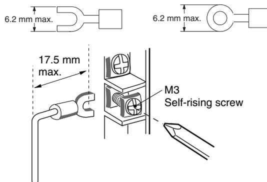
**Note** Tighten the terminal screws to a torque of 0.5 N·m.
