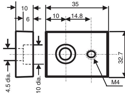
**DIN Track Insulation Spacer Mounting Method**
