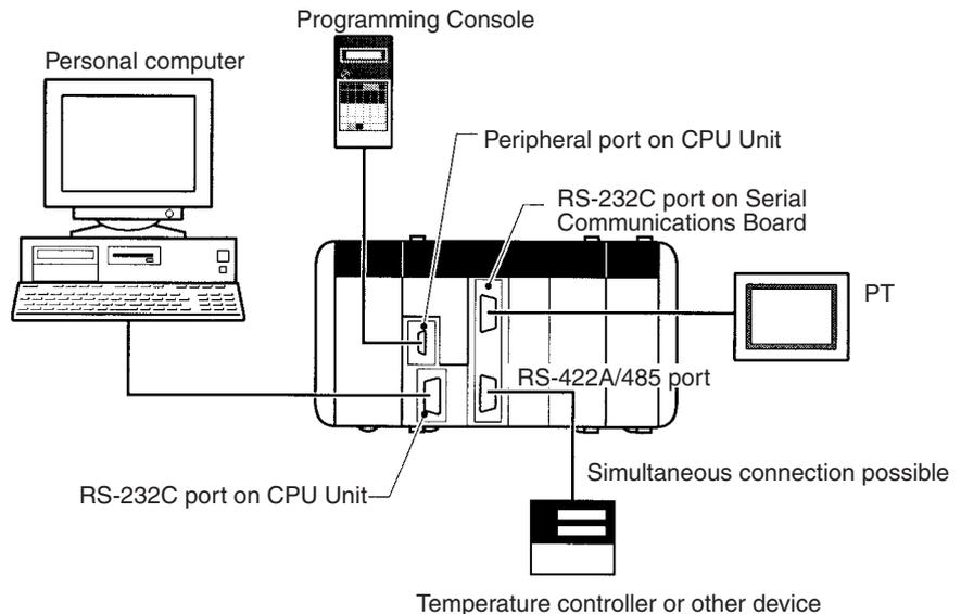
You can also program and monitor from a personal computer at a remote location via a modem. When used in combination with the protocol macro function, it is also possible to call the personal computer from the CQM1H using the PMCR(—) instruction, and when the connection is made, switch the serial communications mode to Host Link (for remote programming/monitoring) using the STUP(—) instruction.
