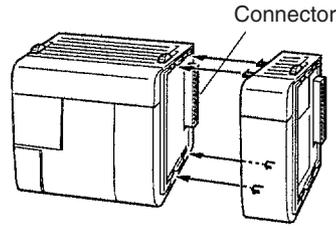
2. The yellow locking tabs at the top and bottom of each Unit lock the Units together. Slide these locking tabs towards the back of the Units as shown below until they click into place.
