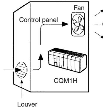
The ambient temperature range in which the CQM1H can be used is 0 to 55°C (0 to 45°C if a Programming Console is connected to the CPU Unit).
