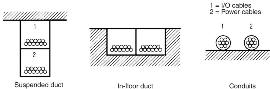
If the I/O wiring and power wiring must be routed in the same duct, use shielded cable and connect the shield to the GR terminal to reduce noise.
