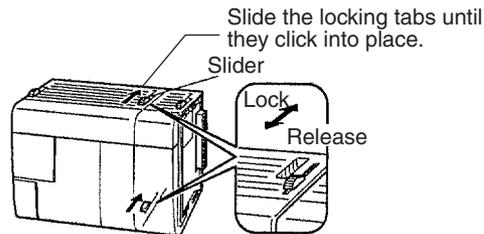
3. Attach the End Cover to the Unit on the far right side of the PC.
