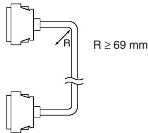
**Note** Place the Expansion I/O Cable into a separate duct from power lines and I/O lines to protect it from noise.
