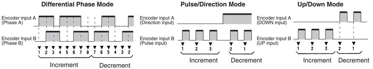
**Note** The function of encoder inputs A and B in Pulse/Direction Mode and Up/Down Mode differs from the High-speed Counter Board (CQM1H-CTB41).
