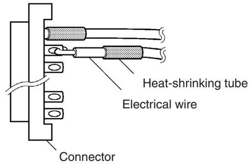
After soldering all of the necessary pins, slide the heat-shrinking tubes over the soldered areas of the respective wires. Then shrink the tubes by heating them with a jet of hot air.
