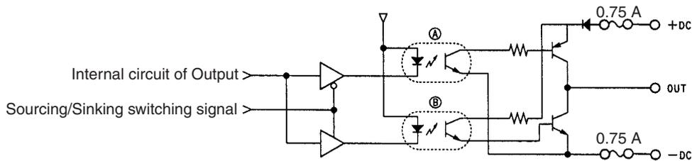
**Note** In the above figure, A is active when sourcing outputs are set, and B is active when sinking outputs are set.
