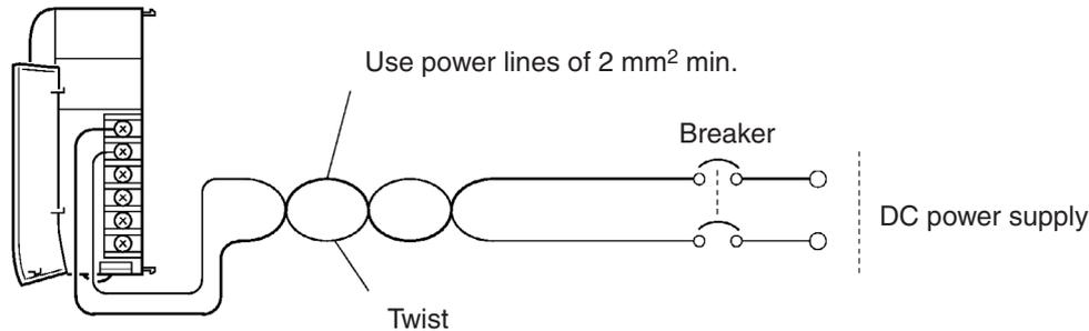
**Caution** Be sure that the DC power supply voltage remains within the allowed fluctuation range of 20 to 28 V DC.
