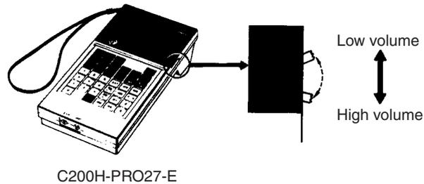
**Note** The buzzer can be turned ON and OFF with a key operation. See 7-3-4 *Buzzer Operation* for details.
