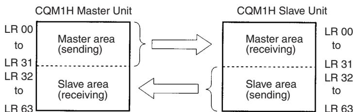
This mode is supported by the RS-232C port on the CPU Unit, as well as the RS-232C port and RS-422A/485 port on the Serial Communications Board.
