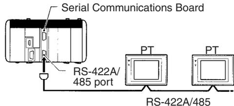
**Note** The 1:1 NT Link mode and 1:N NT Link mode use different types of serial communications and there is no data compatibility between them.
