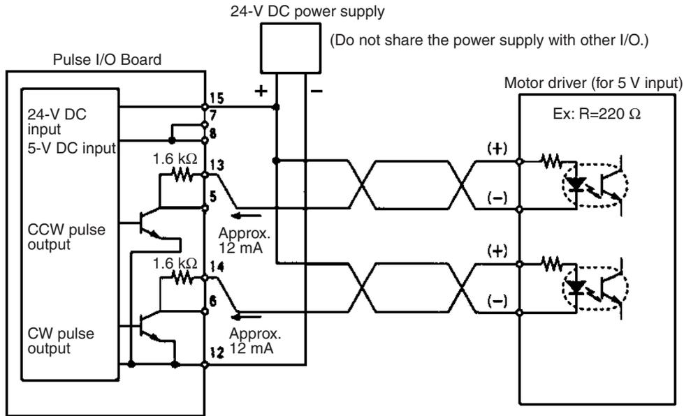
**Note** Here, a 5-V input motor driver is being used with a 24-V power supply. The internal resistance at the Pulse I/O Board (1.6 kΩ) is thus used. Care must be taken to avoid problems caused by the drive current at the motor driver.
