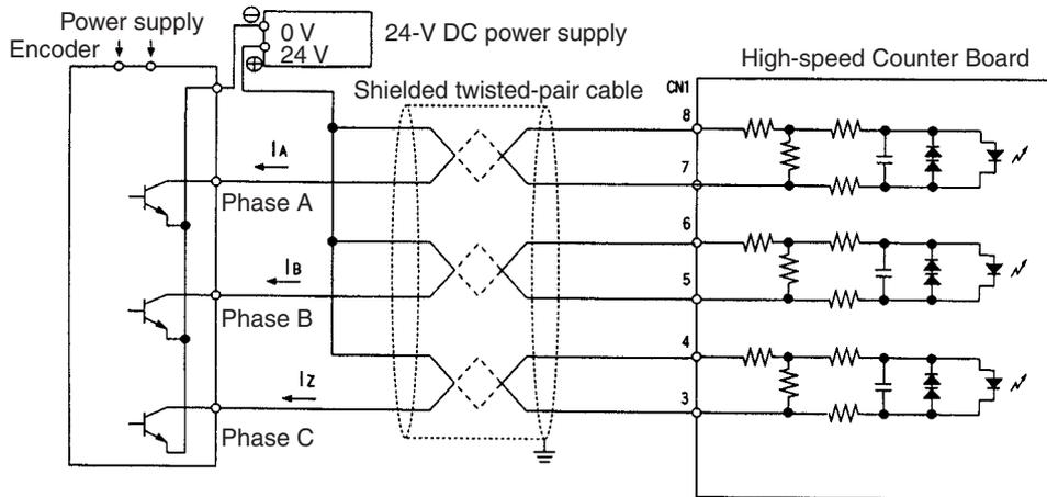
Connecting to an Encoder with a Line-driver Output (Am26LS31)
