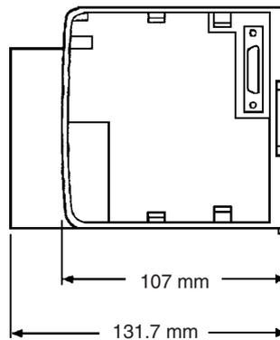
**Note** The depth of connector-type I/O Units is approx. 120 mm when pressure-welded connectors are used.
