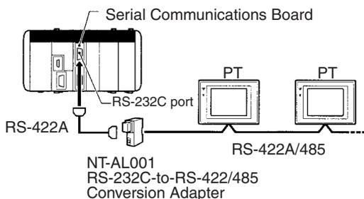
Connection to RS-422A/485 port of Serial Communications Board
