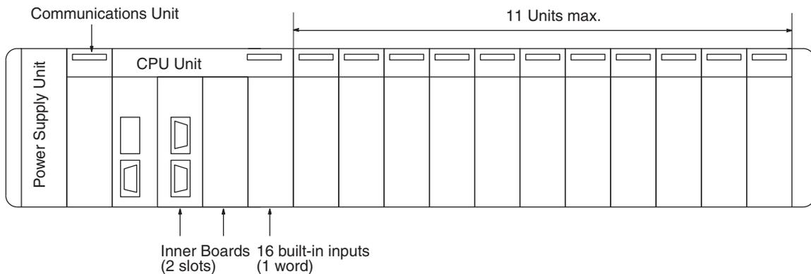
CPU Block and Expansion I/O Block
