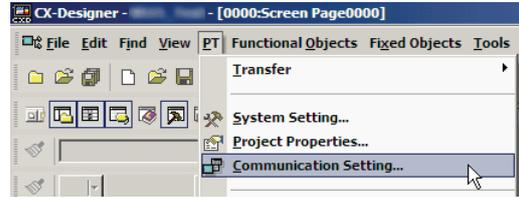
2) **Comm. Setting** Dialog Box will be displayed. Click **Serial Port A** or **Serial Port B** depending on the port you want to connect S7-300 series PLC, and configure it on right-side pane.
