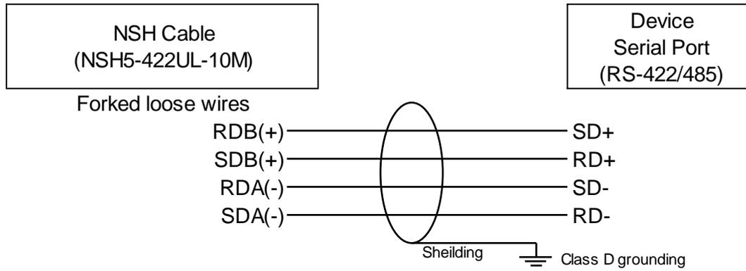
**Connection Diagram 3 (NS-series PTs excluding NSH-series PTs with RS-485 (two-wire method) connection)**
