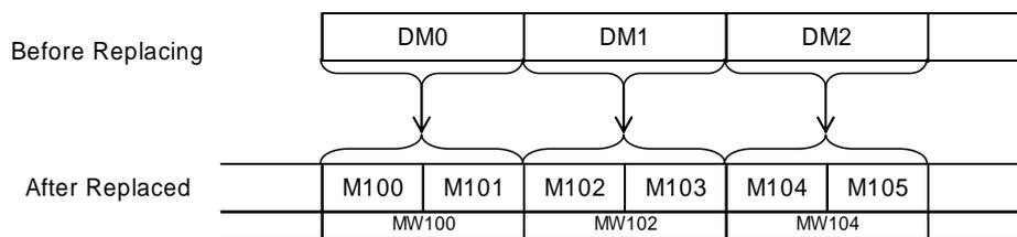
For another example, when SERIALB:MW0 to MW5 are replaced with SERIALA:D100, each MW0, MW2 and MW4 will be replaced with DM100, D101 and D102. However MW1, MW3 and MW5 will not be replaced since they do not have corresponding addresses.
