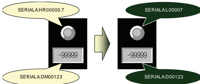
"—" in the right table means those addresses cannot be mapped to new PLC's address, so they will not be changed. This may cause invalid addresses (see the figure below), so you have to modify such invalid addresses by yourself. Refer to 1-3-1 Notes and Restrictions When Changing Host Type for how to find and modify them.
