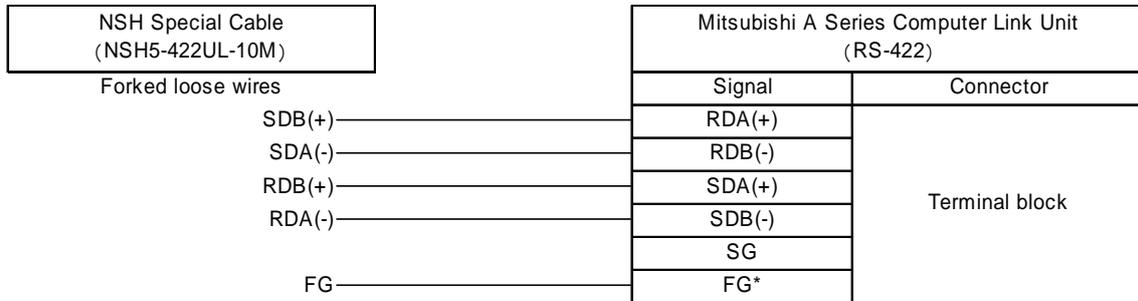
\* Connect to FG which is class D grounded.
