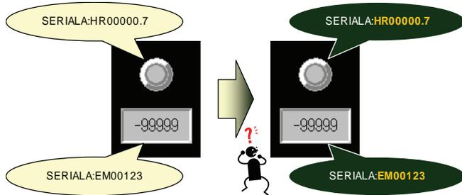
Note: Address numbers will be changed to make their bit offsets equal. For example, CIO00003.12 is the 60th bit ( $60=16 \times 3 + 12$ ) of CIO, so will be converted to M00007.4 ( $60=7 \times 8 + 4$ ).
