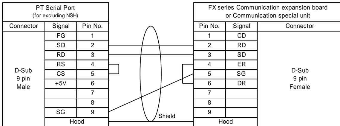
OMRON XW2Z-S002 (2m long) cable is also applicable. Even cable connection of XW2Z-S002 is not same as the connection diagram above, it is applicable because both NS and FX do not check control signals.
