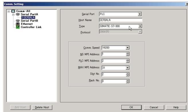
Set **Serial Port** to **PLC**, **Type** to **SIMATIC S7-300**, and **Protocol** to **3964(R)**. Configure other settings according to your environment.
