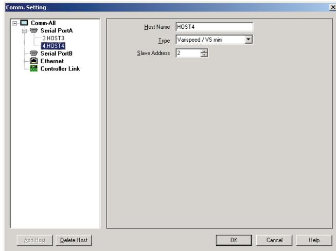
8) Click the **Serial PortA**. Then set **Comm.Speed**, **Stop Bits** and **Parity** in the left pane.
