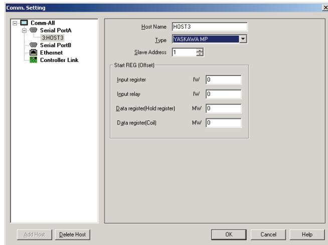
6) When connecting multiple inverters to a single serial port, click either the **Serial PortA** or **Serial PortB** in the left pane. Then click **Add**.
