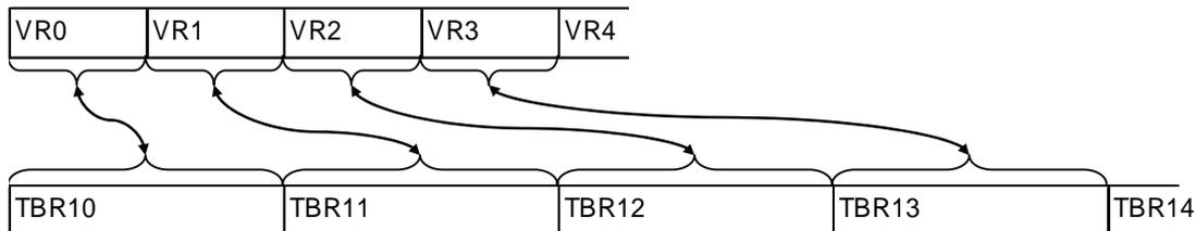
Example: Replacing VR0-VR3 with TBR10- and vice versa.
