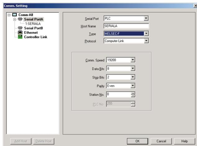
When you use a PLC other than Mitsubishi FX Series, necessary setting items will be displayed in accordance with the PLC type. For details on settings, refer to each PLC chapter.
