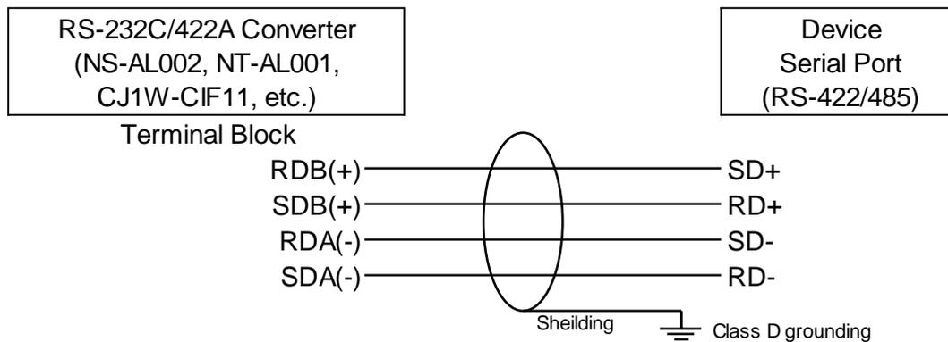
Set as shown on the table for the DIP Switches of the RS-232C/422A Converter.
