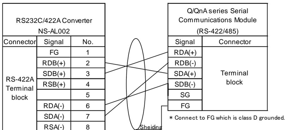
If the functional ground (FG) of the PT cannot be grounded for some reason, the shielding wire needs to be connected to the FG of NS-AL002.
