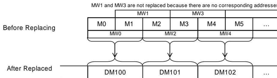
For another example, when SERIALB:MW5 to MW9 are replaced with SERIALA:D100, each MW5, MW7 and MW9 will be replaced with DM100, D101 and D102. However MW6 and MW8 will not be replaced.
