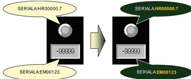
Note: Address numbers will be changed to make their bit offsets equal. For example, AR00003.12 is the 60th bit ( $60=16 \times 3 + 12$ ), so will be changed to AR00005 of SYSMAC, and S00084 to AR00005.4.
