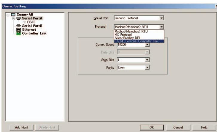
6) This screen is displayed. Confirm the Host Type is set to **Yokogawa FA-M3/FA-M3R**. Set the station number and CPU number so that they can match the settings for your personal link unit or CPU.
