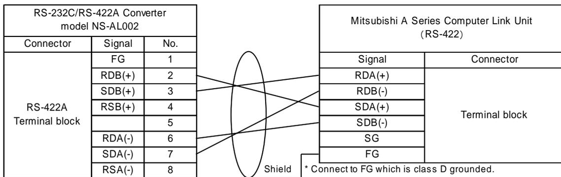
Note: If NS cannot be grounded for some reason, shield wire also needs to be connected to FG of NS-AL002.
