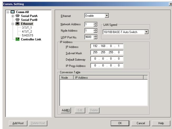
Set the IP address and Sub-net Mask according to the Ethernet environment used.
