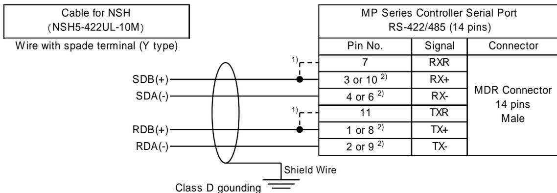
1) Connect them to enable the built-in terminal resistance of MP series.
