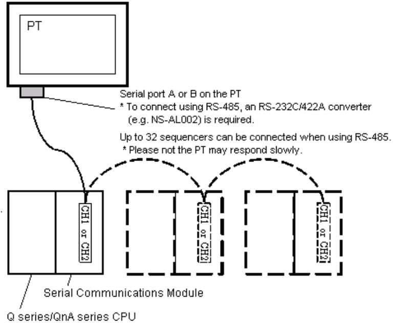
When using Q00CPU or Q01CPU, it is also possible to connect to the serial port on the CPU. In this case, use a Mitsubishi connection cable QC30R2 and conversion cable and wire them as illustrated on the right. For information on connection diagram, refer to 8-3 Communication Cables.
