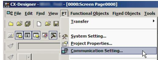
2) **Comm. Setting** Dialog Box will be displayed. Click **Serial Port A** or **Serial Port B** which you want to connect FX series sequencer, and configure it on right-side pane. Set **Serial Port** to **PLC**, **Type** to **MELSEC-F**, and **Protocol** to **Computer Link**. For other settings, refer to 3-2-2 Communication
