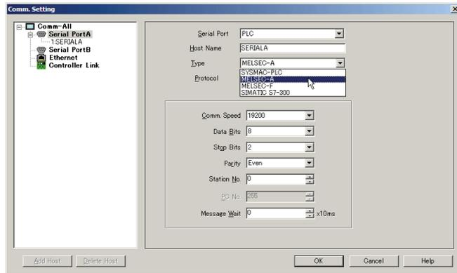
Set **Serial Port** to **PLC**, **Type** to **MELSEC-A**, and **Protocol** to **Computer Link**. The
