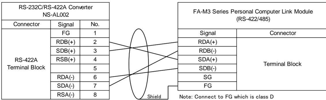
**Note:** If the PT cannot be grounded for some reason, shield wire also needs to be connected to FG of the NS-AL002.
