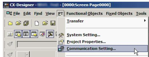
2) **Comm. Setting** Dialog Box will be displayed. Click **Serial Port A** or **Serial Port B** which you want to connect A series sequencer, and configure it in right-side pane.
