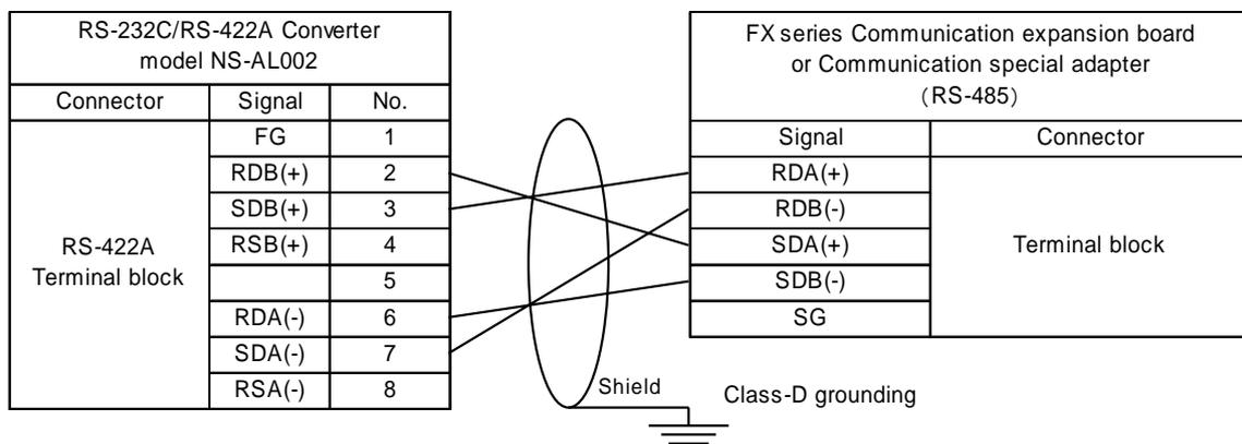
If NS cannot be grounded for some reason, shield wire also needs to be connected to FG of NS-AL002.
