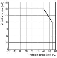
**Note:** The value for standard mounting. Note that the derating curve differs depending on the mounting.
