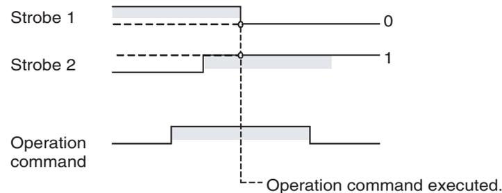
**Note** Software resets are executed again even if the strobe has not been cleared. Therefore the Output Enable Bit or the strobe must be cleared after the software reset command has been sent.
