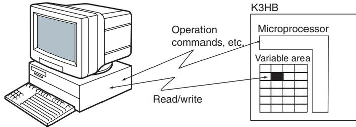
A variable area is accessed by specifying the position of a variable within the variable area using the variable type and address.
