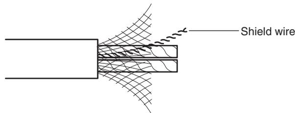
3. Remove the exposed mesh and the aluminum tape from the signal and power lines. Strip the covering from the signal and power lines to the proper length for the crimp terminals. Twist together the wires of each of the signal and power lines.
