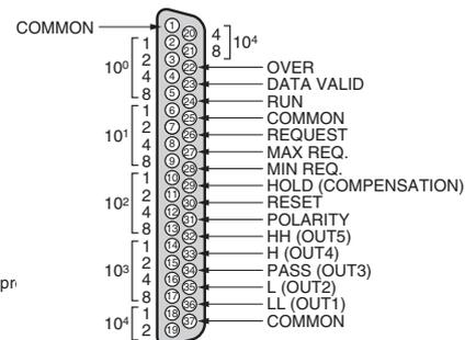
**Note** D-sub connectors are connected to the BCD output cable.
