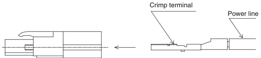
The crimp terminals can be crimped using a crimp tool that conforms to JIS C9711. The following crimp tool is also available: HR31-TC-01 (Hirose Electric)
