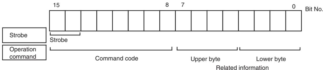
Bit 15 is strobe 2 and bit 14 is strobe 1. A logical OR is taken between the two leftmost bits of the command code and bits 15 and 14, and the result is attached as the strobe to the operation command. The command code for K3HB-DRT operation commands is 0 hex, so when the logical OR is 8 hex, the strobe is ON.
