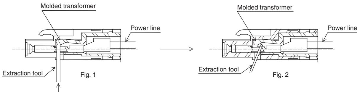
The following extraction tool is available: HR31-SC-TP (Hirose Electric)
