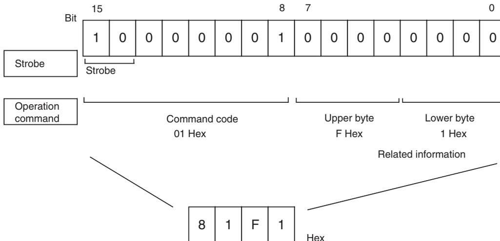
With the CS1W-DRM21 and CJ1W-DRM21 DeviceNet Units, operation commands are made ready for execution by writing to the allocated words (CIO 3202 when the default I/O allocation (fixed allocation area 1) is set.)
