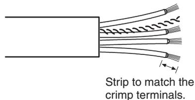
4. Attach crimp terminals to the lines and then cover any exposed areas with vinyl tape or heat-shrink tubing. Making sure that the connector hole numbers are correct, insert each of the signal lines, power supply lines, and the shield wire into the corre-
