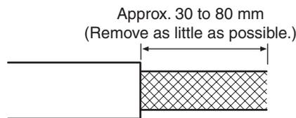
2. Carefully peel back the shield mesh to reveal the signal lines, power lines, and the shield wire. The shield wire is slightly harder to the touch than the mesh.
