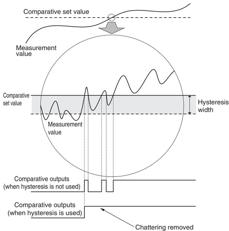
Hysteresis works in the direction of decreasing measurement values for comparative set values HH and H and works in the direction of increasing measurement values for comparative set values LL and L. However, hysteresis works in the direction of decreasing measurement values for all set values if the output pattern is set to a level output.
