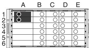
Supply power to terminal numbers A1 and A2. The power supply specifications are outlined below.
