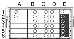
Input the signal to be measured. The following figure shows the inputs that can be measured by each model. Connect the input devices to the terminals shown below according to the input type.
