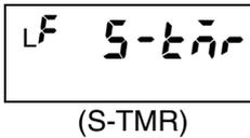
With this function measurement is not performed until a set time has passed after the S-TMR input turns ON. (Timing starts at the rising edge of the S-TMR input and the PV display is “-----” while no measurement has been performed.)
