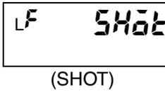
The shot output function turns OFF a comparative output after a set interval after it turns ON. The following diagram shows operation when the shot output is set to 10 ms on the K3HB-S.
