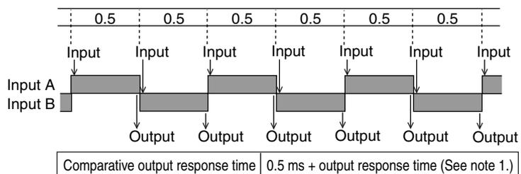
\* The output every 0.5 ms is the comparative output corresponding to the input change for either input A or input B. The input change for both inputs is reflected in the comparative outputs every 1 ms.
