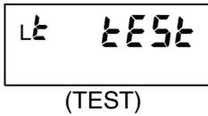
The output test function is used to set test measurement values using the keys to check the comparative outputs against the set comparative set values.
