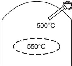
Two points are used to shift the input.
