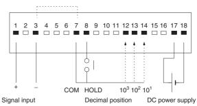
Note: 1. Terminals 3 and 7 of the AC and DC models are not internally insulated. Connect a relay with high contact reliability and insulation (with a minimum load current of 0.3 mA) or a photocoupler with high insulation (with a residual voltage of 1 V max. and a current leakage of 0.1 mA max.) to these terminals for external control.
