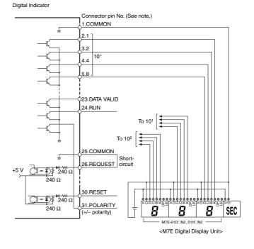
Note: The BCD output connector pin number is the D-sub connector pin number when the BCD Output Cable (sold separately) is connected. This number differs from the pin number for the Digital Indicator narrow pitch connector (manufactured by Honda Tsushin Kogyo Co., Ltd.).
