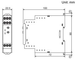
\*Installation Procedure: Mount to the DIN Rail or with front screws
