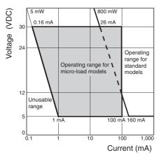
The above diagram is for standard conditions (5°C to 35°C, 40% to 70%). Since the values vary depending on the operating environment conditions, contact your OMRON representative for further details.
