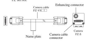
\*The camera cable (FZ-VS,FZ-VSL,FZ-VSB) is polarized, so, make sure that the end bearing a name plate is connected to the Controller.
