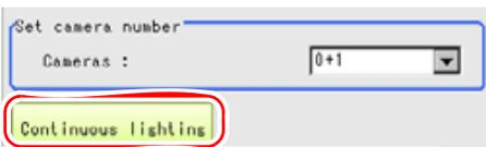
The lighting setting of all connected cameras changes their power of lighting to 50%.
